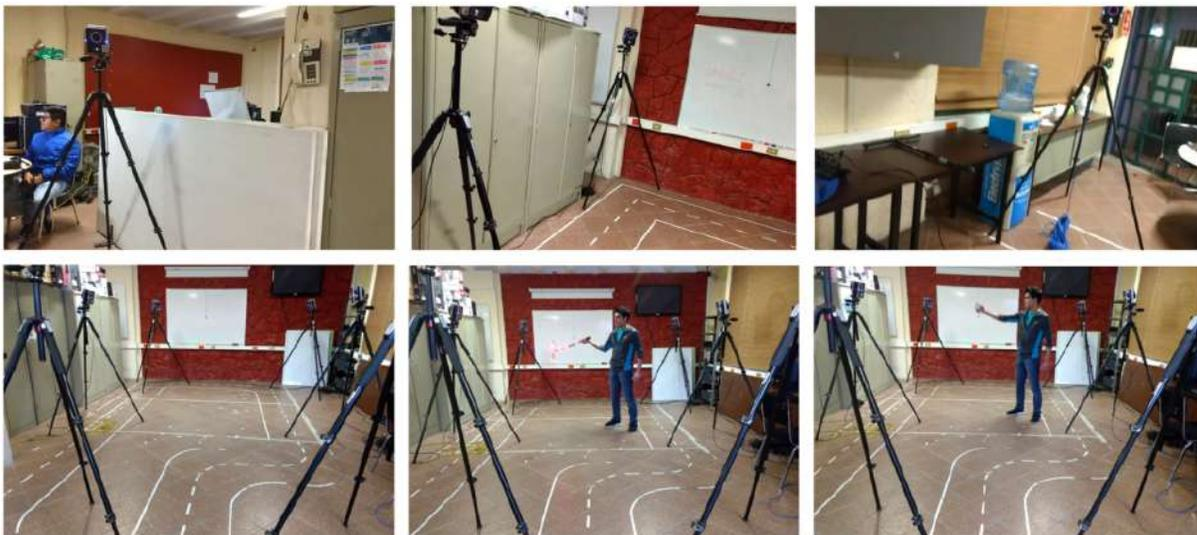
**Figure A.1.** INAOE/DREAM benchmark dataset setup. The data was recorded at full frame rate (60 Hz) and, the ground-truth trajectory was obtained from a high-accuracy motion-capture system with eight high-speed tracking cameras Vicon V8, 8MP, 2000Hz.
