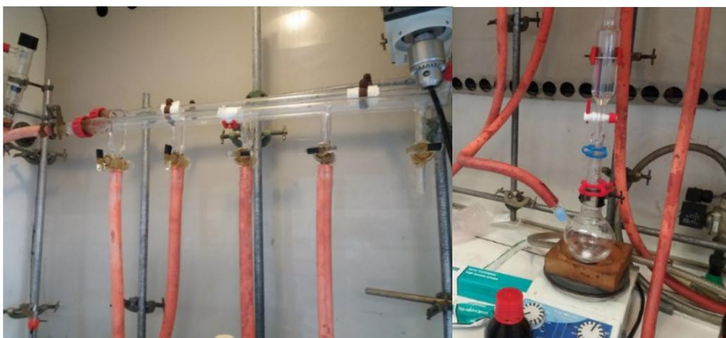
Figure 2.4 Schlenk line used for the synthesis and the drying of the ILs.
