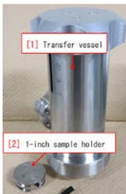
**Figure 2.7 Transfer vessel and sample holder provided by ULVAC-PHI.**
