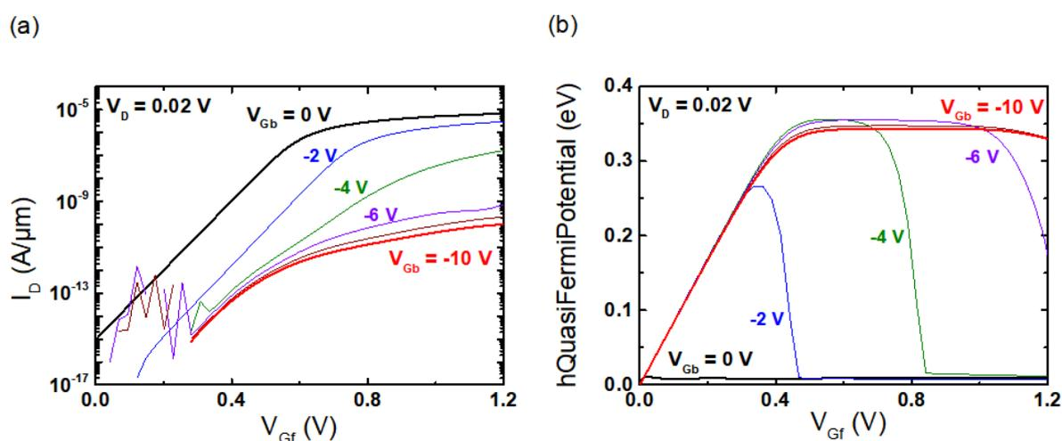
Figure 3.29: TCAD device simulation of (a)  $I_D$  ( $V_{Gf}$ ) versus front-gate bias and (b) Quasi-Fermi potential for holes.  $t_{Si} = 8\text{ nm}$ ,  $t_{BOX} = 25\text{ nm}$ ,  $L_G = 100\text{ nm}$ ,  $V_D = 0.02\text{ V}$ , and  $V_{Gb} = 0\text{ V}$  to  $-10\text{ V}$  (step =  $-2\text{ V}$ ).
