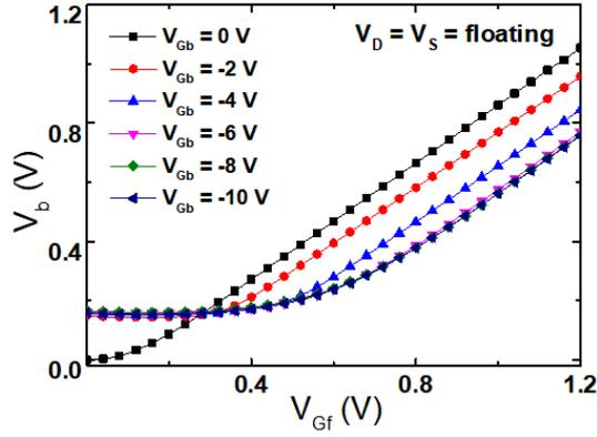
Figure 3.16:  $V_b$  variations for negative back-gate voltages  $V_{Gb}$ , from 0 V to -10 V, with the source and drain contacts floating.  $t_{Si} = 8$  nm,  $W = 10$   $\mu\text{m}$  and  $L_G = 5$   $\mu\text{m}$ .
