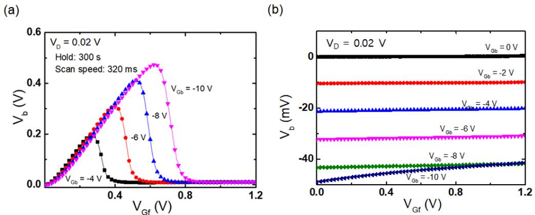
Figure 3.22: Body potential variation in (a) ultrathin body ( $t_{Si} = 8$  nm) and (b) thick body ( $t_{Si} = 25$  nm), with negative back-gate biases.  $t_{BOX} = 25$  nm,  $L_G = 5$   $\mu$ m,  $V_D = 0.02$  V and  $V_{Gb} = 0$  V to  $-10$  V.
