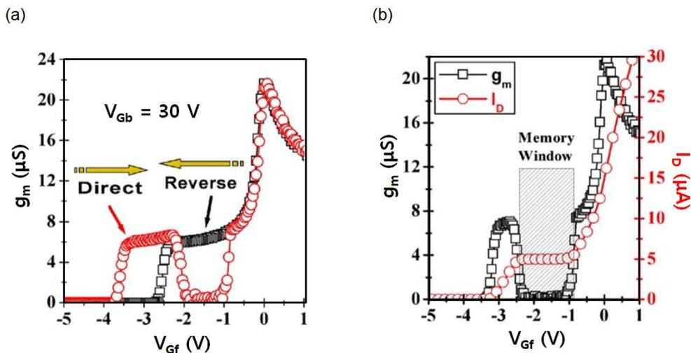
Fig. 2.42: Measured transconductance  $g_m$  versus decreasing (reverse scan; black symbol) and increasing (direct scan; red symbol) of front-gate bias  $V_{Gf}$ : (a)  $g_m(V_{Gf})$ , (b)  $g_m(V_{Gf})$  and drain current.  $V_D = 0.1$  V,  $V_{Gb} = 20$  V.  $t_{Si} = 80$  nm,  $t_{BOX} = 400$  nm, and  $t_{ox} = 10$  nm [42].
