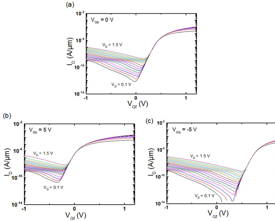
Figure 2.36: Experimental drain current characteristics, from low (0.1 V) to high drain bias (1.5 V), as a function of the front-gate voltage with different back-gate biases. (a)  $V_{Gb} = 0$  V, (b)  $V_{Gb} = 5$  V, and (c)  $V_{Gb} = -5$  V, respectively.  $t_{Si} = 8$  nm,  $t_{BOX} = 25$  nm,  $W = 10$   $\mu\text{m}$ ,  $L = 1$   $\mu\text{m}$ .
