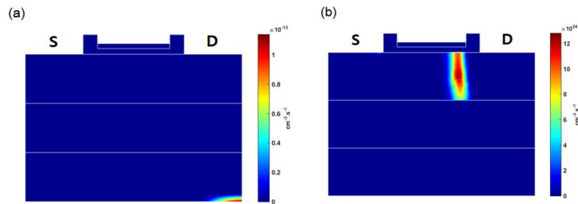
Figure 2.22: Impact ionization multiplication rate extracted from simulation for 'thick' n-MOSFET.  $L = 100 \text{ nm}$ ,  $t_{si} = 25 \text{ nm}$ ,  $t_{BOX} = 25 \text{ nm}$ ,  $V_{Gf} = 1.2 \text{ V}$  and  $V_{Gb} = 0 \text{ V}$ . (a)  $V_D = 0.1 \text{ V}$  and (b)  $V_D = 1.2 \text{ V}$ .
