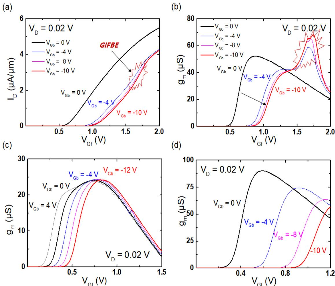
Figure 2.28: Drain current and transconductance  $g_m$  versus gate voltage for variable biasing of the substrate. (a)  $t_{Si} = 25$  nm, drain current, and (b) transconductance showing an ample second peak for negative  $V_{Gb}$ . (c)  $t_{Si} = 12$  nm: the GIFBE is smaller and tends to merge with the regular  $g_m$  peak for  $V_{Gb} < -10$  V. (d)  $t_{Si} = 8$  nm: there is no GIFBE peak.  $t_{BOX} = 25$  nm,  $t_{ox} = 2.9$  nm,  $V_D = 0.02$  V, and  $L = 1$   $\mu m$ .
