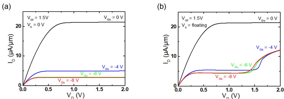
Figure 2.8: Comparison of  $I_D(V_D)$  characteristics of 5-terminal FDSOI MOSFETs measured with the body contact (a)  $V_b = 0\text{ V}$ ; the excess holes are expelled through the grounded body as in bulk silicon device or (b) the body floating condition as for SOI device.  $V_{Gf} = 1.5\text{ V}$ ,  $t_{Si} = 25\text{ nm}$ ,  $t_{BOX} = 25\text{ nm}$ ,  $W = 10\ \mu\text{m}$ , and  $L_G = 5\ \mu\text{m}$ .
