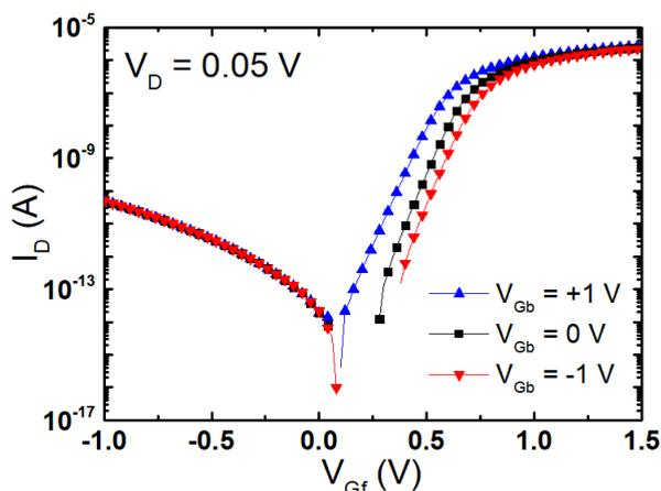
Figure 3.4: Typical  $I_D(V_{Gf})$  characteristics with back-gate biases:  $V_{Gb} = -1$  V, 0 V, and +1 V.  $t_{Si} = t_{BOX} = 25$  nm,  $t_{ox} = 2.9$  nm and  $L_G = 5$   $\mu$ m.  $V_D = 0.05$  V,  $V_{Gb} = +1, 0, -1$  V, respectively.
