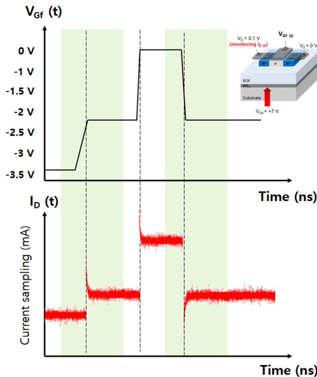
Fig. 2.43: Drain current sampling diagram with pulsed gate biases for measuring the transient current.
