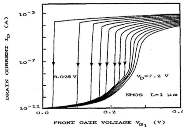
Figure 2.39: Experimental  $I_D(V_G)$  characteristics showing the hysteresis-phenomenon in the n-channel SIMOX MOSFET.  $L = 1 \mu\text{m}$ ,  $V_D = 7.2\text{--}8.025 \text{ V}$  (step = 75 mV). The transients correspond to a negative gate voltage sweep [13].
