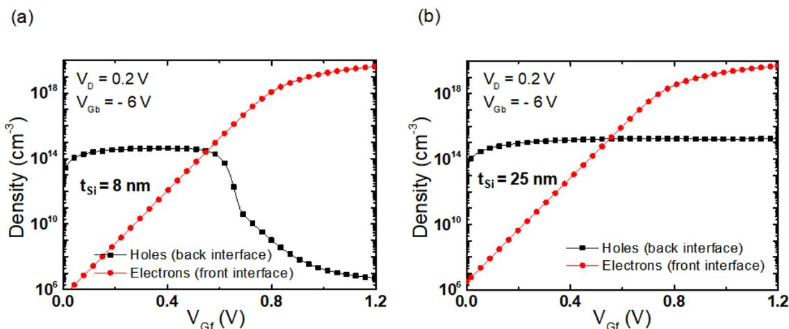
Figure 3.30: Carrier density profile at the back-interface for electron (red symbol) and hole (black symbol), depending on the film thickness with (a)  $t_{Si} = 8$  nm, (b)  $t_{Si} = 25$  nm.  $L_G = 100$  nm,  $V_D = 0.2$  V, and  $V_{Gb} = -6$  V.
