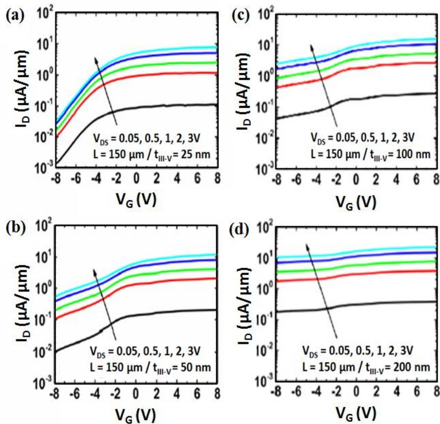
Figure 4.4: Back-gate  $I_D$ - $V_G$  characteristics of lateral  $N+NN+$  InGaAs-OI structures for (a) 25nm, (b) 50nm, (c) 100nm and (d) 200nm thick InGaAs film. Note the transition from full depletion (a) to partial depletion (d).
