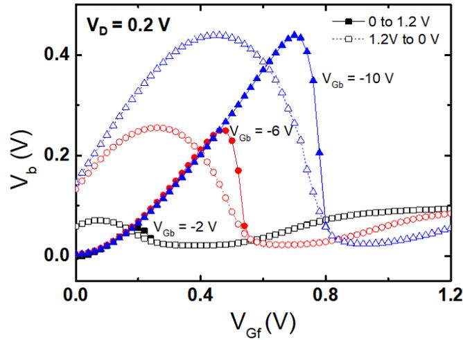
Figure 3.25: The  $V_b$  variation measures in double sweep mode, scanning from 0 V to 1.2 V and return to 0 V right after (scan speed = 20 ms).  $t_{Si} = 8$  nm,  $t_{BOX} = 25$  nm,  $L_G = 5$   $\mu$ m.
