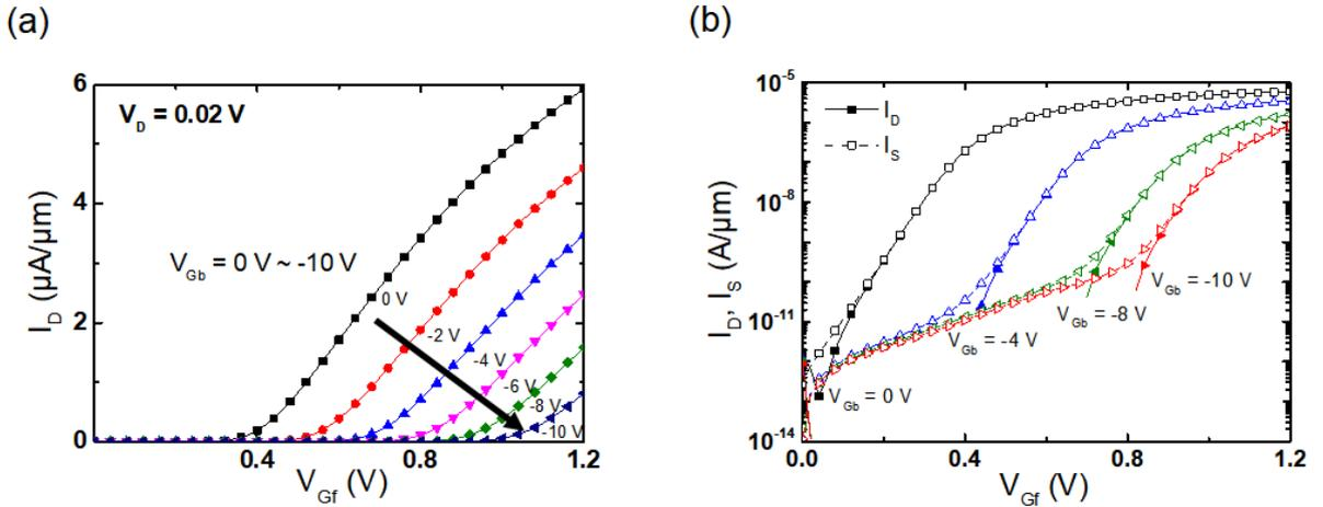
Figure 3.17: Drain current  $I_D$  characteristics with negative back-gate voltage  $V_{Gb}$  (from 0 V to -10 V) in BCN MOSFETs, (a) linear-scale and (b) log-scale with source current  $I_S$ .  $t_{Si} = 8$  nm,  $t_{BOX} = 25$  nm,  $t_{OX} = 1.5$  nm,  $W = 10$   $\mu\text{m}$  and  $L_G = 1$   $\mu\text{m}$ .  $V_D = 0.02$  V.
