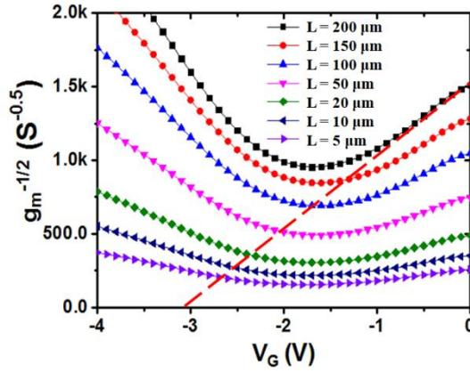
Figure 4.14: Plot of  $1/\sqrt{g_m}$  versus  $V_G$  in bulk conduction (on right region). The dotted line shows the linear fit with Eq.10 in order to determine coefficient  $\theta_1$  and the series resistance.  $W=10 \mu\text{m}$ ,  $t_{III-V} = 200\text{nm}$ ,  $V_D = 0.2 \text{ V}$ .
