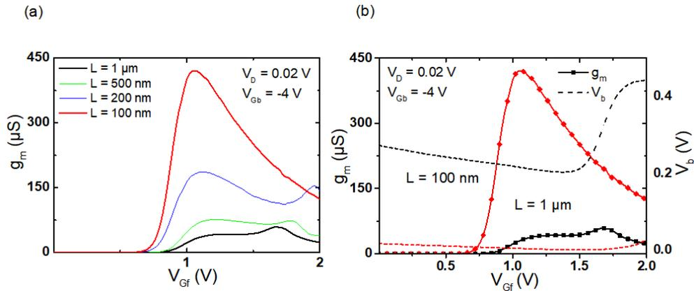
Figure 2.31: (a) Transconductance versus gate voltage measured for different gate lengths. (b) Correlation between transconductance  $g_m$  (plain symbols) and body potential  $V_b$  (dashed lines) in long and short MOSFETs.  $t_{BOX} = 25$  nm,  $t_{ox} = 2.9$  nm,  $V_D = 0.02$  V, and  $L = 1$   $\mu$ m, 100 nm.
