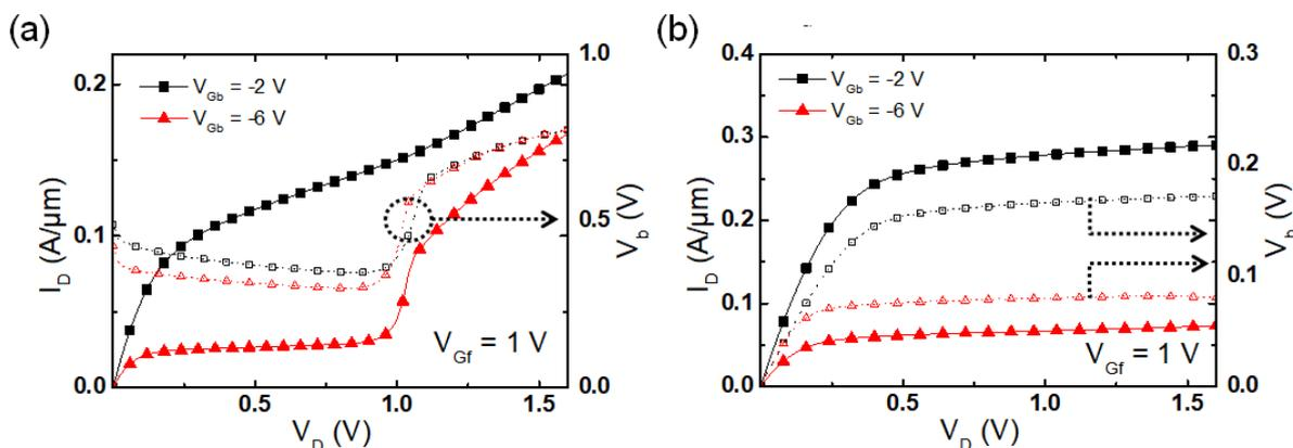
Figure 2.9: Output DC characteristics and corresponding body potential  $V_b$  in FD-SOI MOSFETs with variable Si film thickness. (a)  $t_{Si} = 25\text{ nm}$ , (b)  $t_{Si} = 7\text{ nm}$ ,  $L_G = 100\text{ nm}$  and  $t_{BOX} = 25\text{ nm}$ .
