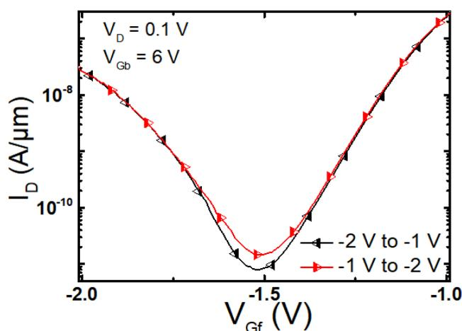
Fig. 2.45: Transfer characteristics in double sweep mode, showing a small hysteresis, which is inadequate for capacitor-less 1T-DRAM application.  $t_{Si} = 25$  nm,  $t_{BOX} = 25$  nm,  $W = 10$   $\mu$ m,  $L = 1$   $\mu$ m,  $V_D = 0.1$  V,  $V_{Gb} = +6$  V.
