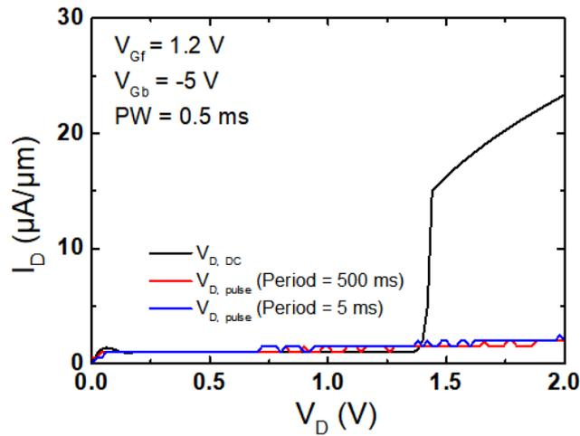
Figure 2.15: Drain current characteristics of 5-terminal MOSFET in DC and pulse mode ( $V_{Gb} = -5$  V) for a long channel device with a short pulse width of drain voltage (0.5 ms) and a long or short period, respectively.  $t_{Si} = 25$  nm,  $t_{Box} = 25$  nm,  $W = 10$   $\mu$ m,  $L = 1$   $\mu$ m.
