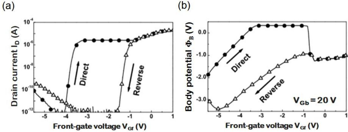
Figure 3.2: (a) The measured transient drain current  $I_D$  hysteresis (or meta-stable effect) resulting from (b) the transient body potential  $\Phi_B$  variations for a SOI n-MOSFET.  $t_{ox} = 4$  nm,  $t_{Si} = 100$  nm,  $t_{BOX} = 400$  nm, and  $L_G = 1$   $\mu$ m [6].
