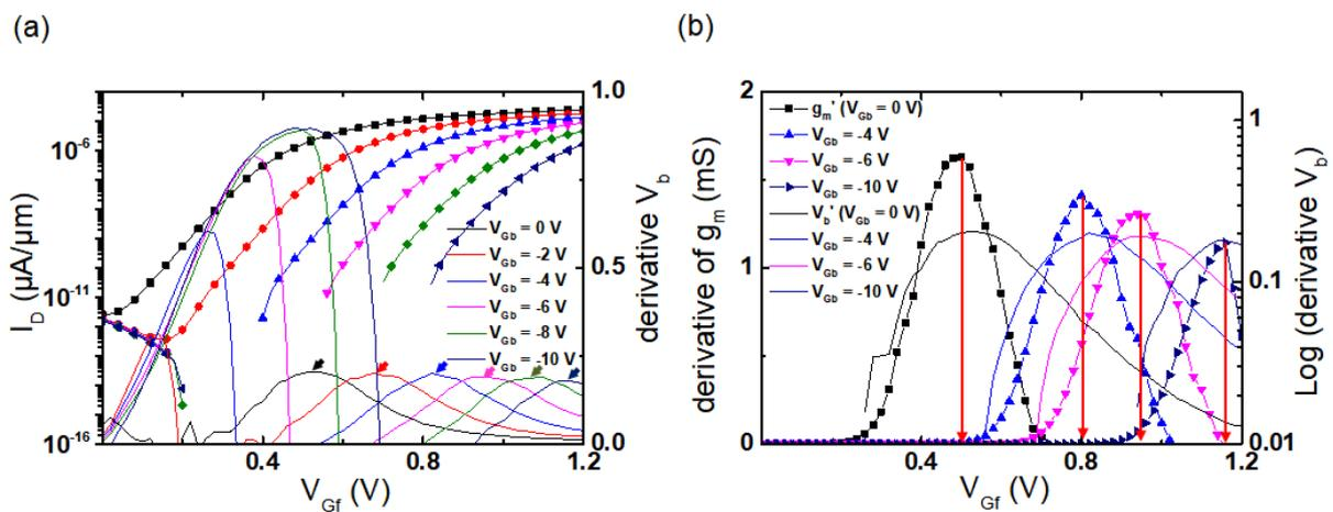
Figure 3.34: Threshold voltage  $V_T$  extraction methods: (a) classical method in  $I_D$  ( $V_{Gf}$ ) (b) first derivative of  $g_m$  method.  $t_{Si} = 8$  nm,  $t_{BOX} = 25$  nm,  $L_G = 5$   $\mu\text{m}$ ,  $V_D = 0.2$  V.
