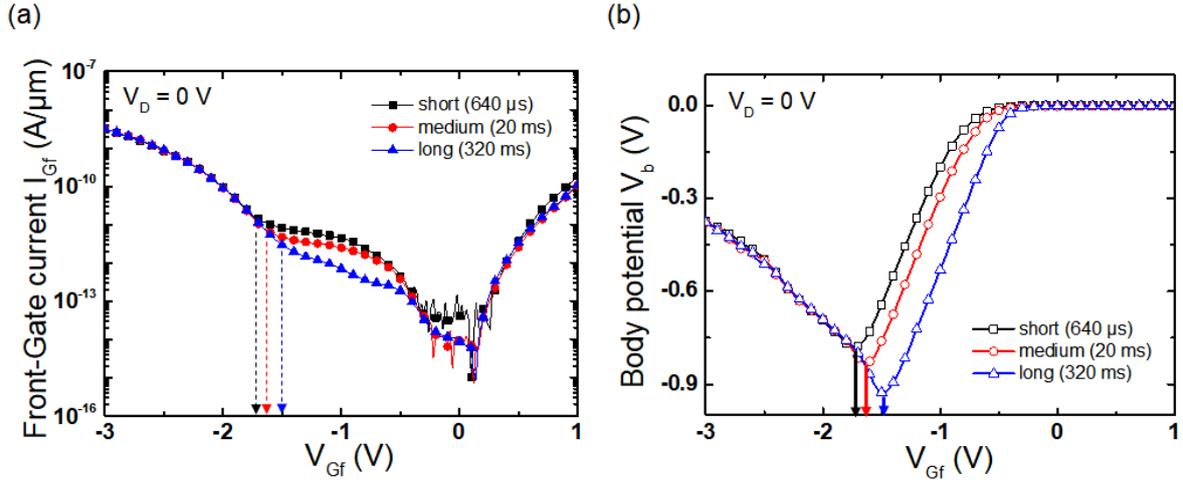
Figure 3.6: Measured (a) front-gate current  $I_{Gf}$  and (b) body potential  $V_b$  versus the front-gate voltage. The front-gate  $V_{Gf}$  sweeps from inversion (or depletion) to accumulation mode, from 1 V to -3 V.  $t_{Si} = t_{BOX} = 25$  nm,  $t_{ox} = 2.9$  nm and  $L_G = 5$   $\mu$ m.  $V_D = V_S = V_{Gb} = 0$  V.
