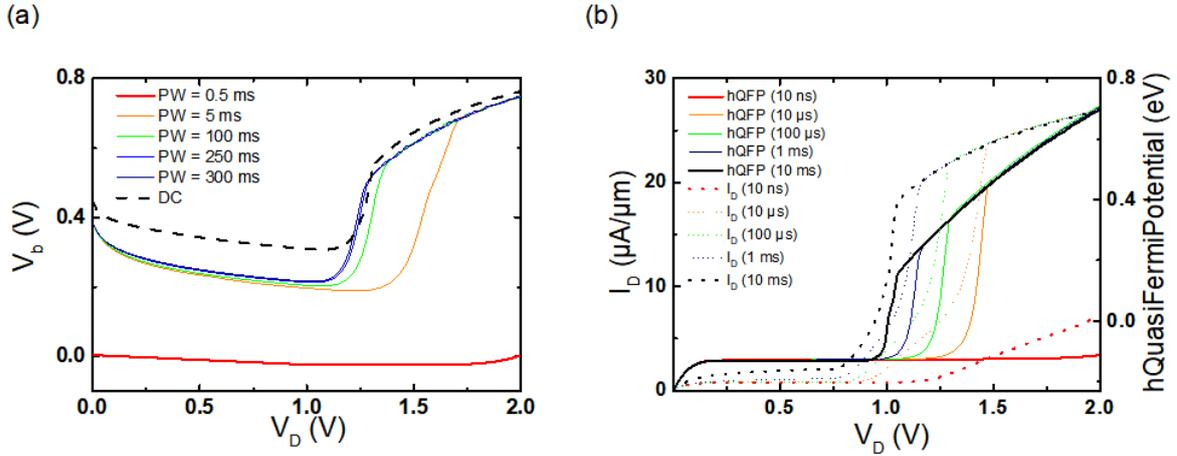
Figure 2.16: (a) Body potentials versus drain bias and pulse width (PW), measured with long-period pulses (500 ms). (b) Simulations showing the quasi-Fermi potential of holes and  $I_D(V_D)$  characteristics.  $V_{Gf} = 1.2$  V,  $V_{Gb} = -5$  V,  $t_{Si} = 25$  nm,  $t_{Box} = 25$  nm.  $W = 10$   $\mu\text{m}$ ,  $L = 1$   $\mu\text{m}$ .
