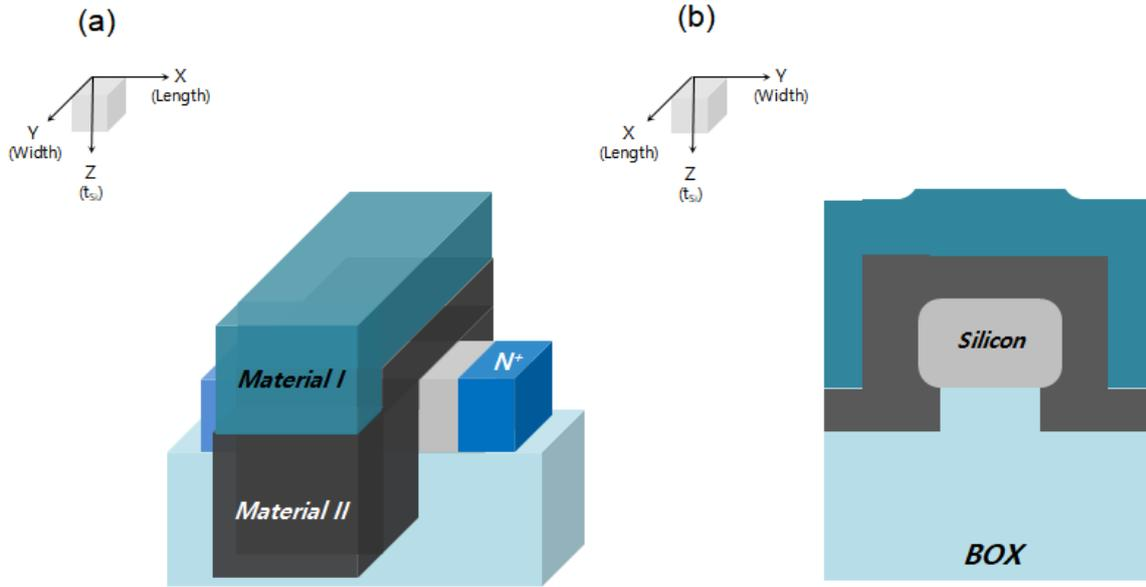
Figure 1.20: (a) Pi ( $\Pi$ ) gate or (b) Omega ( $\Omega$ )-gate shape can reduce the SCEs because the surrounding gate dominates, attenuating the contribution of the electric field from the source and drain into the channel region.
