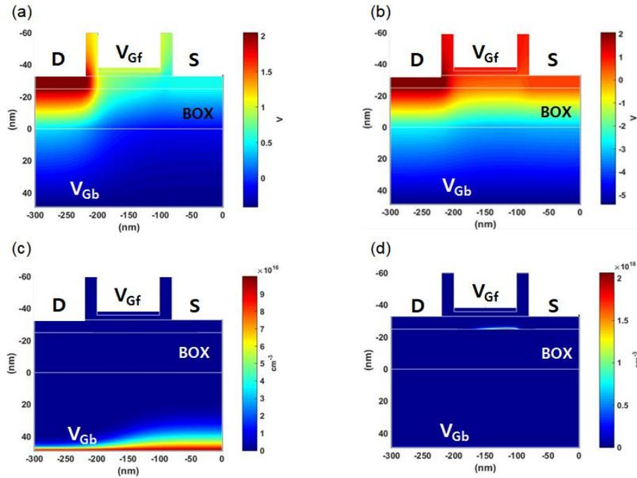
Figure 2.24: Electrostatic potential profiles with (a)  $V_{Gb} = 0$  V, (b)  $V_{Gb} = -5$  V and hole concentrations at the back interface of the silicon body with (c)  $V_{Gb} = 0$  V, (d)  $V_{Gb} = -5$  V, respectively. For  $t_{si} = 8$  nm,  $t_{BOX} = 25$  nm,  $L = 100$  nm, and  $V_{Gf} = 1$  V.
