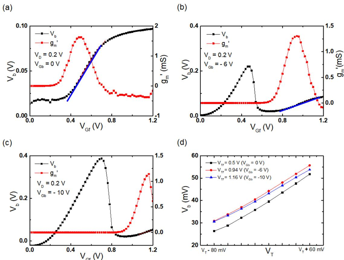
Figure 3.33: Body potential  $V_b$  variation and the first derivative  $g_m$  with back-gate voltages: (a)  $V_{Gb} = 0$  V, (b)  $V_{Gb} = -6$  V, (c)  $V_{Gb} = -10$  V. (d) Correlation between the  $V_b$  and  $g_m'$ .  $t_{Si} = 8$  nm,  $L_G = 5$   $\mu$ m,  $V_D = 0.2$  V.
