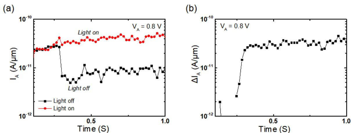
Figure 4.32: A constant voltage of  $V_A = 0.8$  V is used during the measurement (a) Anode current variation with time in the un-gated PIN diode with and without light, (b) current difference between photo-current and dark-current.
