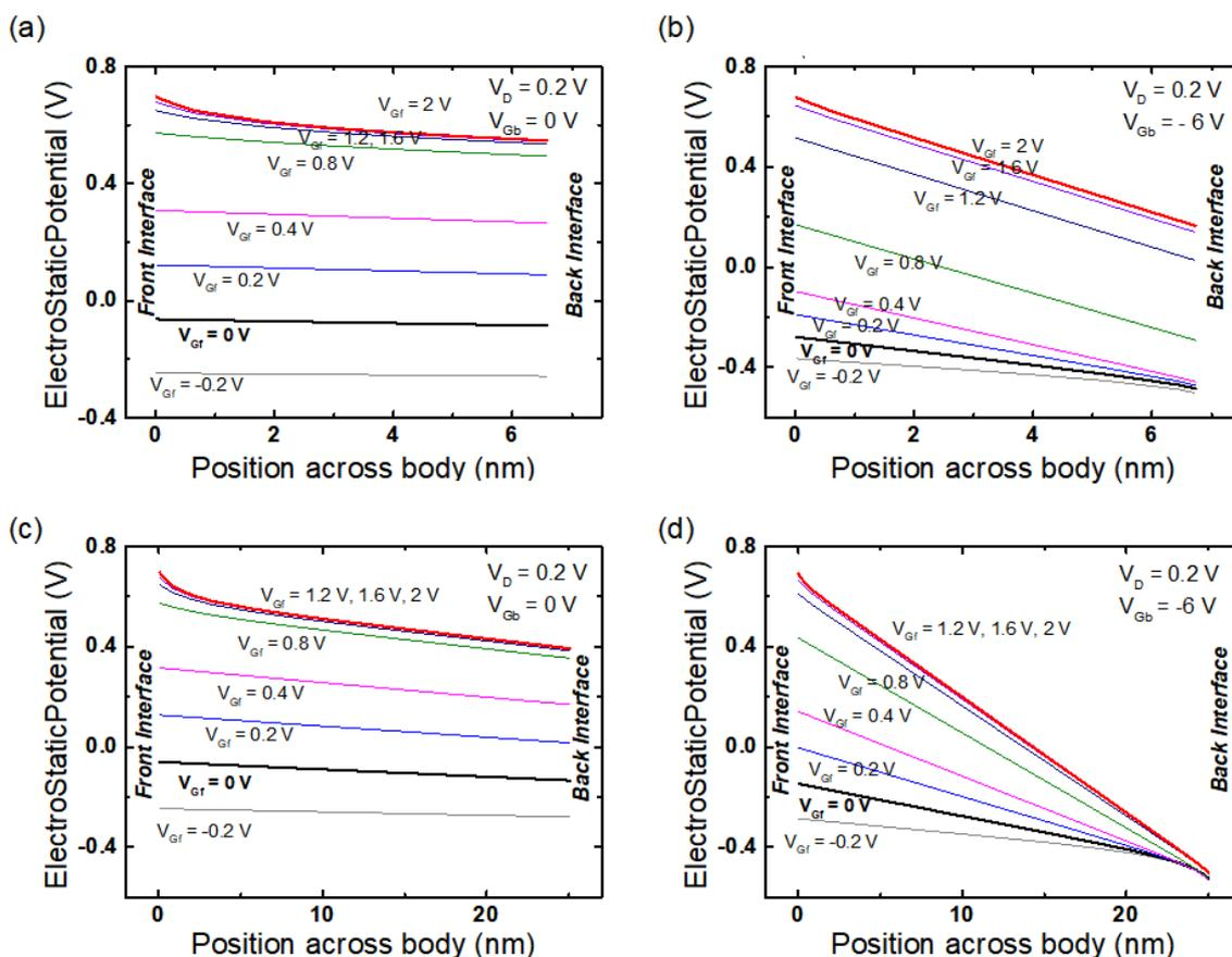
Figure 3.31: Electrostatic potential distributions across the ultrathin body ( $t_{Si} = 8$  nm) present with (a)  $V_{Gb} = 0$  V, (b)  $V_{Gb} = -6$  V. For a relatively thick body ( $t_{Si} = 25$  nm), the electrostatic potential shows with (c)  $V_{Gb} = 0$  V, (d)  $V_{Gb} = -6$  V.  $V_D = 0.2$  V,  $V_{Gf} = -0.2, 0, 0.2, 0.4, 0.8, 1.2, 1.6,$  and  $2$  V, respectively.  $t_{BOX} = 25$  nm,  $L = 1$   $\mu$ m.
