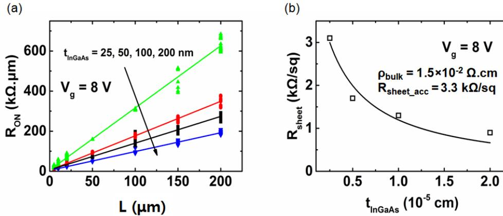
Figure 4.6: (a) On-resistance  $R_{ON}$  versus channel length  $L_g$  extracted at  $V_G=8 \text{ V}$  and  $V_D=0.05 \text{ V}$  for four different InGaAs-OI thickness. (b) Sheet resistance  $R_{sheet}$  deduced from (a) versus InGaAs film thickness fitted by a two parallel conductance model.
