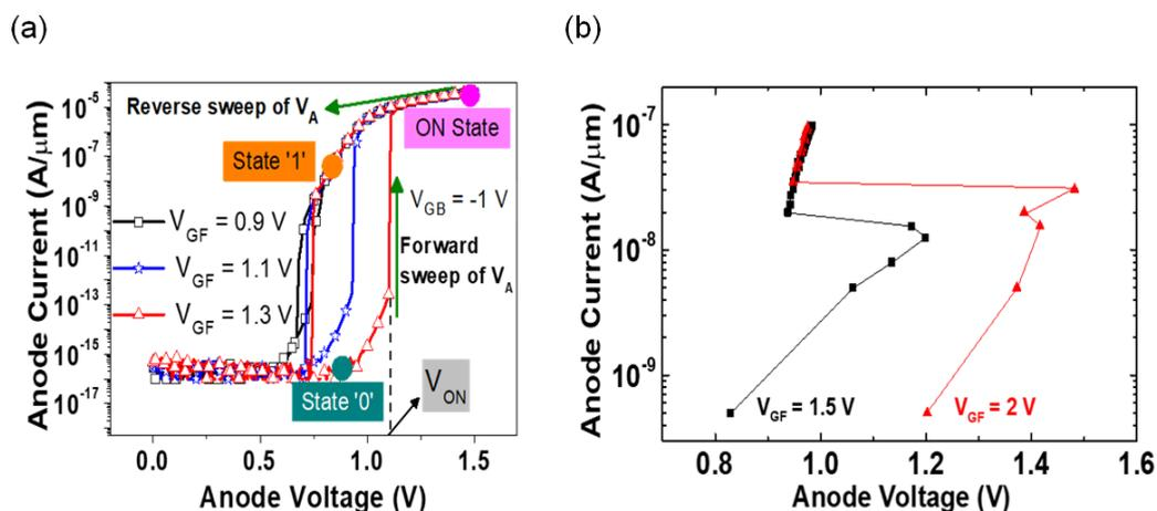
Figure 4.22: Experimental  $I_A$ - $V_A$  curves for different gate voltages in quasi steady-state (DC mode). Measurements were performed by setting the gate biases for several seconds, then (a) slowly scanning the anode voltage to reveal the hysteresis or (b) forcing the anode current to reach the S-shaped curve.  $L_G = L_{int} = 200$  nm.
