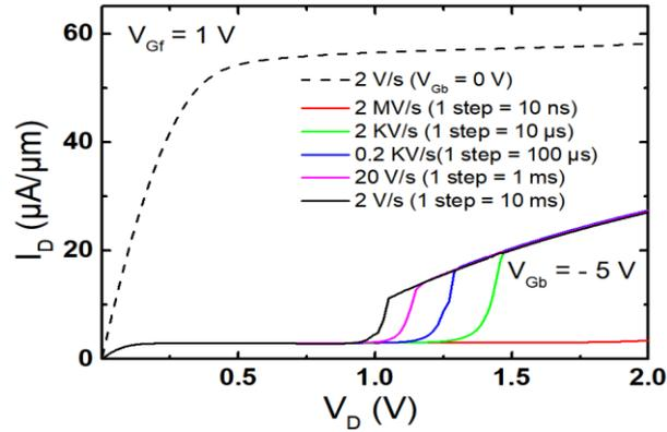
Figure 2.20: Transient simulation of output characteristics for a unit step time increased from 10 ns to 10 ms, respectively.  $V_{Gf} = 1$  V,  $V_{Gb} = -5$  V,  $t_{si} = 25$  nm,  $t_{BOX} = 25$  nm,  $W = 10$   $\mu$ m,  $L = 1$   $\mu$ m.
