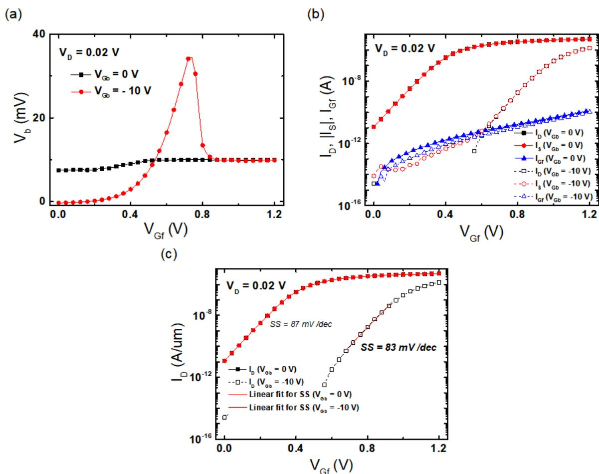
Figure 3.20: A short channel device, showing (a) the  $V_b$  variations with front-gate voltage for variable back-gate bias, (b) drain, source, and gate currents, and (c) subthreshold swing.  $t_{Si} = 8$  nm,  $t_{BOX} = 25$  nm,  $L_G = 50$  nm,  $V_D = 0.02$  V.
