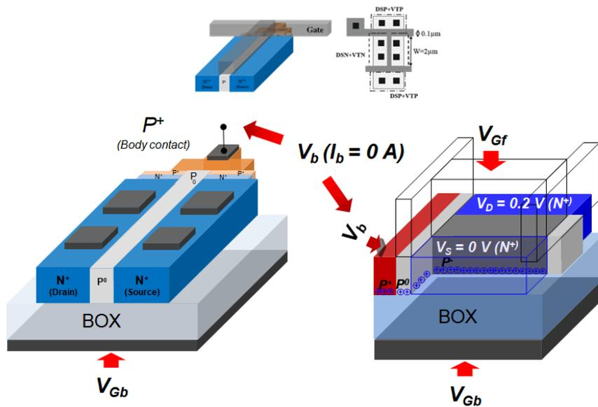
Figure 3.14: Schematic views of the H-gate FDSOI BCN MOSFETs.
