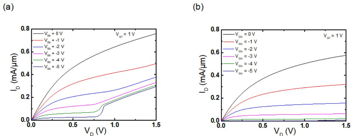
Figure 2.19: Simulated  $I_D(V_D)$  characteristics for different back-gate voltages: (a)  $t_{Si} = 25$  nm, (b)  $t_{Si} = 8$  nm.  $L = 100$  nm,  $t_{BOX} = 25$  nm,  $V_{Gf} = 1$  V,  $V_{Gb} = 0$  to  $-5$  V.
