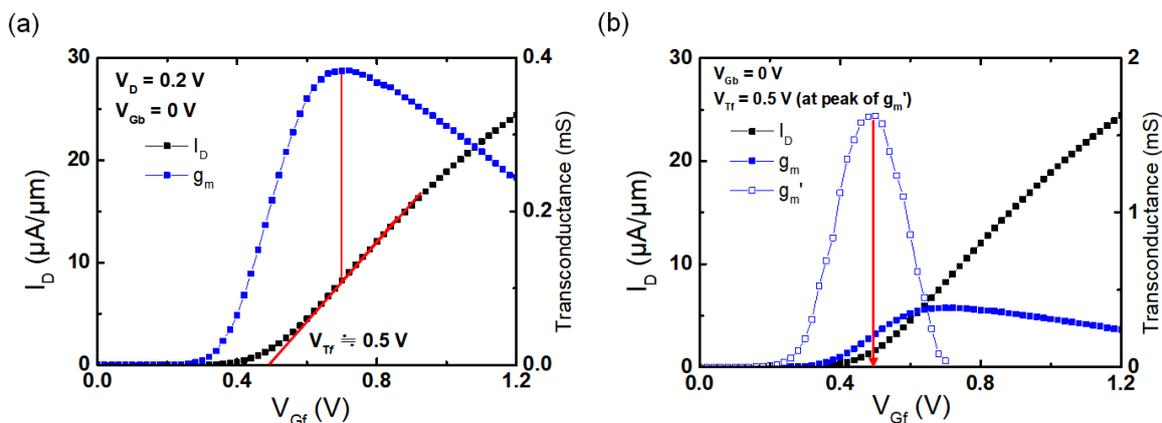
Figure 3.32: Threshold voltage  $V_T$  extraction with two methods: (a) the linearly extrapolation method in  $I_D(V_{Gf})$  and (b) second derivative  $g_m$  method.  $t_{Si} = 8$  nm,  $t_{BOX} = 25$  nm,  $L_G = 5$   $\mu m$ ,  $V_D = 0.2$  V.
