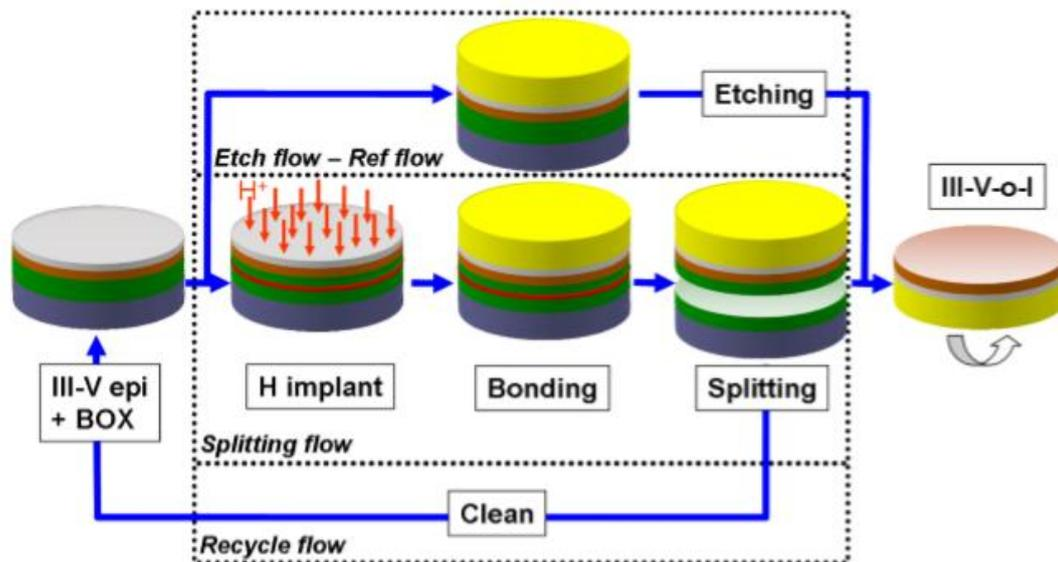
Figure 1.22: Process flow of III-V-on-Insulator wafer fabrication fully compatible with VLSI standards using Direct wafer bonding (DWB), hydrogen implantation, thermal splitting, selective etching, and reusing the InP donor wafer [46].
