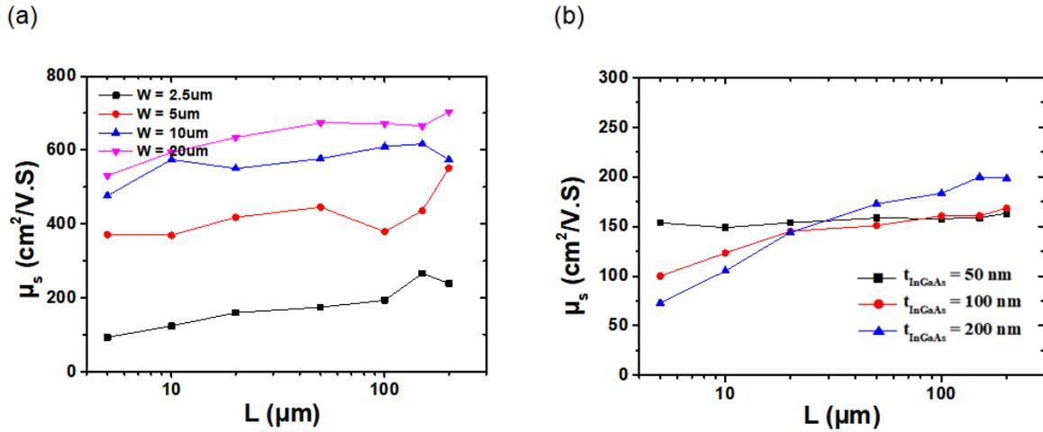
Figure 4.16: Extracted surface mobility versus gate length in (a) 200 nm thick devices with different widths, and (b) narrow devices of 2.5  $\mu\text{m}$  with variable thickness.  $V_D = 0.2 \text{ V}$
