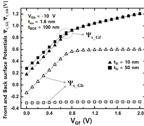
Figure 1.18: Surface potential as a function of the front-gate bias for thick- and thin-silicon body [30]. For the ultrathin device (triangle shape), the back-surface potential follows the front-surface potential because of the supercoupling effect.  $V_{Gb} = -10$  V,  $t_{OX} = 1.6$  nm,  $t_{BOX} = 100$  nm.
