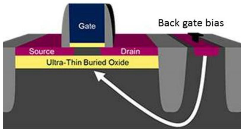
Figure 1.14: UTBB FDSOI MOSFET with back-bias applied via a P+ contact.
