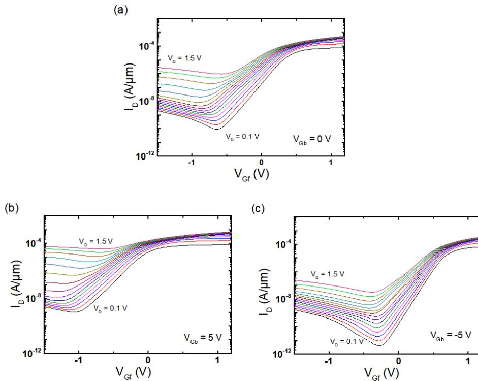
Figure 2.37: Experimental drain current characteristics for a short channel device with different back-gate biases (a)  $V_{Gb} = 0$  V, (b)  $V_{Gb} = 5$  V, and (c)  $V_{Gb} = -5$  V.  $t_{Si} = 8$  nm,  $t_{BOX} = 25$  nm,  $W = 10$   $\mu\text{m}$ ,  $L = 30$  nm.
