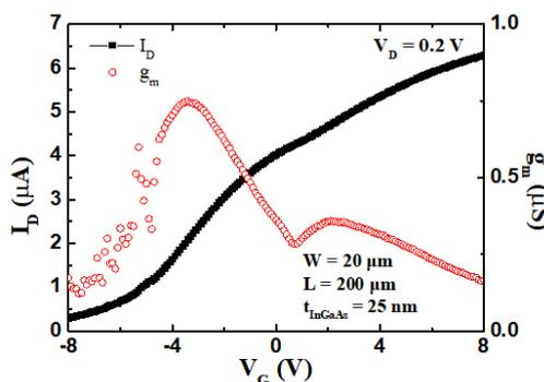
Figure 4.8: Drain current  $I_D$  (black solid symbols) and transconductance  $g_m$  (red empty symbols) as a function of gate bias.  $t_{InGaAs} = 25$  nm,  $W = 20$   $\mu$ m, and  $L = 200$   $\mu$ m.
