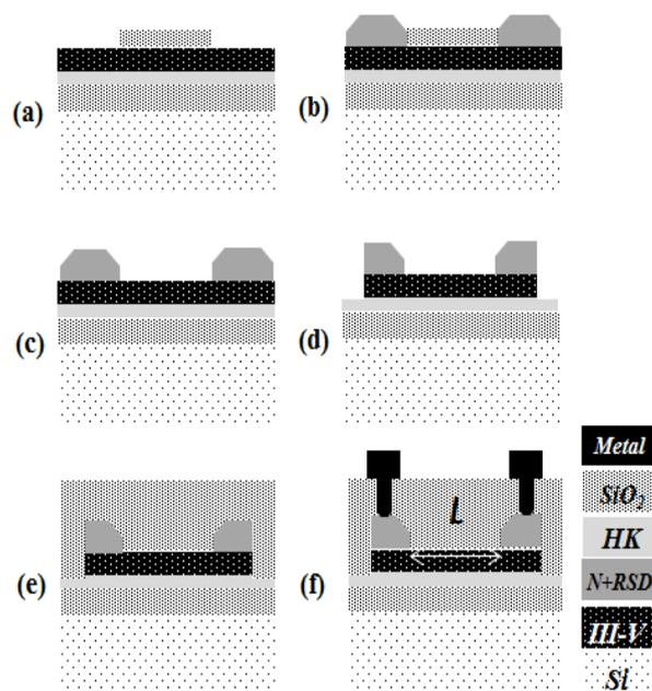
Figure 4.1: Schematic processing sequence of lateral N+NN+ test structure : (a) SiO<sub>2</sub> hard-mask on InGaAs-OI layer with bottom passivation, (b) growth of N<sup>+</sup> InGaAs contacts, (c) hard-mask removal, (d) mesa wet etching, (e) top passivation and interlayer dielectric deposition, (f) contact and metallization.
