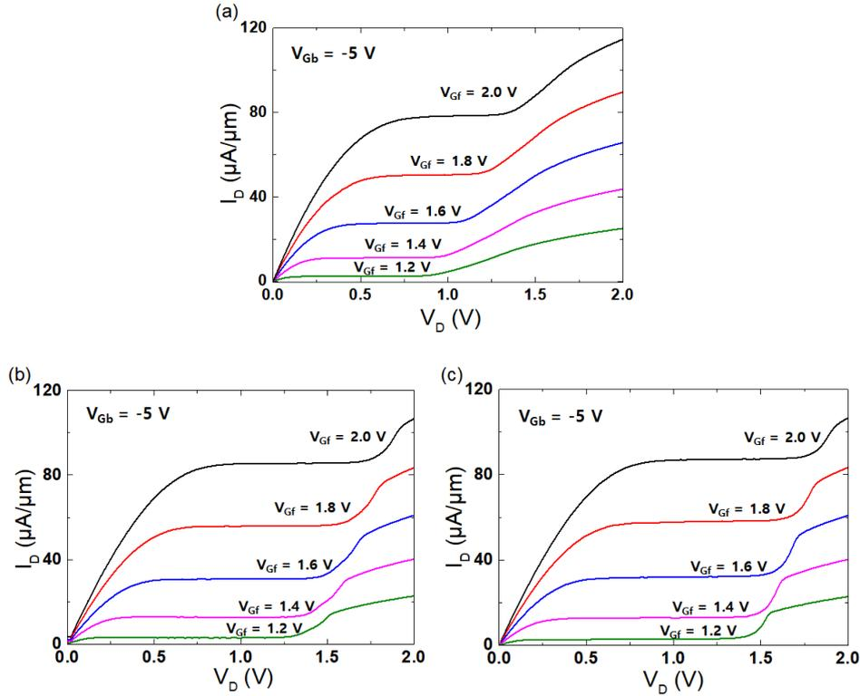
Figure 2.13: Kink effect output characteristics as a function of gate bias  $V_{Gf}$  in the normal n-MOSFET. (a) DC bias condition, and pulsed mode measurement: minimum pulse width of 0.5 ms per (b) a short period of 5 ms and (c) a long period of 500 ms.
