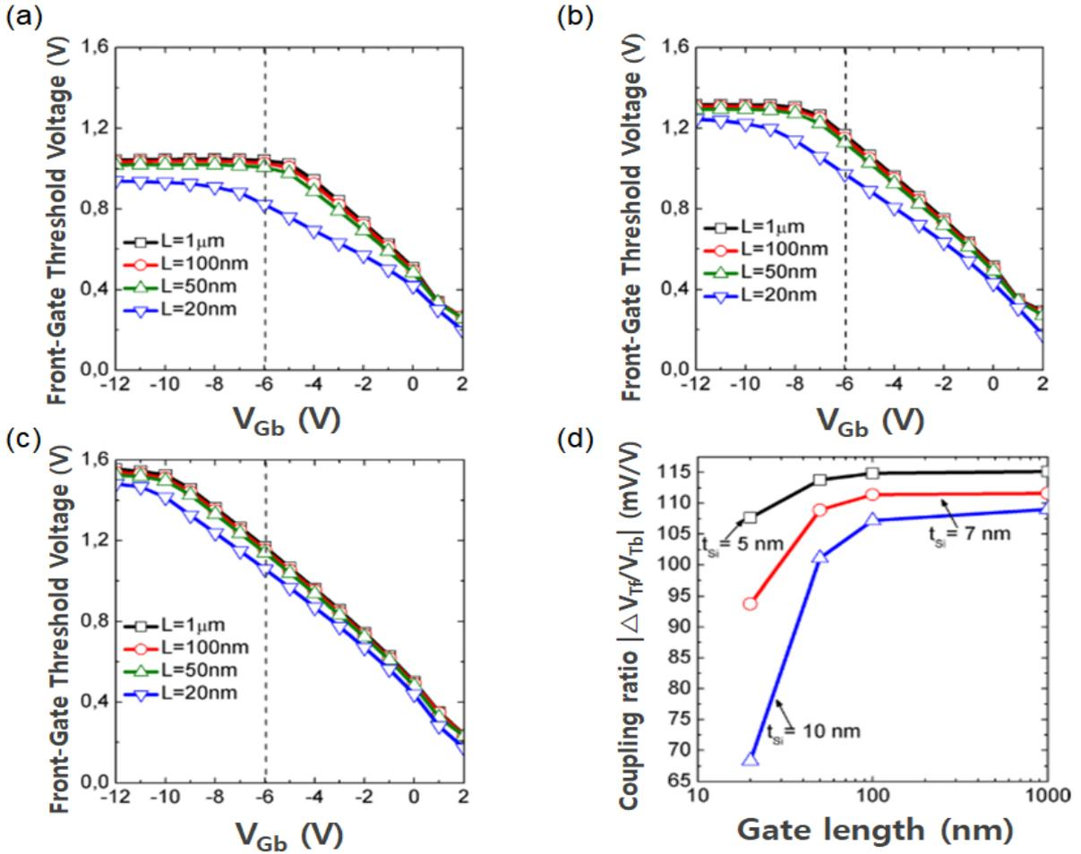
Figure 1.19: Front-gate threshold voltage coupling curves for variable SOI thickness, (a)  $t_{Si} = 10$  nm, (b)  $t_{Si} = 7$  nm, and (c)  $t_{Si} = 5$  nm. (d) The coupling coefficient extracted from the maximum slope in the decreasing threshold voltage region.  $t_{OX} = 1$  nm,  $t_{BOX} = 10$  nm,  $V_D = 0.02$  V, and  $V_{Gf} = 1$  V [33].
