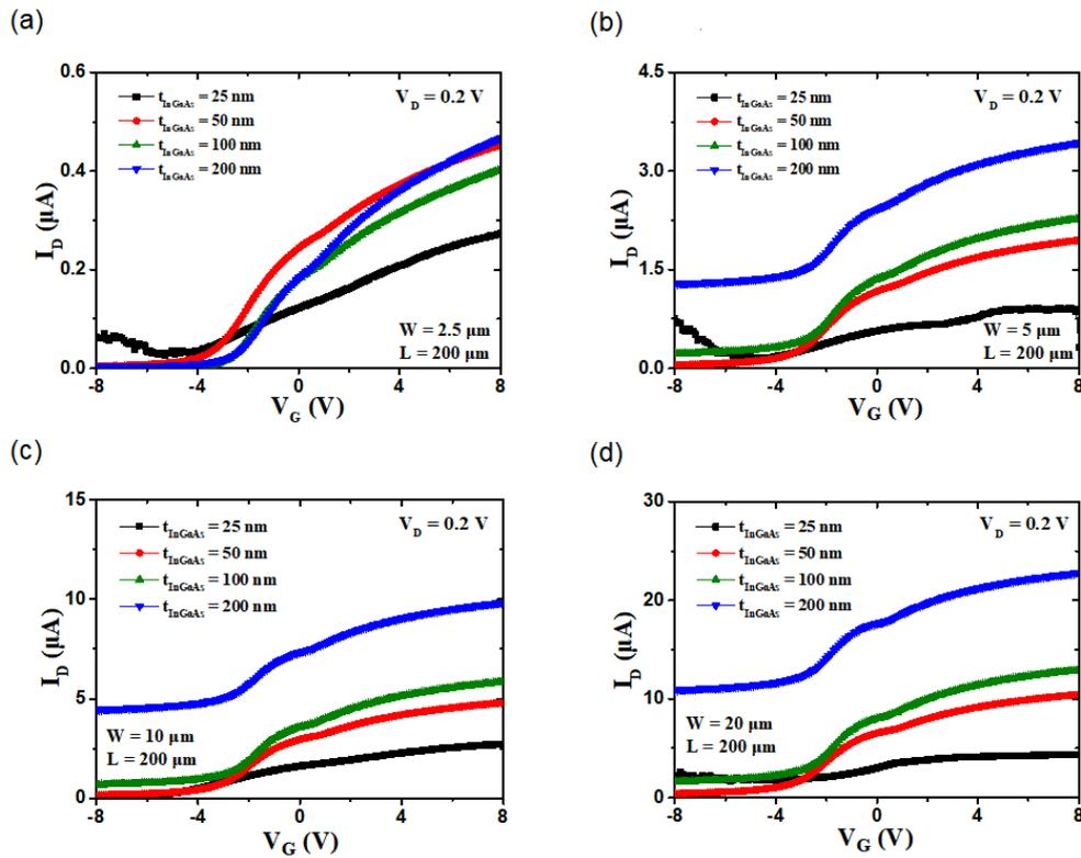
Figure 4.10: Drain current  $I_D$  versus gate voltage for long device widths and different thickness of InGaAs film. (a)  $W = 2.5 \mu\text{m}$ , (b)  $W = 5 \mu\text{m}$ , (c)  $W = 10 \mu\text{m}$ , and (d)  $W = 20 \mu\text{m}$  with a long length ( $L = 200 \mu\text{m}$ ).  $V_D = 0.2 \text{ V}$ .
