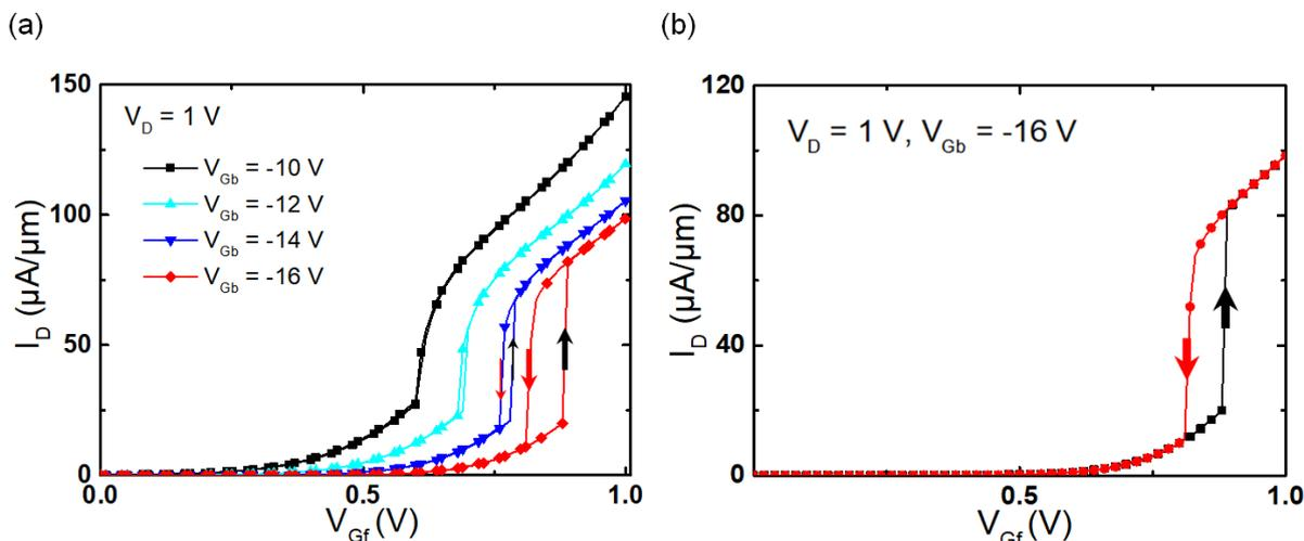
Figure 2.41: (a) Experimental  $I_D(V_{Gf})$  characteristic of a normal FDSOI n-MOSFET measured for various negative back-gate biases. (b) Double swept curve highlighting the hysteresis and sharp switching behavior that occurred for  $V_{Gb} = -16$  V and  $V_D = 1$  V.  $t_{Si} = 25$  nm,  $t_{BOX} = 25$  nm,  $G_{ox} = 2.9$  nm,  $W = 10$   $\mu\text{m}$ ,  $L = 70$  nm.
