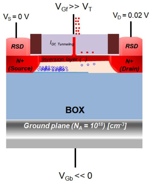
Figure 2.27: Schematic of GIFBE mechanism in FDSOI n-MOSFET, showing excess holes created by the gate tunneling current  $I_{Gf, T}$ , which contributes to excess holes left into the floating body. The excess holes lower the front threshold ( $V_T$ ) and drastically increase drain current instantly.
