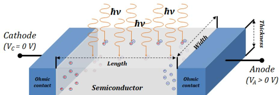
Figure 4.28: Schematic diagram of a photoconductor with applying bias in between anode and cathode [51].
