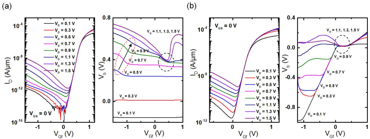
Figure 3.11:  $I_D$  ( $V_{Gf}$ ) characteristics and the  $V_b$  variation, with drain voltage  $V_D$  changed from 0.1 V to 1.5 V, respectively. For (a) a thick,  $t_{Si} = 25$  nm and (b) an ultrathin BCN MOSFET versus the front-gate  $V_{Gf}$  bias,  $t_{Si} = 8$  nm.  $t_{BOX} = 25$  nm,  $t_{ox} = 2.9$  nm and  $L_G = 1$   $\mu\text{m}$ .  $V_{Gb} = 0$  V,  $V_D = 0.1$  to 1.5 V (step = 0.2 V).
