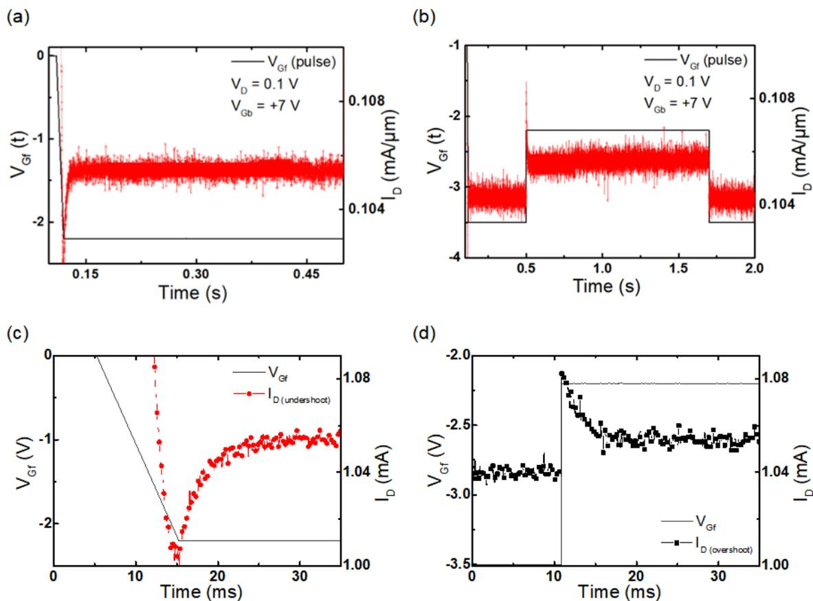
Fig. 2.44: Experimental transient currents measured in (a) undershoot condition with applying the  $V_{Gf}$  pulsed from 0 V to -2.2 V, and (b) overshoot condition:  $V_{Gf}$  pulsed from -3.5 V to -2.2 V. Zoom on the transient variations of drain current in the conditions of (c) undershoot and (d) overshoot.  $t_{Si} = 25$  nm,  $t_{BOX} = 25$  nm,  $W = 10$   $\mu$ m,  $L = 60$  nm,  $V_D = 0.1$  V,  $V_{Gb} = +7$  V.
