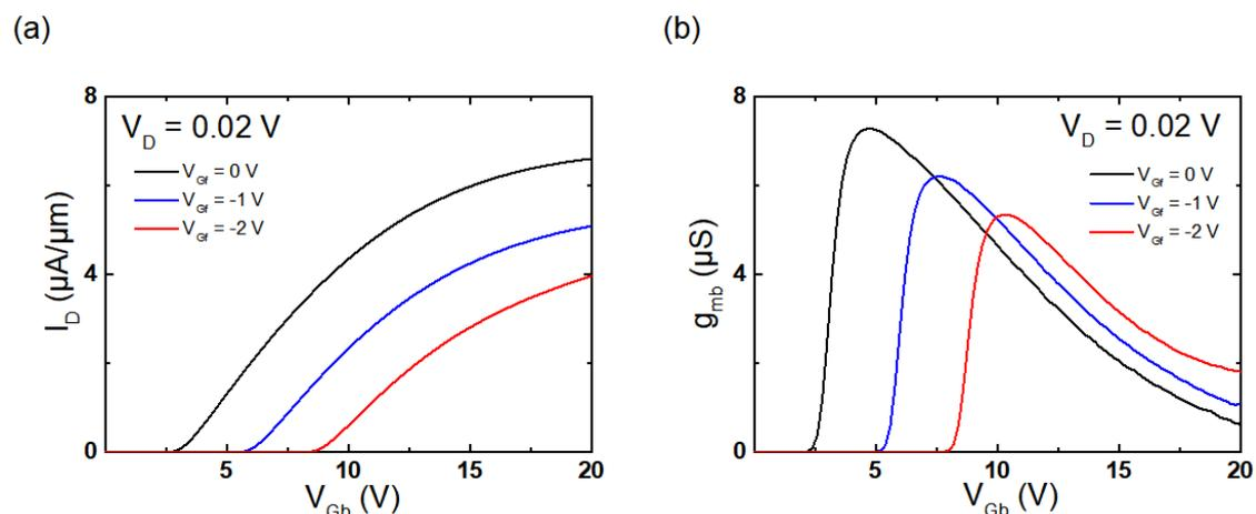
Figure 2.33: GIFBE-free back-channel characteristics. Drain current and transconductance  $g_m$  versus back-gate voltage for variable biasing of the front gate.  $t_{Si} = 25 \text{ nm}$ ,  $t_{BOx} = 25 \text{ nm}$ ,  $V_D = 0.02 \text{ V}$ , and  $L = 1 \mu\text{m}$ .
