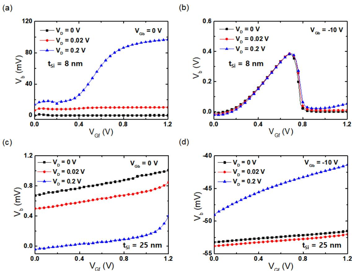
Figure 3.15: Measured body voltage  $V_b$  variations with drain biases from 0 V to 0.2 V versus the front-gate bias. For thin devices ( $t_{Si} = 8$  nm) with (a)  $V_{Gb} = 0$  V, (b)  $V_{Gb} = -10$  V, and thick devices ( $t_{Si} = 25$  nm) with (c)  $V_{Gb} = 0$  V, (d)  $V_{Gb} = -10$  V, respectively.  $W = 10$   $\mu$ m and  $L_G = 5$   $\mu$ m.
