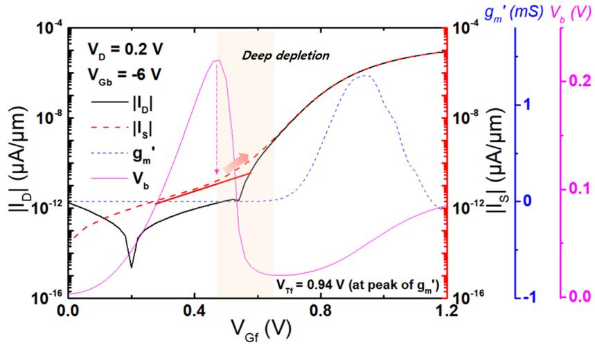
Figure 3.21: Body potential variation reflects the change of source  $I_S$  and drain  $I_D$  currents. Derivative of transconductance  $g_m'$  also shows the threshold voltage  $V_T$ .  $t_{Si} = 8$  nm,  $t_{BOX} = 25$  nm,  $L_G = 5$   $\mu$ m.
