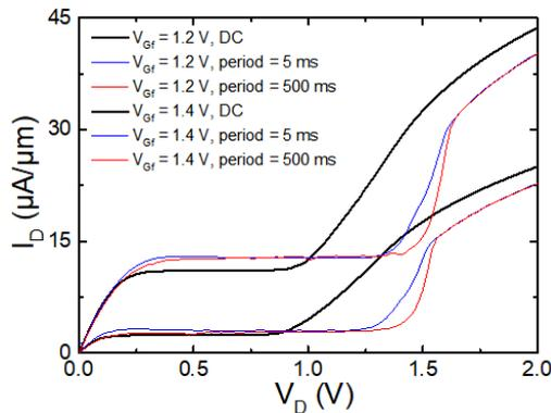
Figure 2.14: Comparison of the kink effect measured in DC and pulsed modes for a normal n-MOSFET device.  $V_{Gb} = -5$  V,  $t_{Si} = 25$  nm,  $t_{BOX} = 25$  nm,  $W = 10$   $\mu\text{m}$ ,  $L_G = 1$   $\mu\text{m}$ , and  $PW = 0.5$  ms.
