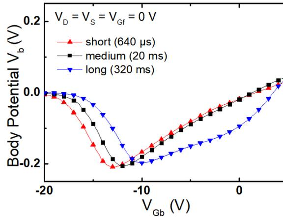
Figure 3.7: Measured  $V_b$  during sweeping back-gate  $V_{Gb}$  from inversion to accumulation.  $t_{Si} = t_{BOX} = 25$  nm,  $t_{ox} = 2.9$  nm and  $L_G = 5$   $\mu$ m.  $V_D = V_S = V_{Gf} = 0$  V.
