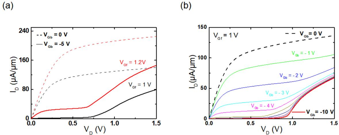
Figure 2.4: Normalized output  $I_D(V_D)$  characteristics with back-gate voltage (a)  $V_{Gf} = 1\text{ V}$ ,  $1.2\text{ V}$  and  $V_{Gb} = 0\text{ V}$  or  $-5\text{ V}$ . (b)  $V_{Gf} = 1\text{ V}$  and  $V_{Gb} = 0$  to  $-10\text{ V}$ .  $W = 10\ \mu\text{m}$ ,  $L = 150\text{ nm}$ ,  $t_{Si} = 25\text{ nm}$ ,  $t_{ox} = 2.9\text{ nm}$ ,  $t_{BOX} = 25\text{ nm}$ .
