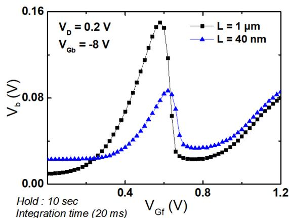
Figure 3.19: Long- and short-channel BCN MOSFETs, showing the  $V_b$  variation versus front-gate voltage with negative back-gate,  $V_{Gb} = -8$  V.  $t_{Si} = 8$  nm,  $t_{BOX} = 25$  nm,  $t_{OX} = 1.5$  nm,  $V_D = 0.2$  V.
