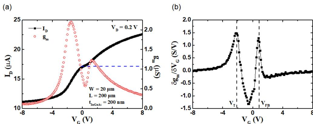
Figure 4.7: (a) Drain current  $I_D$  (plain symbols) and transconductance  $g_m$  (empty symbols) versus gate bias. The dashed line represents the 'bulk' current  $I_{vol}$ . (b) Corresponding  $g_m$  derivative versus  $V_G$ , which features a double threshold voltage behavior.  $t_{InGaAs} = 200$  nm,  $W = 20$   $\mu$ m, and  $L = 200$   $\mu$ m.
