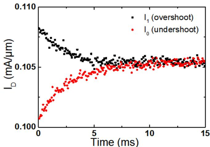
Fig. 2.46: Normalized transient currents,  $I_1$  and  $I_0$ , overlapped on the same axis in order to determine the retention time.  $t_{Si} = 25$  nm,  $t_{BOX} = 25$  nm,  $W = 10$   $\mu$ m,  $L = 1$   $\mu$ m,  $V_D = 0.1$  V,  $V_{Gb} = +6$  V.
