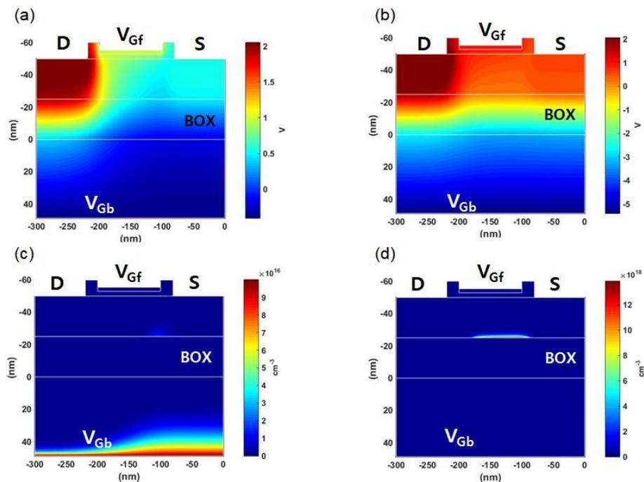
Figure 2.23: Electrostatic potential profiles with (a)  $V_{Gb} = 0 \text{ V}$ , (b)  $V_{Gb} = -5 \text{ V}$  and hole concentration at the back interface of the silicon body with (c)  $V_{Gb} = 0 \text{ V}$ , (d)  $V_{Gb} = -5 \text{ V}$ , respectively. For  $t_{si} = 25 \text{ nm}$ ,  $t_{BOX} = 25 \text{ nm}$ ,  $L = 100 \text{ nm}$ , and  $V_{Gf} = 1 \text{ V}$ .
