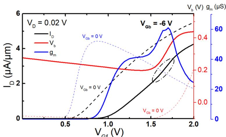
Figure 3.9: Measured  $I_D$ ,  $V_b$ , and  $g_m$  with low drain voltage ( $V_D = 0.02$  V). Correlation with between transconductance  $g_m$  (blue curve) and body potential  $V_b$  variation (red curve) in long channel MOSFET during sweeping back-gate  $V_{Gb}$ .  $t_{Si} = t_{BOX} = 25$  nm,  $t_{ox} = 2.9$  nm and  $L_G = 1$   $\mu$ m.  $V_D = 0.02$  V,  $V_{Gb} = 0$  V and  $-6$  V.
