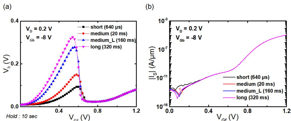
Figure 3.24: (a)  $V_b$  variation with bias scan speed (from 640  $\mu$ s to 320 ms) and (b) source currents  $I_S$  are demonstrated in order to identify the reason why the  $V_b$  is low value in the fast scan mode, short integration time (640  $\mu$ s).  $t_{Si} = 8$  nm,  $t_{BOX} = 25$  nm,  $L_G = 5$   $\mu$ m.
