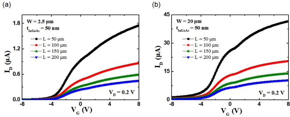
Figure 4.9: Drain current  $I_D$  versus gate bias for different channel lengths, from  $50 \mu\text{m}$  to  $200 \mu\text{m}$ , showing the width dependency. (a)  $W = 2.5 \mu\text{m}$ , (b)  $W = 20 \mu\text{m}$ .  $t_{\text{InGaAs}} = 25 \text{ nm}$  and  $V_D = 0.2 \text{ V}$ .
