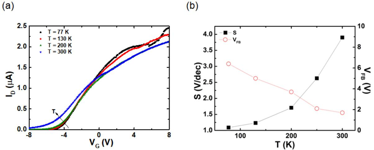
Figure 4.17: (a) Drain current as a function of gate bias measured at variable temperature. (b) Associated variations of sub-threshold swing  $S$  and flat-band voltage  $V_{FB}$  with low temperature  $T$ . For  $t_{InGaAs} = 25 \text{ nm}$ ,  $W = 5 \text{ }\mu\text{m}$ ,  $L = 100 \text{ }\mu\text{m}$ , and  $V_D = 0.2 \text{ V}$ .
