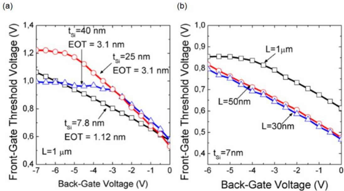
Figure 1.17: Experimental variation of front-gate threshold voltage versus back-gate bias, showing impact of (a) silicon thicknesses and (b) gate lengths.  $L = 1 \mu\text{m}$ ,  $t_{BOX} = 25 \text{ nm}$ ,  $N_A = 10^{15} \text{ cm}^{-3}$ ,  $V_D = 0.02 \text{ V}$  [33].
