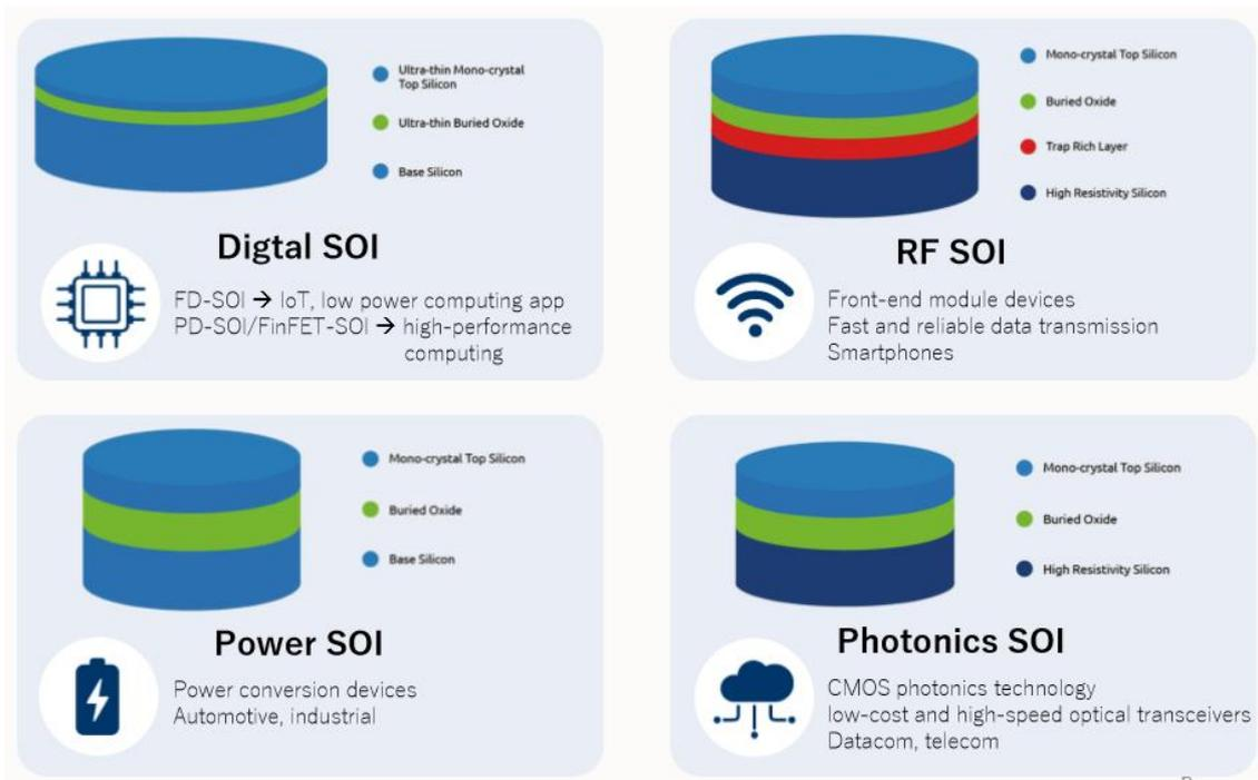
Figure 1.8: Different types of engineered SOI wafer for specified commercialized products: generic CMOS devices, RF circuit and components, power chips, and photonics applications.
