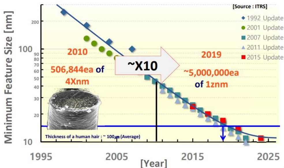
Figure 1.2: Evolution of the DRAM scaling trend with minimum feature size.
