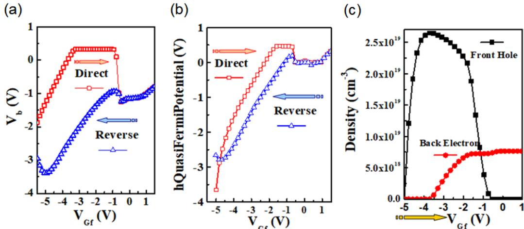
Figure 3.26: (a) Measured body potential and (b) simulated hole quasi-Fermi level  $QFL$  versus decreasing (reverse scan) and increasing (direct scan) front-gate bias  $V_{Gf}$  (c) Simulated hole and electron densities versus increasing (direct scan) front-gate bias  $V_{Gf}$ .  $V_{Gb}$  and  $V_D$  are 30 V and 0.1 V respectively.  $t_{BOX}$ ,  $t_{ox}$  and  $t_{Si}$  are 400 nm, 10 nm and 80 nm. The channel length and width are 300  $\mu$ m [6].
