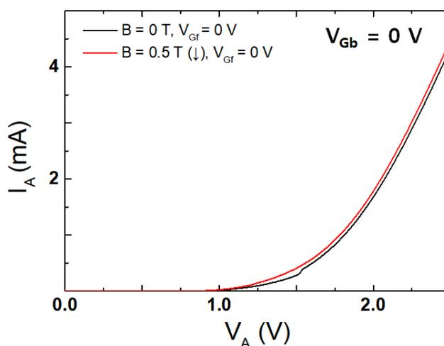
Figure 4.24: Current-voltage characteristics of a p-i-n diode under magnetic field (red line) and without magnetic field (black line).  $L_G = 2 \mu\text{m}$ ,  $L_i = 0.5 \mu\text{m}$ ,  $B = 0$  or  $0.5$  T, and  $V_{Gf} = V_{Gb} = 0$  V.
