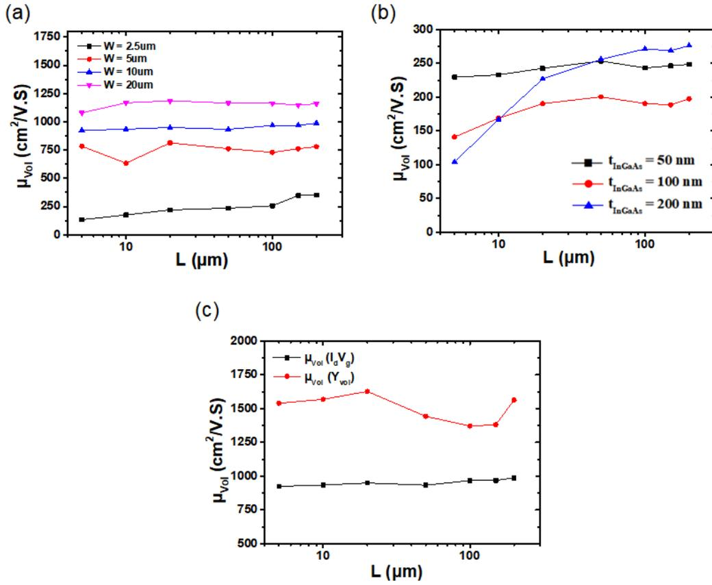
Figure 4.13: Extracted bulk mobility versus channel lengths in (a) 200 nm thick films with variable width and (b) narrow devices of 2.5  $\mu\text{m}$  with different thickness. (c) Comparison of bulk mobility values extracted from  $I_D(V_G)$  curves with Eq.(2) or by using  $Y_{\text{Vol}}$ -function method (Eq.(8)). For  $W = 10 \mu\text{m}$ ,  $t_{\text{InGaAs}} = 200 \text{ nm}$ ,  $V_D = 0.2 \text{ V}$ .
