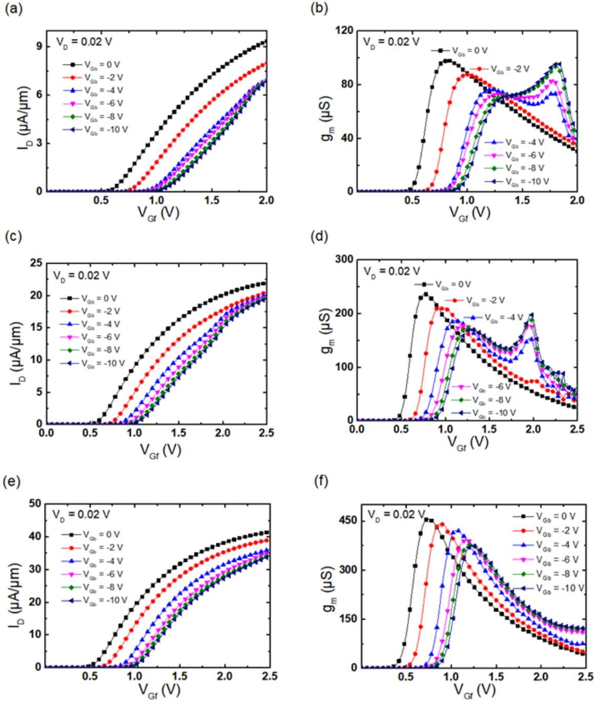
Figure 2.29: Experimental data of drain current  $I_D$  and transconductance  $g_m$  versus gate voltage for variable biasing of the substrate. Independence on channel length, showing (a) - (b)  $L = 500$  nm, (c) - (d)  $L = 200$  nm, (e) - (f)  $L = 100$  nm.  $t_{Si} = t_{BOX} = 25$  nm,  $t_{ox} = 2.9$  nm,  $V_D = 0.02$  V.
