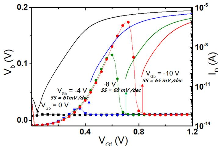
Figure 3.18: Body potential  $V_b$  variations and drain currents  $I_D$ , depending on the different back-gate biases. Subthreshold swing (SS) is also indicated.  $t_{Si} = 8$  nm,  $t_{BOX} = 25$  nm,  $L_G = 5$   $\mu$ m,  $V_D = 0.02$  V.
