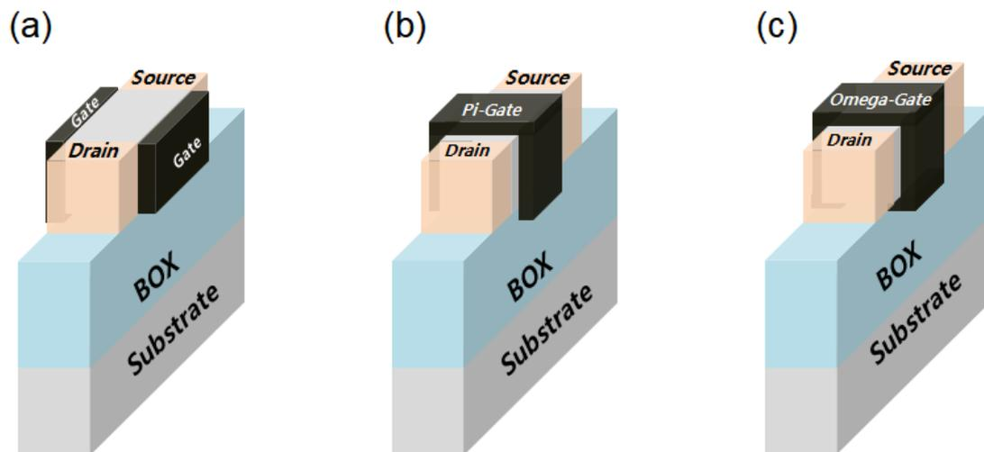
Figure 1.13: Different types of the multi-gate SOI MOSFET distinguished by the gate configuration: (a) double gate, (b) Pi( $\Pi$ ) gate (likewise the tri-gate Fin-FET), and (c) Omega( $\Omega$ )-gate.
