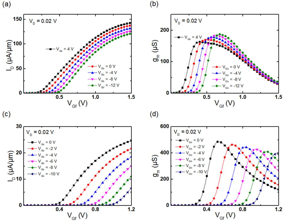
Figure 2.30: Experiment data of drain current and transconductance  $g_m$  versus gate voltage in short channel devices, showing (a) - (b)  $t_{Si} = 12$  nm, (c) - (d)  $t_{Si} = 8$  nm.  $L = 100$  nm,  $t_{BOX} = 25$  nm,  $t_{ox} = 1.5$  nm.
