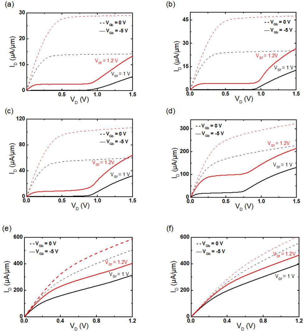
Figure 2.5: Impact of back-gate bias  $V_{Gb}$  from 0 V to -10 V (step -1 V) on  $I_D(V_D)$  characteristics for various channel lengths: (a) 1  $\mu\text{m}$ , (b) 500 nm, (c) 250 nm, (d) 100 nm, (e) 50 nm, and (f) 40 nm;  $W = 10 \mu\text{m}$ ,  $t_{Si} = 25 \text{ nm}$ ,  $t_{ox} = 2.9 \text{ nm}$ , and  $t_{BOX} = 25 \text{ nm}$ .
