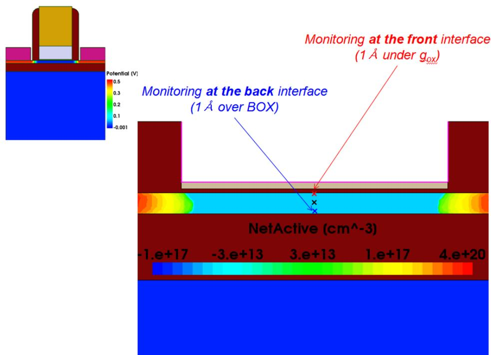
Figure 3.27: Cross-section view of a test structure made by sprocess.  $t_{Si} = 8$  nm,  $t_{BOX} = 25$  nm,  $L_G = 100$  nm.
