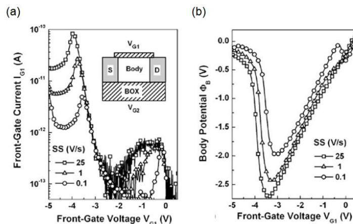
Figure 3.1: Measured dynamic (a) gate current  $I_{Gf}$  [6] and (b) corresponding body potential  $\Phi_B$  versus a decreasing front-gate voltage  $V_{Gf}$  scanned from depletion to accumulation in a PD SOI n-MOSFET. Scan speed ( $Ss$ ) is varied from 0.1 to 25 V/s.  $t_{ox} = 4$  nm,  $t_{Si} = 100$  nm,  $t_{BOX} = 400$  nm, and  $L_G = 1$   $\mu$ m.  $V_D = V_S = V_{Gb} = 0$  V.
