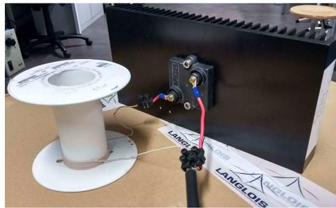
Figure 4.11 – The RL series load connected to the two-conductor  $2.5\text{ mm}^2$  cable
