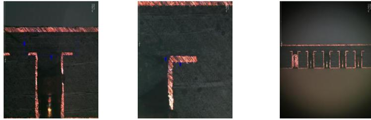
Figure 2-21: Cross-section view (Photograph) of internal metallized via holes
