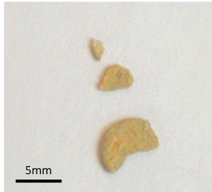
FIGURE 2.32: Reaction between the sample surface and the atmosphere powder in NBT-BT sample sintered using NBT + ZrO<sub>2</sub> powder to create the sintering atmosphere at 1050°C resulting in an inhomogeneous sample surface.
