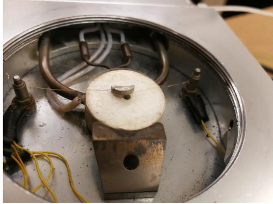
FIGURE 3.1: Picture of the impedance measurement device (Linkam).
