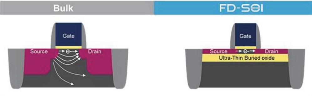
Figure 1.7: From Bulk-MOS Transistor to UTBB-FDSOI transistor (Source: ST.com)
