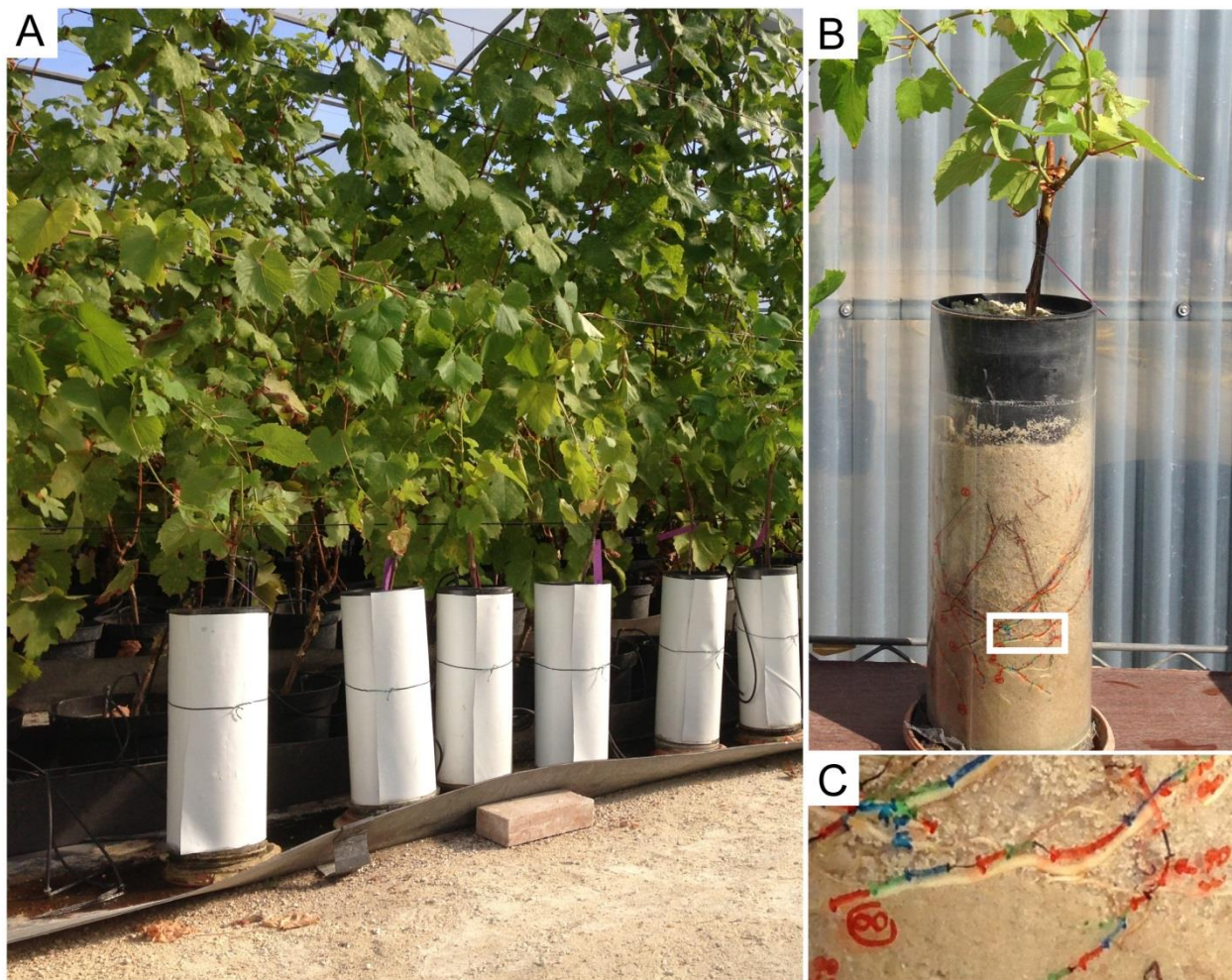
Figure 3.1 Rhizotron system used in the experiments. Roots can be observed through the transparent walls of the cylinder rhizotron. A sheet of transparent film was attached around the cylinder and roots were followed every day with hand drawing. A piece of thick and non-transparent lightproof paper was wrapped around each rhizotron in order to prevent the exposure of roots to light.
