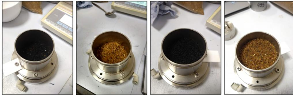
FIGURE 3.36. Snapshots for some steps in the experimental preparation of layers packing in the oedometer cell.
