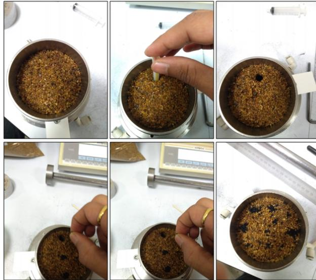
FIGURE 3.37. Snapshots for the experimental preparation of vertical stripes packing in the oedometer cell.
