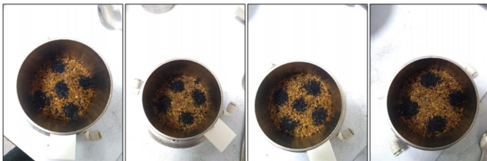
FIGURE 3.34. Snapshots of some steps in the preparation of cluster packing arrangements of sand-rubber mixtures (10% rubber fraction arrangement is shown here).
