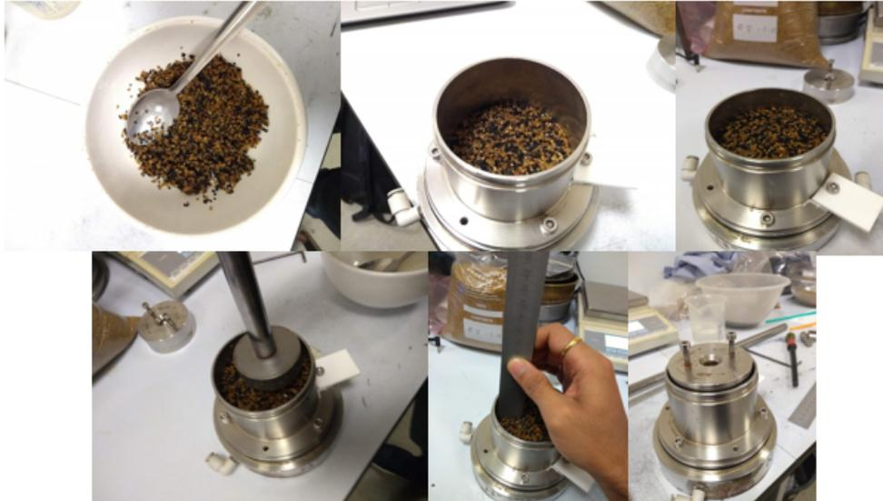
FIGURE 3.1. Preparation of sand-rubber mixtures using moist tamping method
