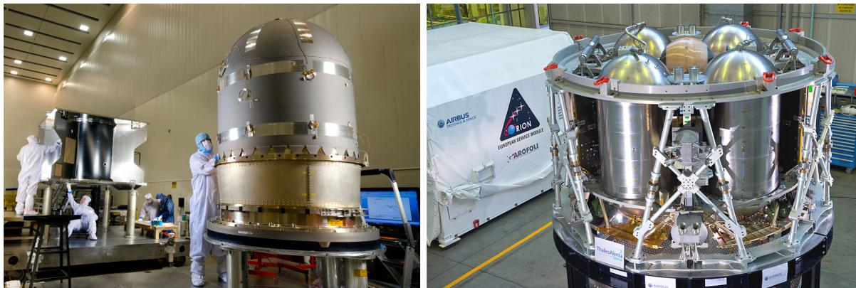
Figure 1.2 – **Left figure:** Hydrazine propellant tank built for NASA’s MAVEN spacecraft. (Credit: Lockheed Martin). **Right figure:** Bipropellant tanks integrated to the Structural Test Article of Orion’s European Service Module before delivery to NASA Glenn (Image taken from [1]).
