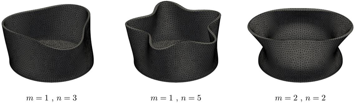
Figure 3.2 – Example of three hydroelastic eigenmodes.
