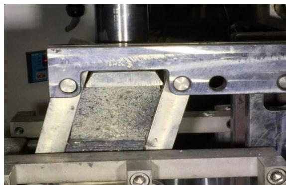
Figure 1. 25: Experimental proposed device for shear strength investigation.
