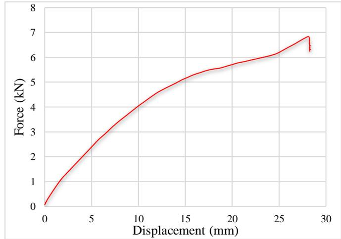
Figure 2.20: Force-displacement behaviour for OSB wall.
