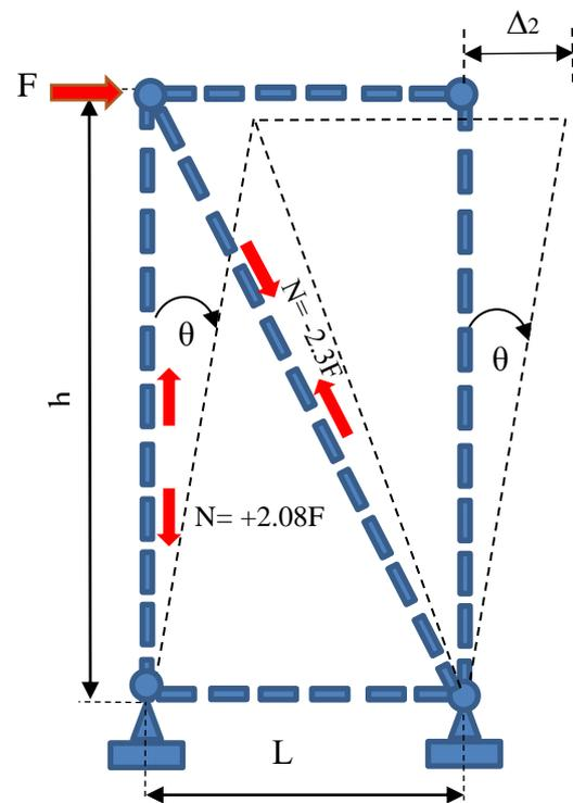
Figure 3. 2: Loaded and unloaded states of diagonal bracing wall unit.
