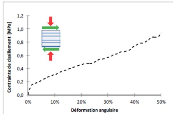
Figure 1. 23: Shear perpendicular to the direction of fabrication with vertical load 1 MPa.
