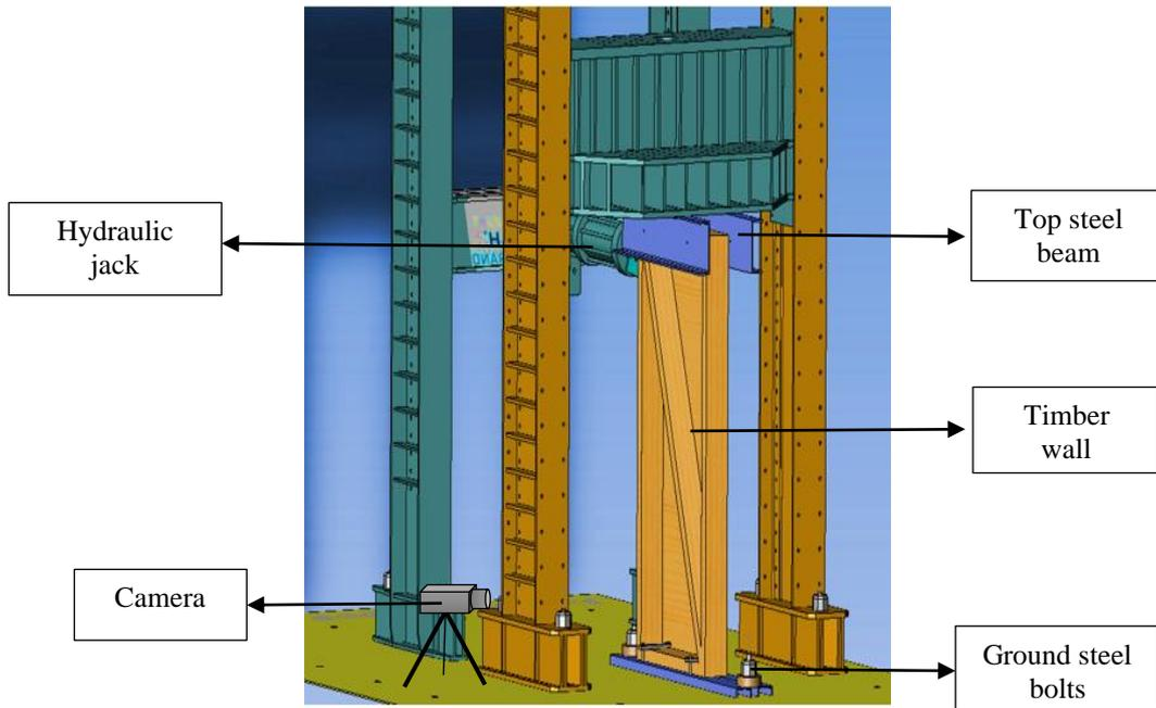
Figure 3. 10: The test setup for timber walls.
