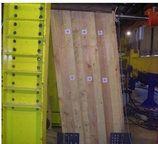
Figure 2. 13: Timber wall of first group (S1) in test.
