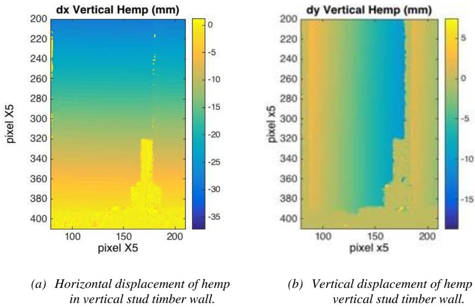
Figure 3. 21: Example of displacement fields of hemp concrete in vertical stud timber wall (V-H-2) for an overall horizontal displacement at the top of the wall equal to 50mm.
