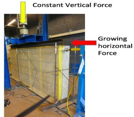
Figure 1. 38: Mechanical test of the wall.
