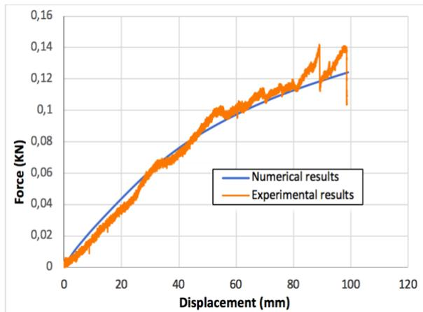
Figure 4. 7: Comparison between the experimental and the numerical results.
