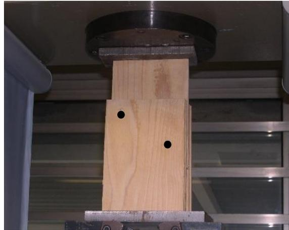
Figure 2.11: Shear test set up for fasteners.
