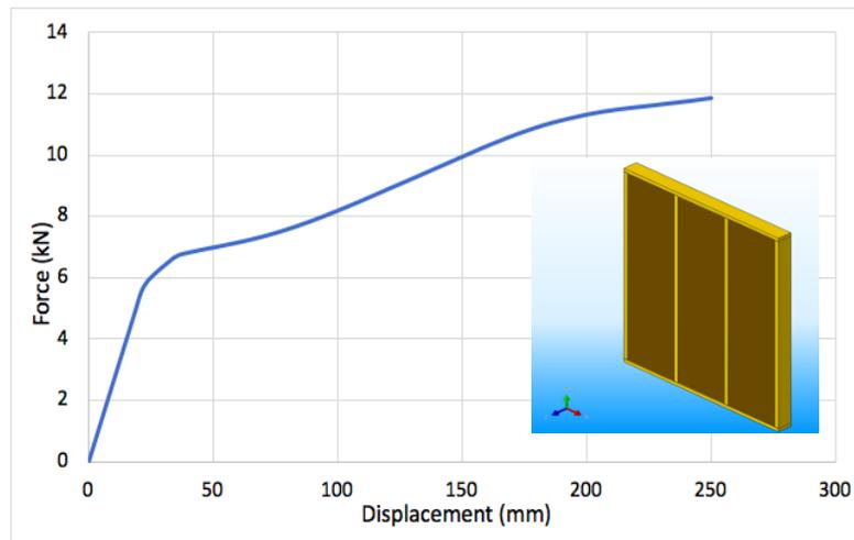
Figure 4. 15: Lateral strength of hemp wall three panels with length 1.8 m.
