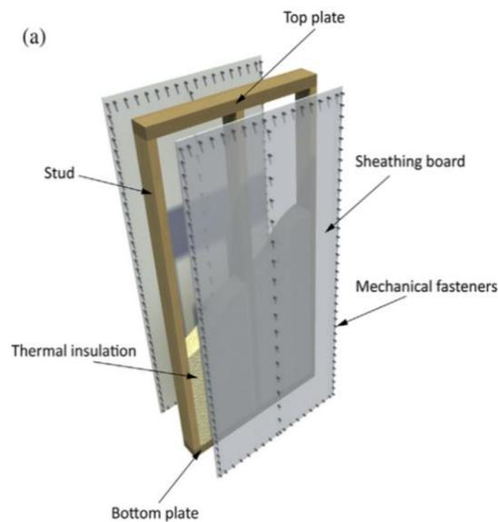
**Figure 1. 29: Composition of single panel wall element.**
