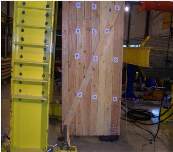
**Figure 2. 15: Timber wall of the second group (S2) in test.**
