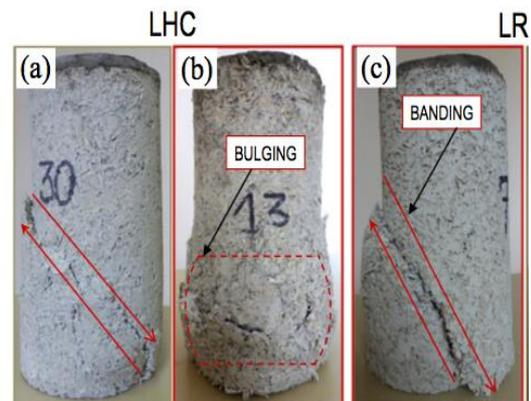
Figure 1. 21: Shear banding (a) and (c), bulging failure (b).
