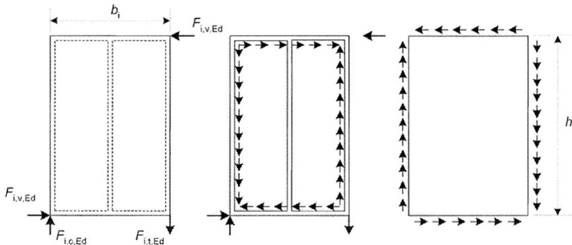
**Figure 1. 27: Forces distribution on wall panels according to Eurocode (5).**
