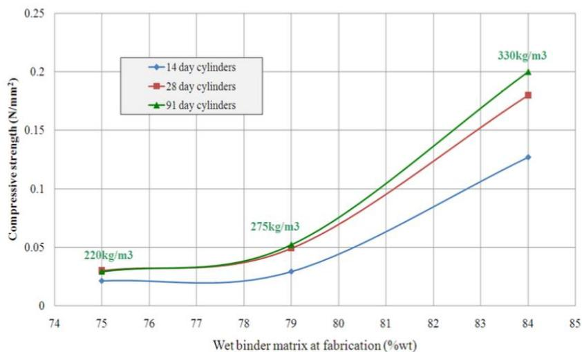
Figure 1. 17: Compressive strength vs. wet binder percentage of THB (Tradical™ Binder) specimens.
