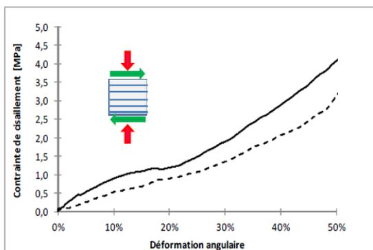
Figure 1. 24: shear applied perpendicular to the direction of fabrication with vertical load 1MPa dotted line and 2 MPa solid line.
