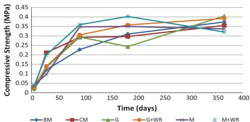
**Figure 1. 13: Compressive strength of hemp-lime concretes over time.**
