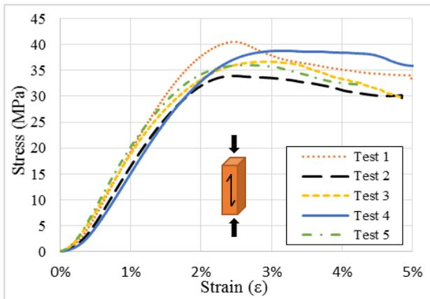
Figure 3.3: Stress-strain diagrams of timber sample behaviour parallel to the grain.
