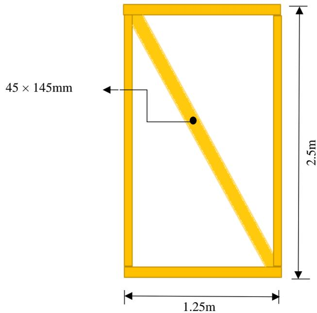
**Figure 3. 8: Diagonal bracing wall details.**
