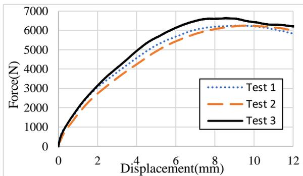
Figure 2.12: Simple shear behaviour of nail fasteners.
