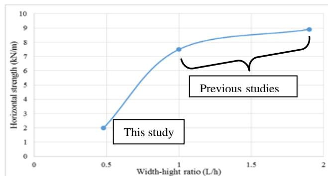
Figure 3.26: Comparison of racking strength of timber hemp wall with different width-height ratios.
