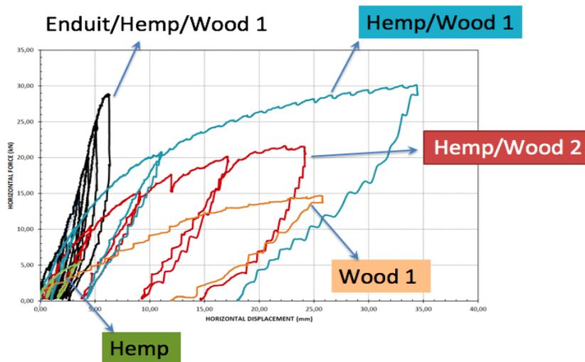
Figure 1. 39: Racking Strength of tested walls.
