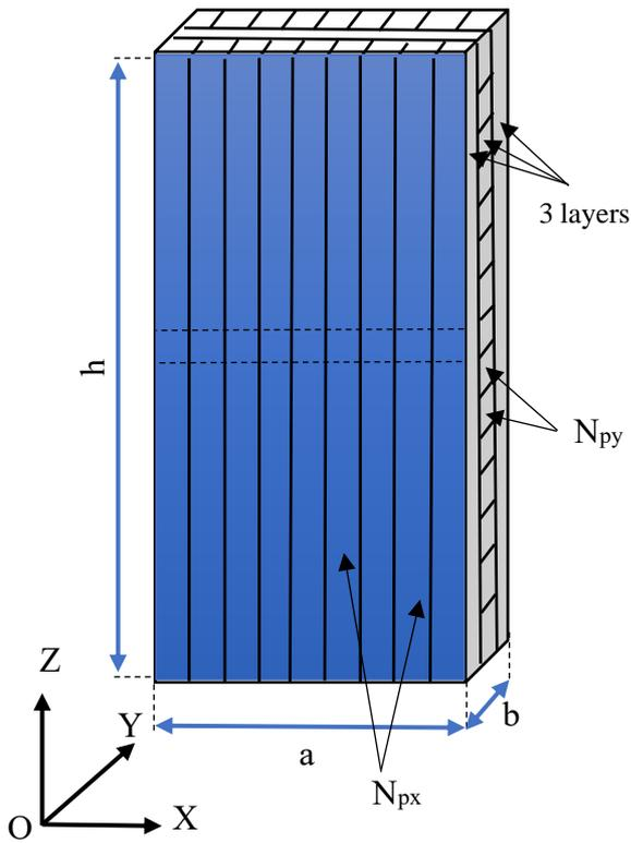
Figure 2. 3: Timber cross-laminated wall.
