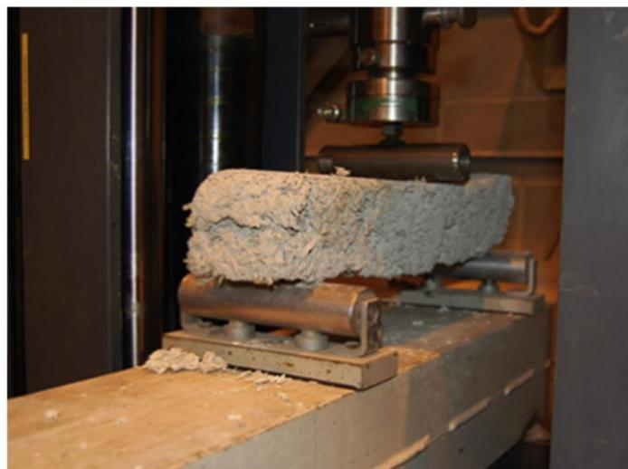
Figure 1. 18: Typical deflection of hemp-lime concrete in bending.
