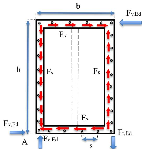
Figure 2. 23: fasteners behaviour as Eurocode 5 principle in OSB panel.
