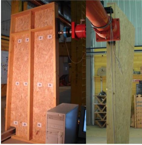
Figure 2.19: OSB wall during test.
