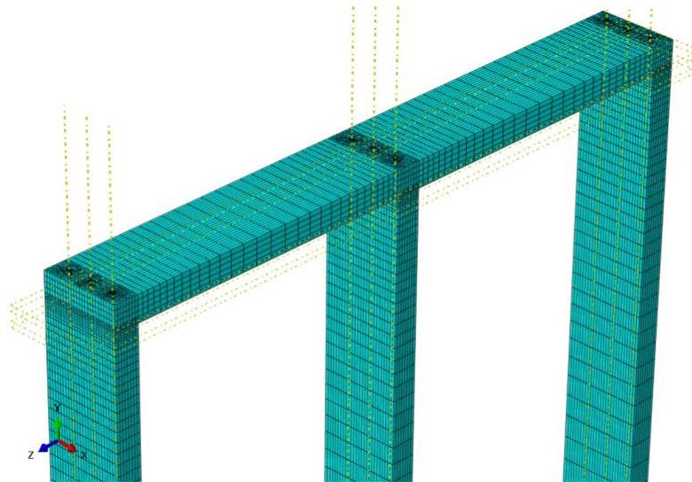
**Figure 4. 4: Mesh of Finite Element Model for timber frame wall.**
