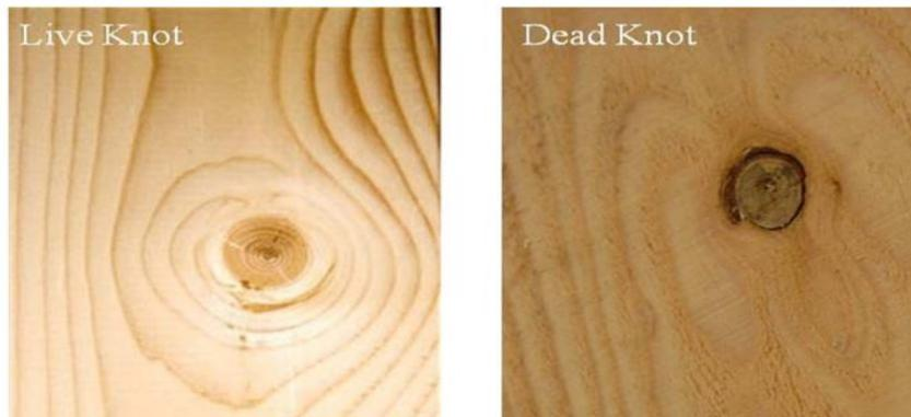
Figure 1. 5: Live and Dead Knots in Timber.
