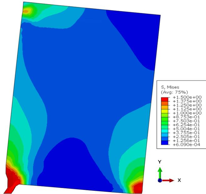
Figure 4. 19: Stresses distribution in hemp wall with four panels.
