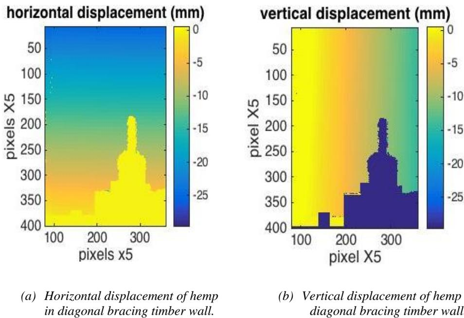
Figure 3. 22: Example of displacement fields of hemp concrete in diagonal bracing timber wall (D-H-2) for a global horizontal displacement at the top of the wall equal to 50mm.
