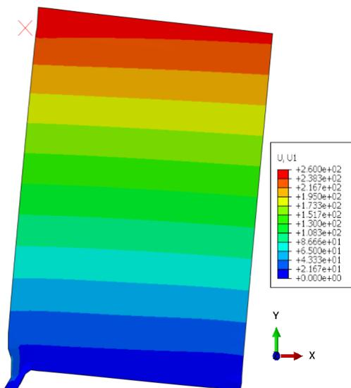
Figure 4.17: Lateral displacement of hemp wall with four panels.
