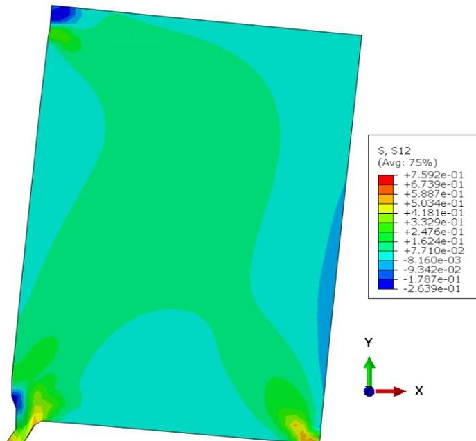
Figure 4. 20: Stresses distribution in x-y directions in hemp wall with four panels.
