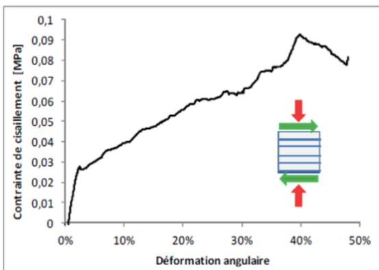
Figure 1. 22: shear perpendicular to the direction of fabrication with vertical load 0.2 MPa.
