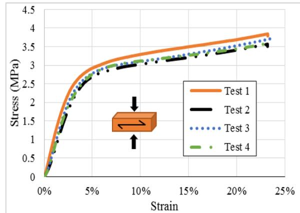
Figure 3.4: Stress-strain diagrams of timber samples behaviour transversally to the grain.
