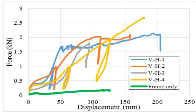
Figure 3.24: Comparison between empty frame and vertical stud hemp walls.
