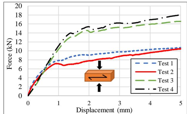
Figure 2. 10: Compressive timber behaviour transverse to the grain.
