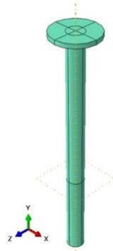
Figure 4. 2: The represented nail at the timber joints between rails and columns.
