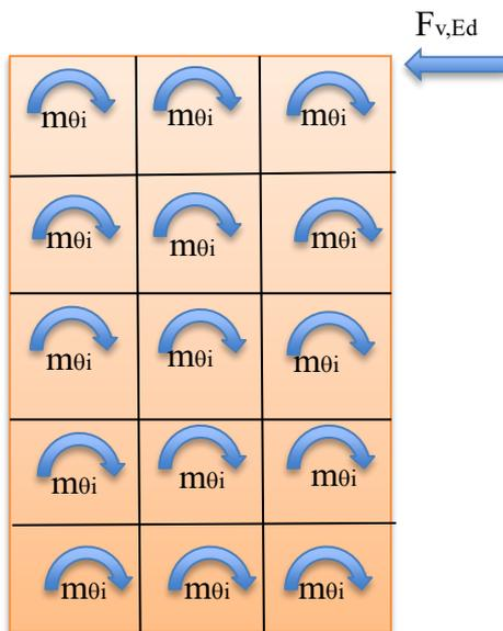
Figure 2. 22: Internal resistance of rotational moments for cross-laminated wall.
