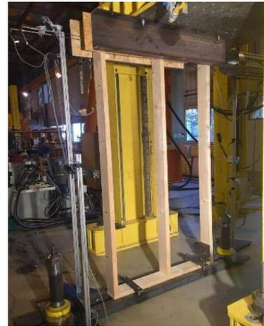
Figure 4. 8: Empty timber frame in test.
