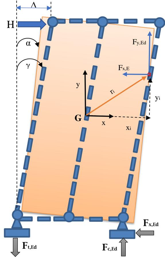
Figure 2. 2: Loaded state of timber frame.
