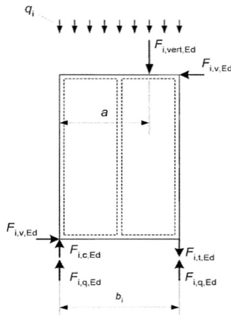
Figure 1. 28: Determination of equivalent vertical action  $q_i$  in method (B).
