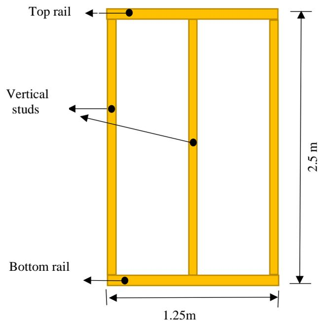
Figure 3. 7: *Vertical stud wall details.*
