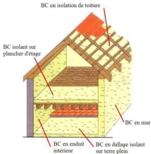
Figure 1. 10: hemp concrete applications.
