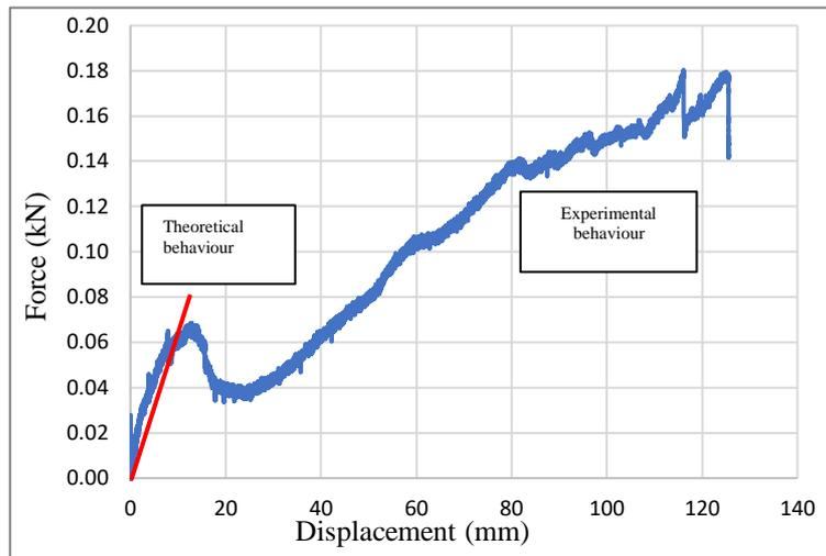
Figure 3. 14: Force-Displacement behaviour for frame only.
