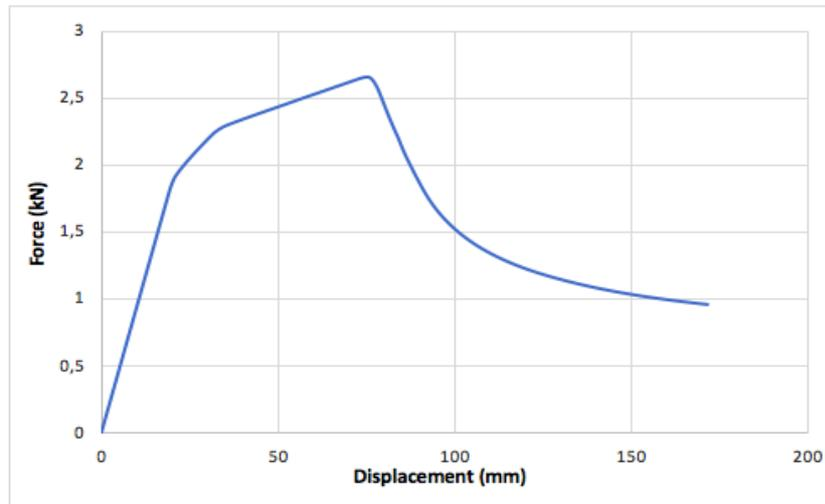
Figure 4. 12: Elasto-plastic behaviour of timber wall filled with hemp.
