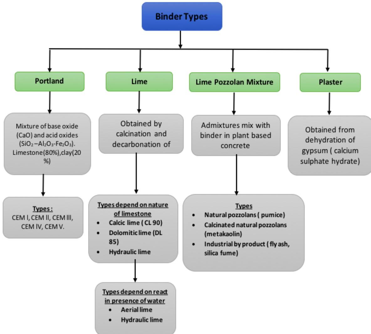
Figure 1. 12: Binder types used in concretes.
