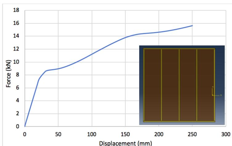
Figure 4. 16: Lateral strength of hemp wall four panels with length 2.4 m.
