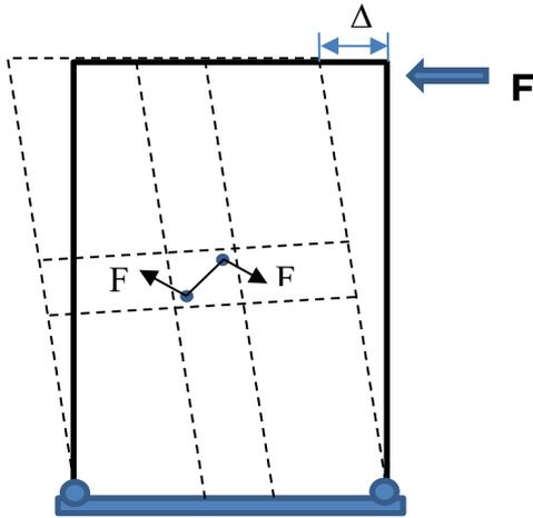
Figure 2. 7: The deformation of the cross-laminated wall.
