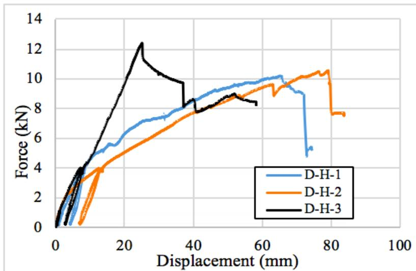
Figure 3. 20: Force-Displacement behaviour for diagonal bracing hemp walls.
