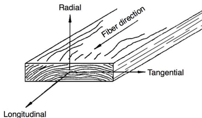
Figure 1. 4: Three principal axes of wood with respect to the grain direction.
