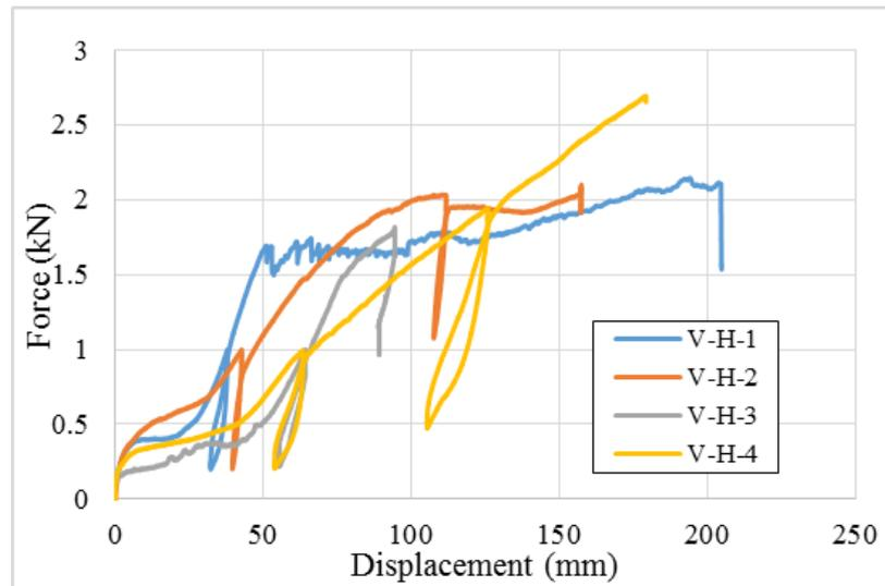
Figure 3. 16: Force-Displacement behaviour for vertical stud hemp wall.
