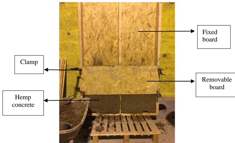
Figure 3. 9: Casting protocol of vertical stud timber wall.
