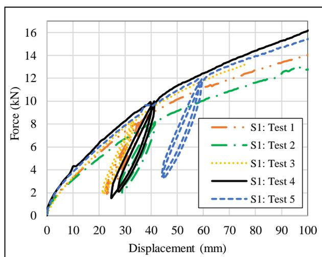
Figure 2. 14: Force-displacement behaviour for (S1)
