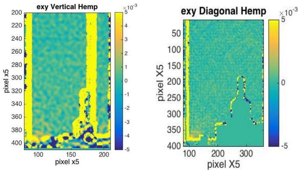
(a) Shear strain of hemp in vertical stud timber wall in (V-H-2).
