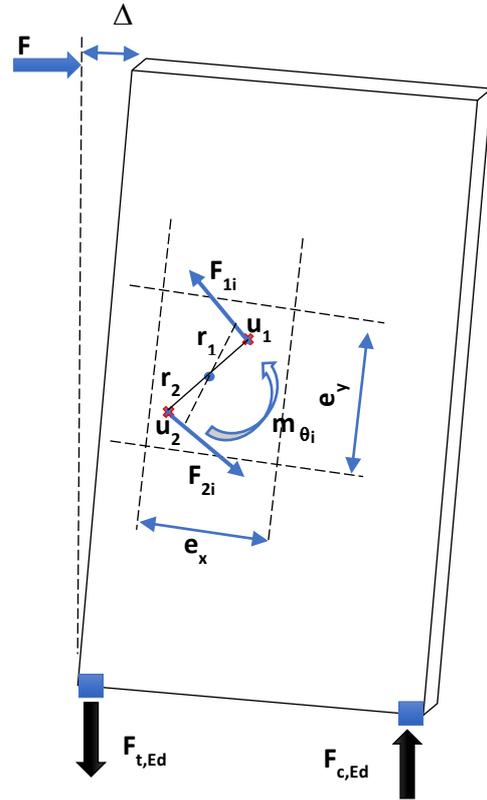
Figure 2. 4: Intersection plane of the fasteners.
