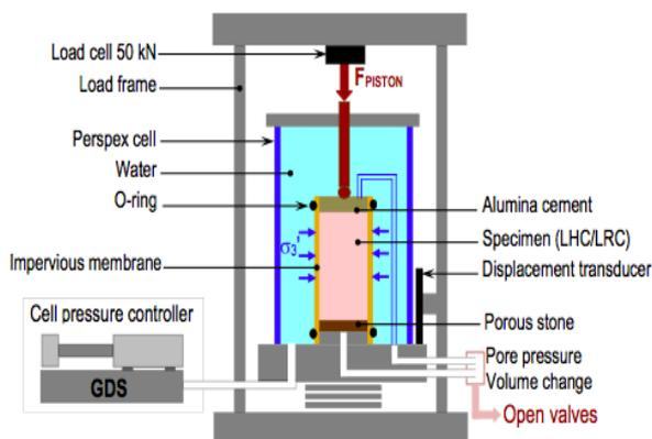
Figure 1. 20: Device of triaxial shear test on plant-based concrete.
