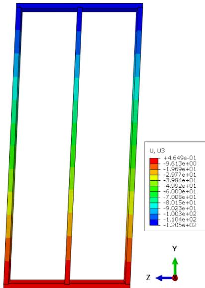
Figure 4. 5: The deformed shape showing the displacement in z-direction.
