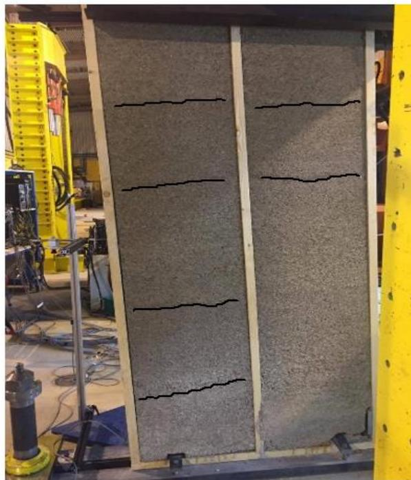
Figure 3. 15: Vertical stud hemp wall in test.
