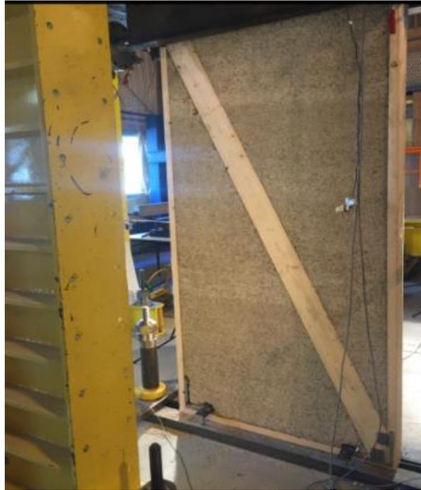
Figure 3. 19: Diagonal bracing hemp walls in test.
