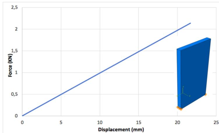
**Figure 4. 11: Lateral resistance of wall in linear behaviour and simply support foundation.**
