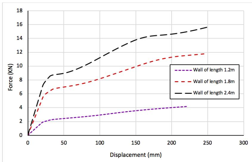
Figure 4. 21: Comparison between numerical results with different wall lengths.
