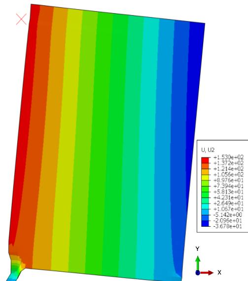
Figure 4.18: Vertical displacement of hemp wall with four panels.
