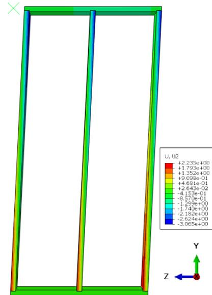
Figure 4. 6: The deformed shape showing the displacement in y-direction.
