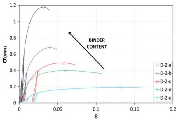
Figure 1. 15: Compressive strength tests of different binder content.
