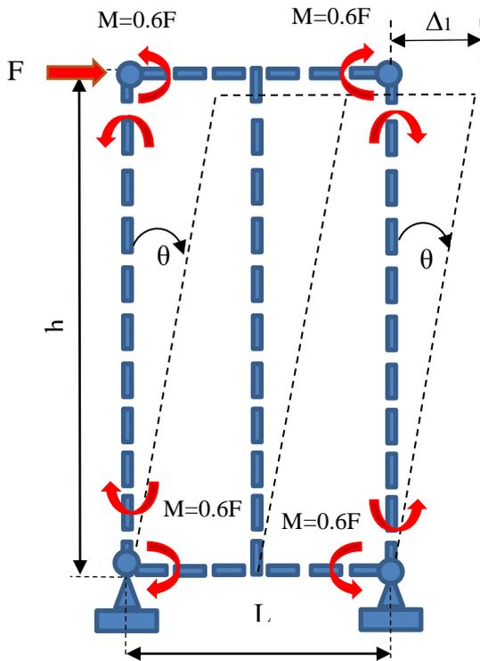
Figure 3. 1: Loaded and unloaded states of vertical stud wall unit.
