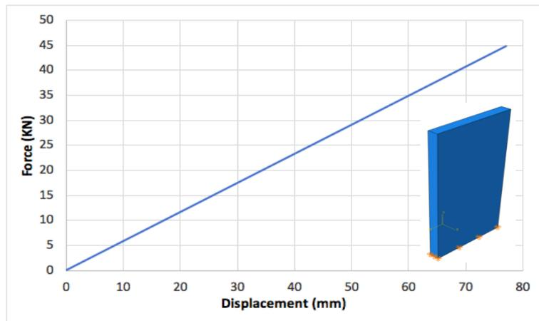
**Figure 4. 10: Lateral resistance of wall in linear behaviour and fix support foundation.**
