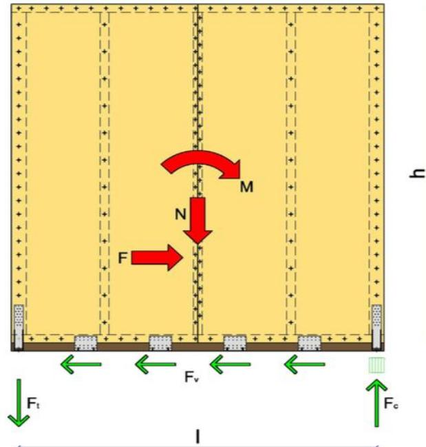
**Figure 1. 31: Role of the connection system between vertical panel and horizontal diaphragm.**
