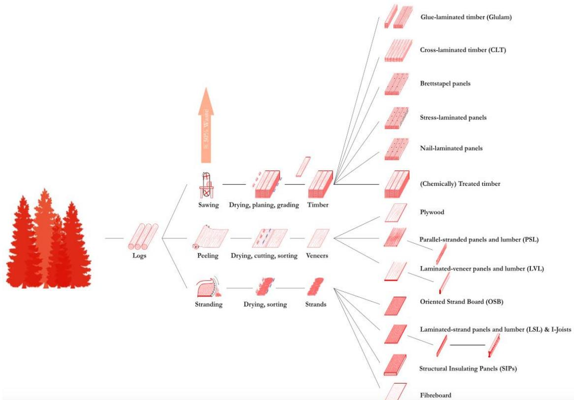
**Figure 1. 3: The processing chain of engineered timber products.**
