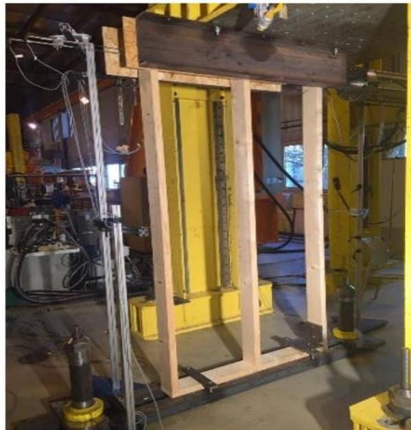
**Figure 3. 13: Empty vertical stud frame in test.**
