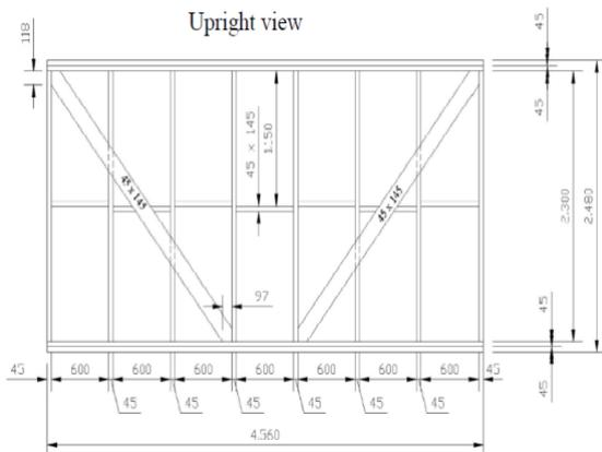
Figure 1. 32: Wood panel of the structure.
