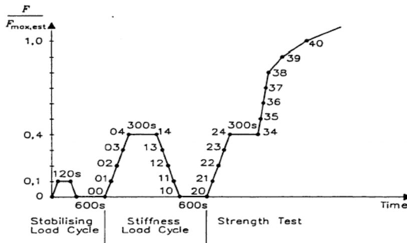
Figure 3. 11: Lateral load versus time for walls.
