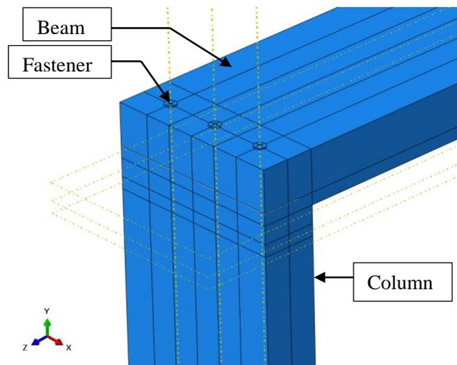
Figure 4. 3: Simulated timber joint with represented nails.
