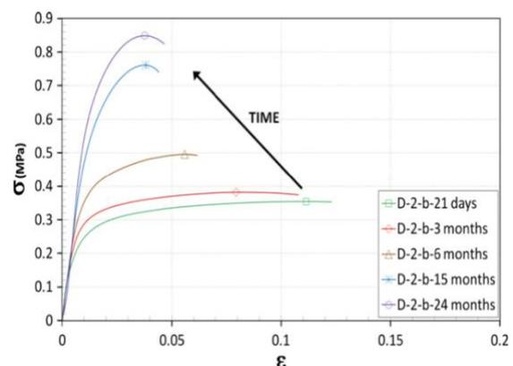
Figure 1. 16: Compressive strength of hemp samples for increasing ages.
