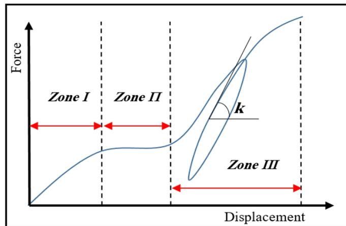
Figure 3.25: Representative curve for the lateral load resistance of vertical stud hemp wall.
