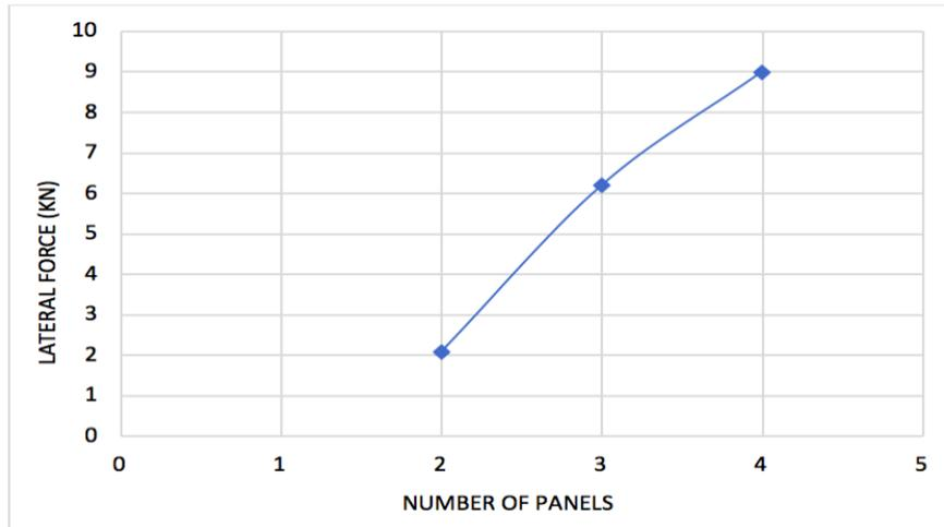
Figure 4. 22: Lateral strength vs number of panels in timber frame wall.
