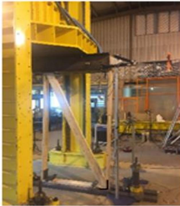
Figure 3. 17: Diagonal bracing walls in test.
