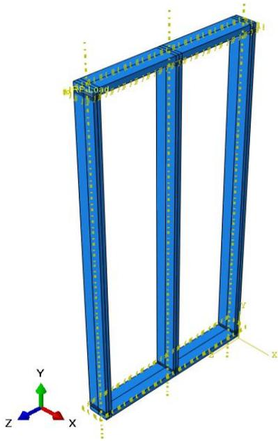
Figure 4. 1: Model geometry of the vertical stud timber wall.
