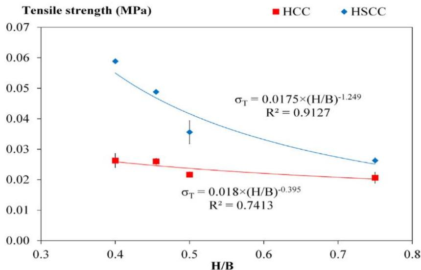
Figure 1. 19: Variation of tensile strength versus hemp to binder ratio(H/B).
