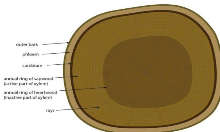
**Figure 1. 1: Tree cross section.**
