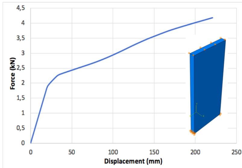
Figure 4. 13: Elasto-plastic behaviour of hemp wall with top boundary condition.
