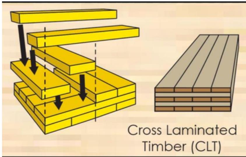
**Figure 1. 30: Cross laminated timber principle.**
