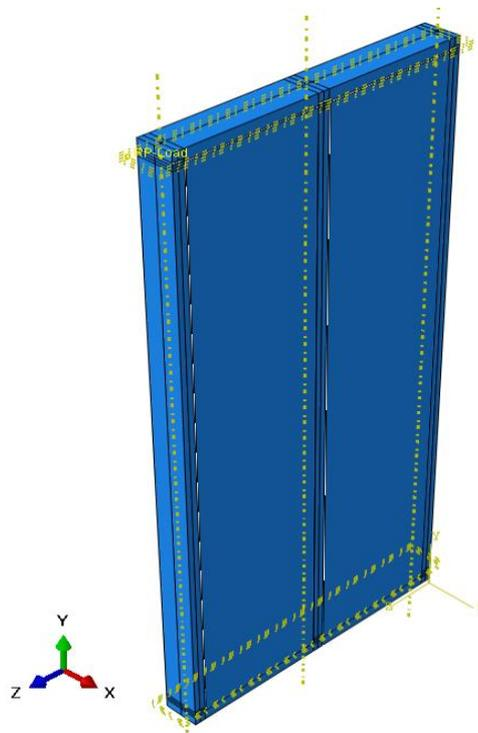
**Figure 4. 9: Model geometry of the vertical stud timber wall filled with hemp concrete.**
