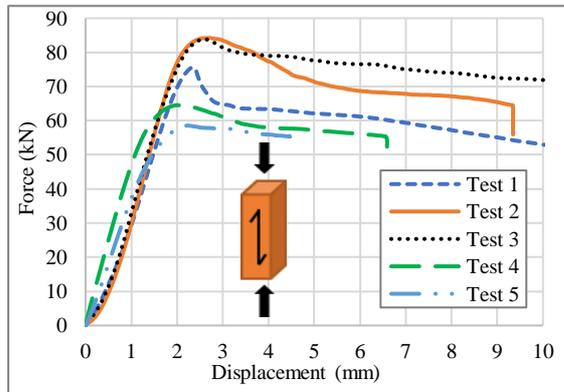
Figure 2. 9: Compressive timber behaviour parallel to the grain.
