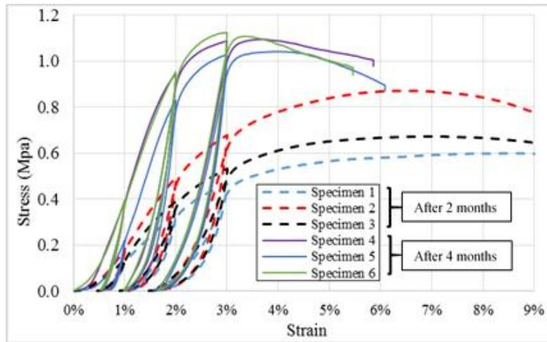
Figure 3. 5: Stress-strain behaviour of hemp concrete specimens.
