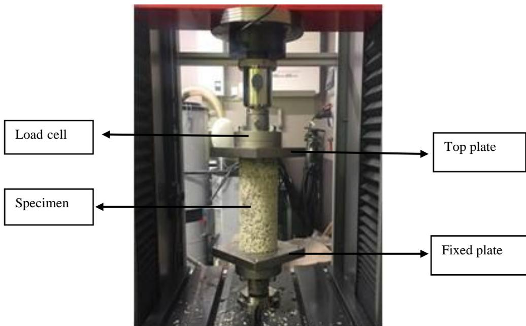
Figure 3. 6: Hemp concrete specimen in test.
