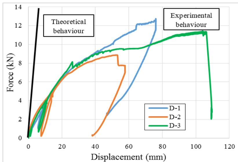
Figure 3. 18: Force-Displacement behaviour for diagonal bracing walls.
