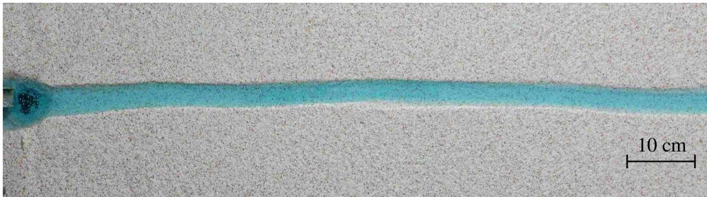
Figure 3.2 – Top view of a laboratory river. It corresponds to the experimental run 2 of table 3.1 ( $Q_w = 1.0 \text{ L/min}$  and  $Q_s = 0.42 \text{ g/min}$ ).
