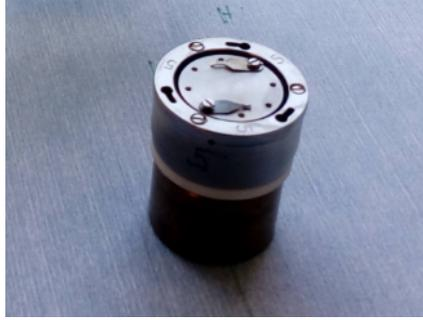
FIGURE 2.6: Picture of a sample holder bottom used for MEIS measurements. The adequate dimensions of a piece of sample should be  $1 \times 1 \text{ cm}^2$ , but the holder can also host a sample of extra dimensions with a rectangular or circular shape.
