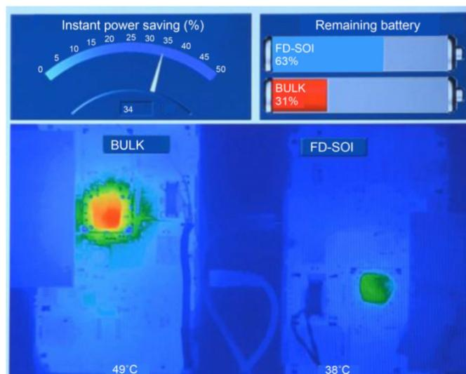
FIGURE 1.12: A demo of the power and temperature efficiencies of UTBB-FDSOI and bulk FinFETs[10].
