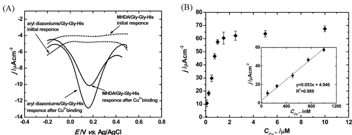
**Figure IV.10. Copper-binding tripeptide Gly-Gly-His-based electrochemical sensor, by Wawrzyniak *et al.*: (A) Square wave voltammograms of a carbon electrode modified with Gly-Gly-His before and after exposure to copper ions ( $0.1 \mu\text{M Cu}^{2+}$ ) in 50 mM ammonium acetate solution (pH 7.0),  $f=25 \text{ Hz}$ . (B) Plot of  $I_{\text{swv}}$  versus concentration of accumulated copper(II) ion <sup>(12)</sup>.**
