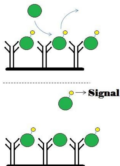
*Figure I.3. A competitive homogeneous immunoassay, unlabelled analyte displaces bound labelled analyte, which is then detected or measured.*
