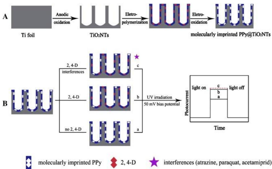
Figure III.5. Schematic illustration for (A) fabrication and (B) detection mechanism of the photoelectrochemical sensor<sup>(16)</sup>.
