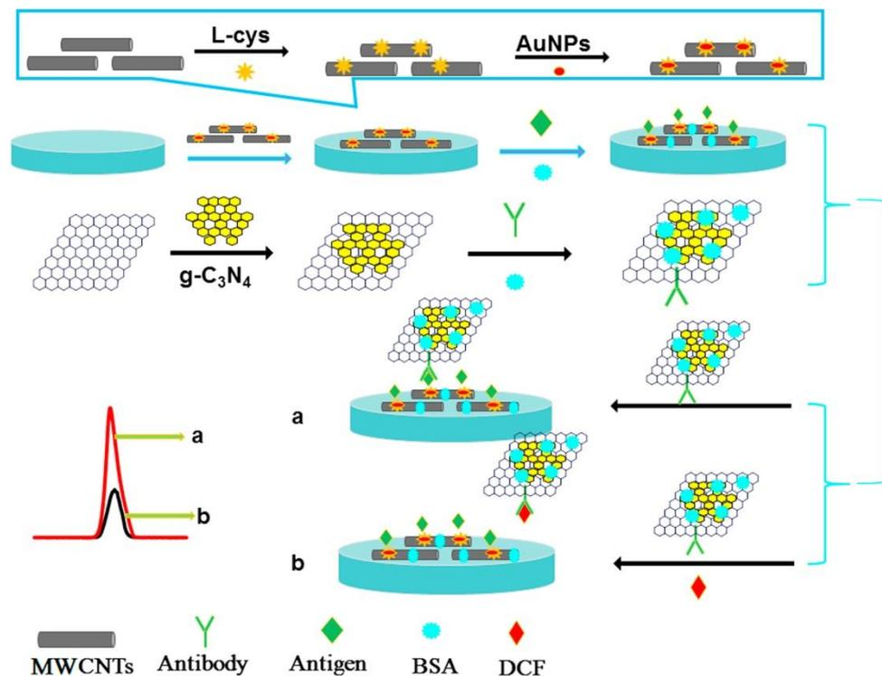
**Figure II.9.** ECL detection mechanism for DCF based on GCE/MWCNTs-AuNPs/coating antigen/BSA/GO-g-C<sub>3</sub>N<sub>4</sub> labeled DCF antibody<sup>(20)</sup>.
