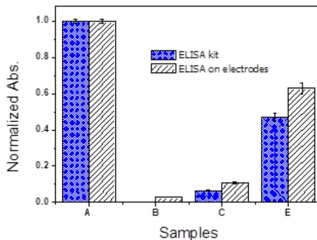
**Figure SI6.** Normalized absorbencies from ELISA tests: **A.** blank sample ( $Ab_{DCF}$  + secondary HRP-coupled Ab, no DCF added in solution); **B.** Control sample #1 ( $Ab_{DCF}$  +  $10^{-4}$  M DCF, no secondary HRP-coupled Ab); **C.** Control sample #2 (no  $Ab_{DCF}$ , secondary HRP-coupled Ab +  $10^{-4}$  M DCF); **D.** Sample ( $Ab_{DCF}$  + secondary HRP-coupled Ab +  $10^{-4}$  M DCF). For all experiments:  $[Ab_{DCF}] = 10^{-8}$  M in all experiments.
