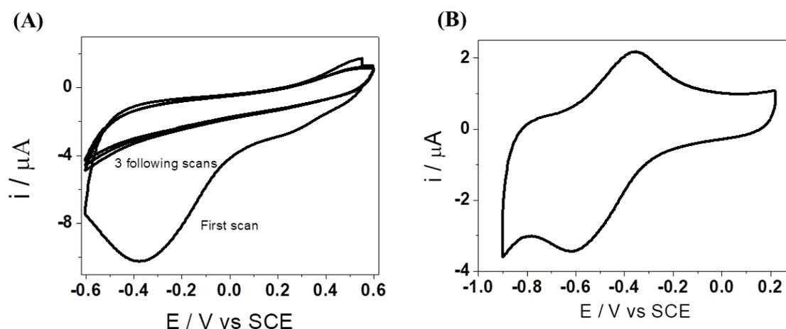
**Figure 2:** (A) Cyclic voltammograms corresponding to the electrografting of the DCF-Probe and E-Probe on a GC electrode. Scan rate  $100 \text{ mV s}^{-1}$ . (B) CV of a DCF-Probe/E-Probe/GC electrode in PBS. Scan rate  $50 \text{ mV s}^{-1}$ . Area =  $0.07 \text{ cm}^2$ . Solutions deaerated with argon.
