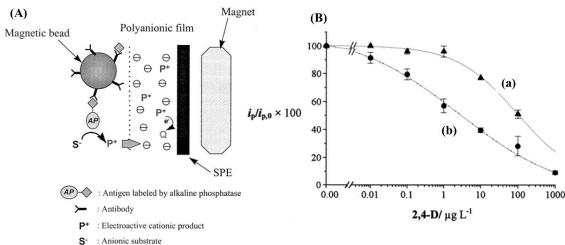
**Figure III.1.** The magnetic electrochemical immunosensor for 2,4-D detection: (A) Schematic representation of the key step of (B) Calibration curve of 2,4-D obtained for (a) 50 and (b) 15 µL of Ab-MBs stock solution incubated for 40 min at room temperature (total assay volume of 250 µL).  $i_{p,0}$  corresponds to the peak current value obtained in the absence of 2,4-D. Methylene blue was used as mediator <sup>(9)</sup>.
