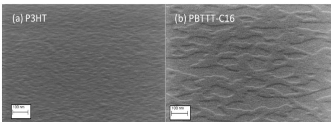
**Figure I.20. Lamellar structure of P3HT(a), pBTTT-C16 (b), normal or parallel to the substrate**<sup>(133)</sup>.
