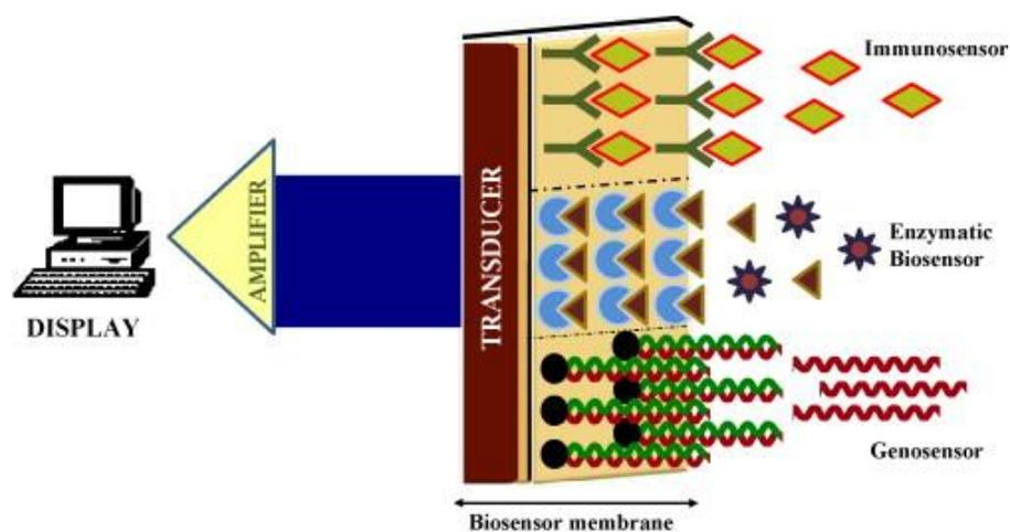
*Figure I.1. Schematic representation of a biosensor <sup>(14)</sup>*
