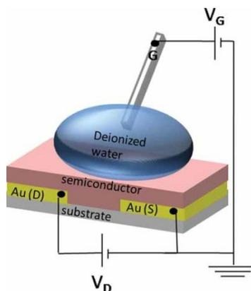
**Figure I.17. Scheme of the first water-gated EGOFET. The semiconductor was rubrene and the gate a platinum wire** <sup>(109)</sup>.
