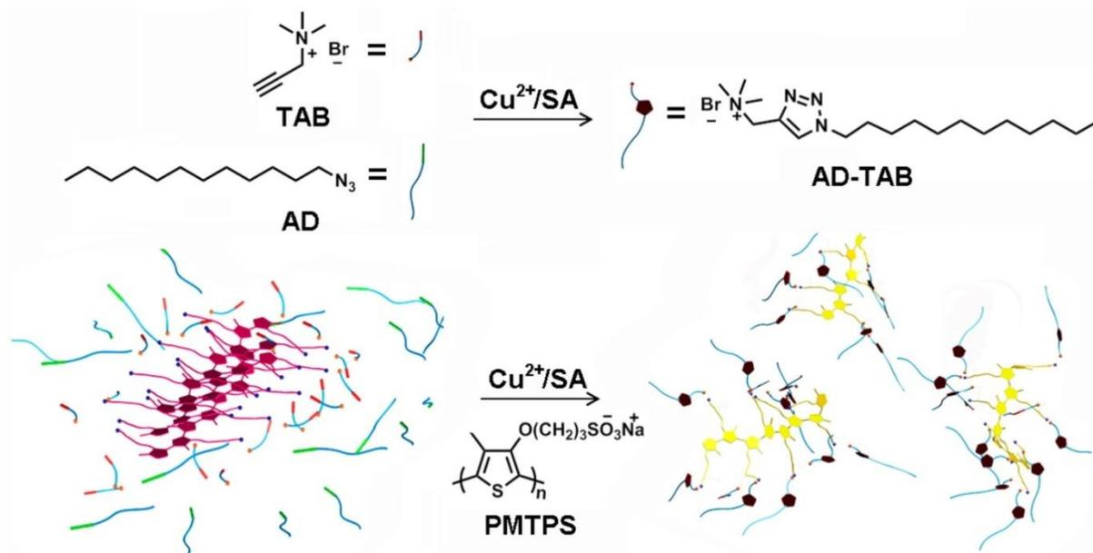
**Figure IV.2.** Chemical structure of PMTPS, illustration of the formation of AD-TAB and sensing mechanism for the detection of  $\text{Cu}^{2+}$  (3).
