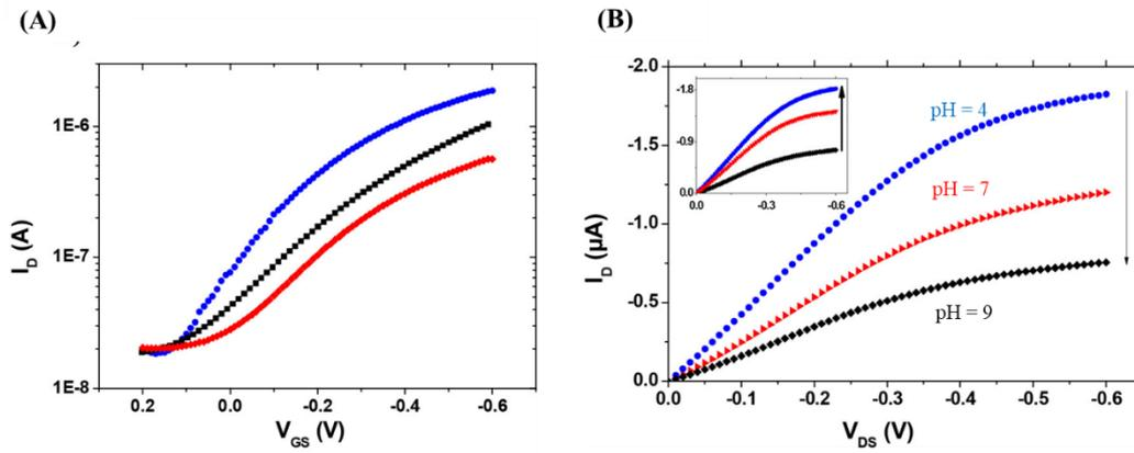
**Figure IV.7.** Electrical characteristics of an EGOFET with a hydrogel-modified gate electrode: (A) Transfer curves ( $V_{DS} = -0.6$  V) of a (●) bare Au-gated, (■) BrBD-functionalized, and (♦) AA-functionalized EGOFET. In all cases, the electrolyte was PBS. (B) Output curves ( $V_{GS} = -0.6$  V) of a PAA-functionalized EGOFET at different pH <sup>(6)</sup>.
