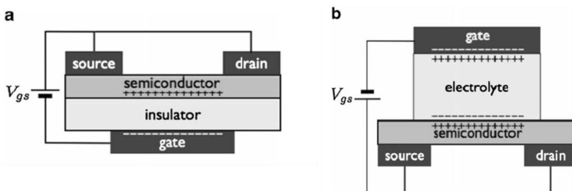
Figure I.15. General scheme of an OFET (a) and an EGOFET (b). <sup>(94)</sup>
