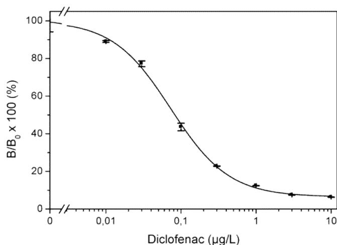
**Figure II.2.** Dose-response curve for diclofenac spiked into ultrapure water samples. Error bars represent the standard deviation and the ratio  $B/B_0$  (sample absorbance at a given DCF concentration over the maximum absorbance) <sup>(11)</sup>.
