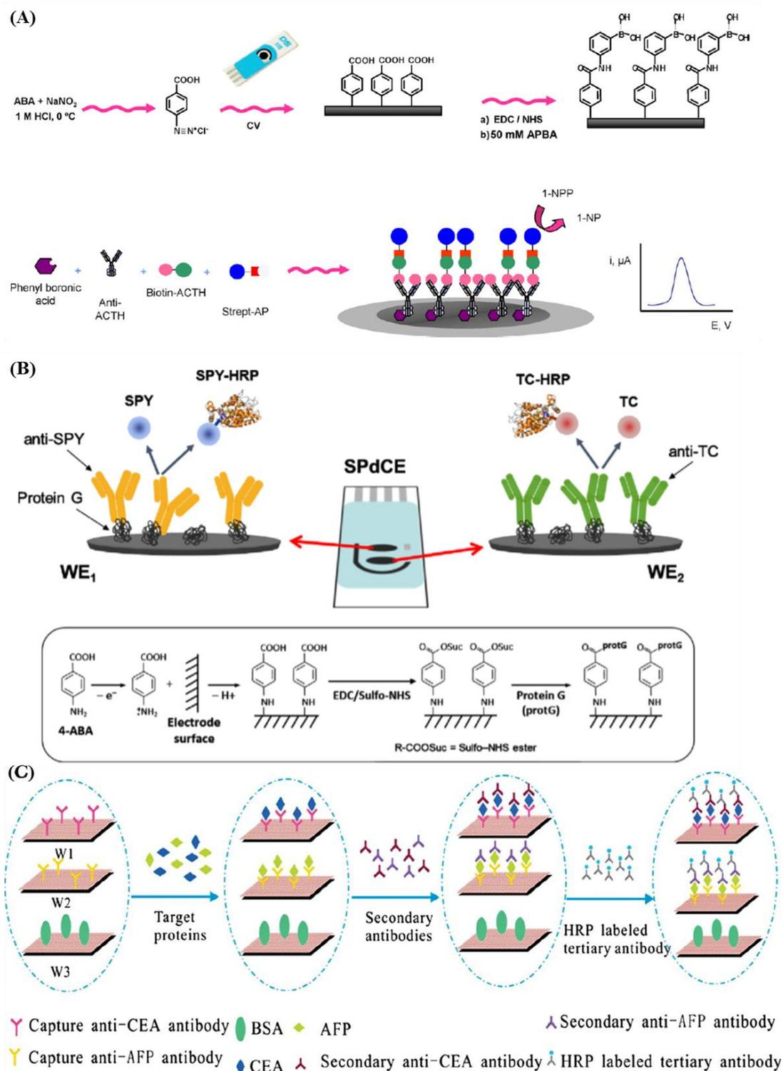
**Figure I.12. Illustration of antigen detections:** (A) Reactions involved in the ACTH immunosensor using SPEs modified with phenylboronic acid <sup>(49)</sup>. (B) Above, scheme of the immunosensor principle for SA and TC antibiotics. Below, surface chemistry involved for covalent binding of Protein G <sup>(56)</sup>. (C) Detection principle of the screen-printed bi-analyte array, including a BSA (reference) electrode <sup>(59)</sup>.
