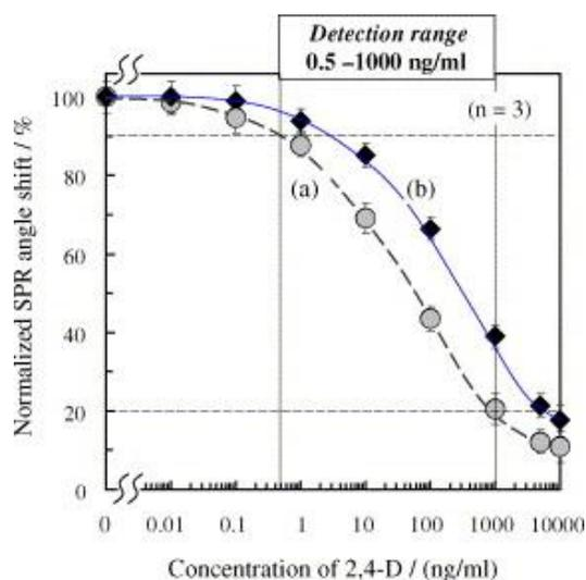
**Figure III.3.** Variation of normalized SPR angle shift with the concentration of 2,4-D in the competitive immunosensing experiments described in Fig. III.2 and the related text. Two different concentrations, 20 ppm (a) and 40 ppm (b), were used for the amount of antibody, 2,4-D-Ab<sup>(14)</sup>.
