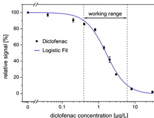
**Figure II.5.** Calibration curve obtained for DCF in pasteurised milk. The working range, between  $0.44$  and  $6.2 \mu\text{g L}^{-1}$  is indicated by dotted lines <sup>(16)</sup>.
