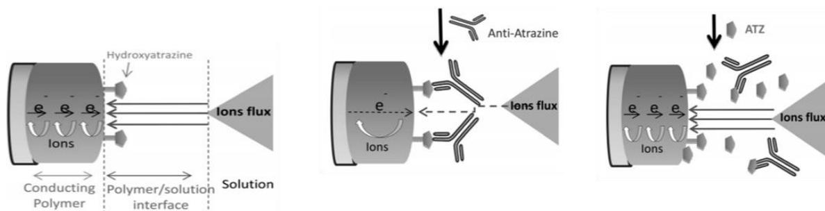
Figure I.7. Displacement assay coupled to an electrochemical transduction, by Tran *et al.* <sup>(54)</sup>.
