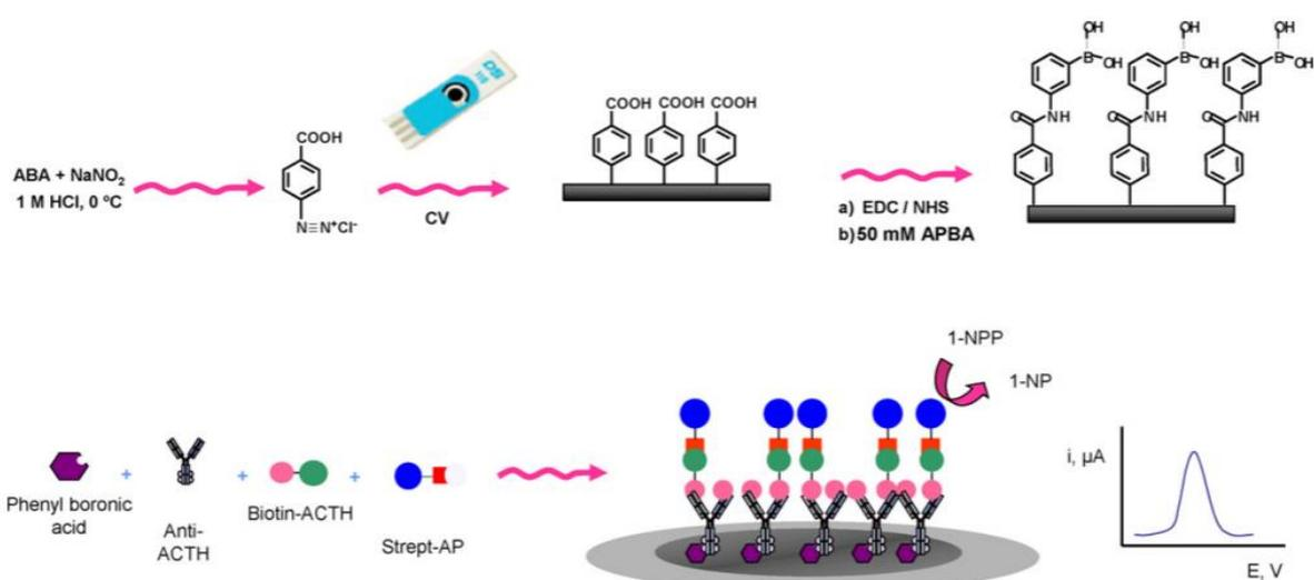
**Figure I.9.** Illustration of the different steps and protocols for adrenocorticotropin hormone (ACTH) detection via electrochemical immunosensor involved in the development of a disposable screen-printed electrodes modified with phenylboronic acid <sup>(49)</sup>.
