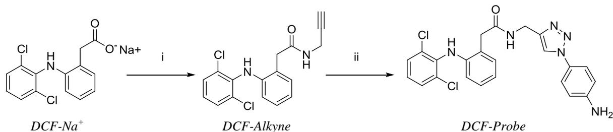
**Figure SI2.** Synthesis route for DCF-Probe, *N*-((1-(4-aminophenyl)-1H-1,2,3-triazol-4-yl)methyl)-2-((2,6-dichlorophenyl)amino)phenylacetamide. i) DMF, HATU, DIPEA, propargylamine, 50°C, 15h, 75%; ii) DCM/ $\text{H}_2\text{O}$ : 1/1,  $\text{CuSO}_4$ , L-ascorbate, 4-azidoaniline, 24h, 77%.
