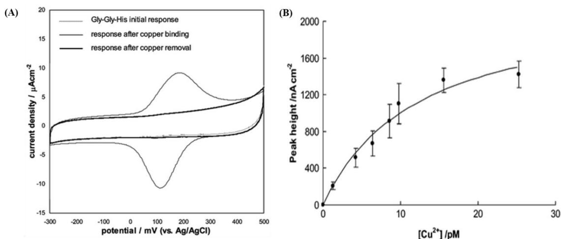
**Figure IV.9. Copper-binding tripeptide Gly-Gly-His-based sensor, by Yang *et al.* (2003) :** (A) Cyclic voltammogram of a Gly-Gly-His-modified electrode before and after exposure to copper in 0.05 M ammonium acetate buffer. (B) Plot of  $I_{\text{SWV}}$  vs. concentration of copper <sup>(10)</sup>.
