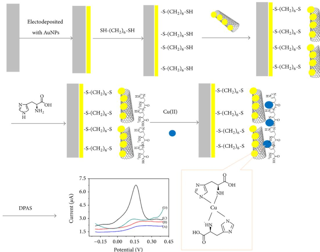
**Figure IV.5.** Principle of the sensor applying *L*-histidine immobilized on gold-labeled multiwalled CNTs proposed by Zhu et al. in 2017<sup>(5)</sup>.
