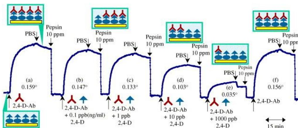
**Figure III.2.** SPR sensorgram observed under a flow of 2,4-D-Ab solutions of fixed concentration (20 ppm) over the 2,4-D-BSA immobilized sensor chip, in the absence and presence of 2,4-D at various concentrations: 0.1, 1, 10 and 1000 ppb <sup>(14)</sup>.
