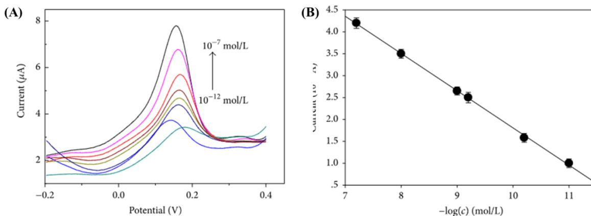
**Figure IV.6.** The Cu<sup>2+</sup> detection by *L*-histidine immobilized on gold-labeled multiwalled CNTs-based sensor (A) Stripping peak currents for various Cu<sup>2+</sup> concentrations; (B) Corresponding calibration curve<sup>(5)</sup>.
