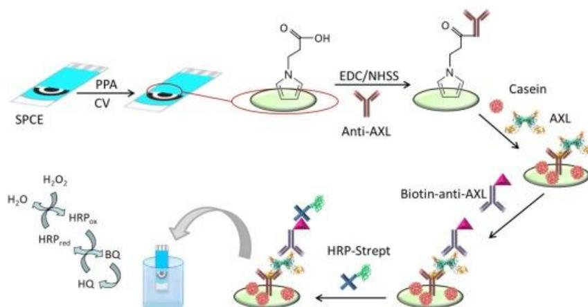
**Figure I.10.** Different steps construct the amperometric immunosensor for AXL detection involving pPPA-modified SPCEs and covalent immobilization of anti-AXL<sup>(53)</sup>.
