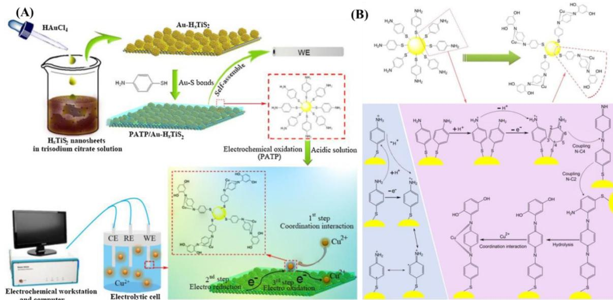
Figure IV.3. The electrochemical sensor for detection of  $\text{Cu}^{2+}$  applying PATP immobilized on AuNPs decorated with hydrogenated  $\text{TiS}_2$  nanosheets, by Gan et al. (2016). (A) Sensor design (B) Proposed mechanism for selective detection of  $\text{Cu}^{2+}$  (4)
