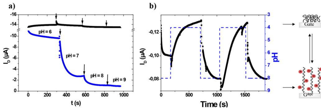
**Figure IV.8.** Plots of  $I_D$  for an EGOFET with a hydrogel-modified gate electrode, versus time: (a) ( $V_{GS} = V_{DS} = -0.4$  V) performed using a (black line) bare gate electrode and (blue line) a PAA-functionalized gate for successive pH jumps (values indicated on the graph); each arrow indicates injection of NaOH. (b) pH was abruptly varied from 8 to 4 and then back to 8 (twice) <sup>(6)</sup>.
