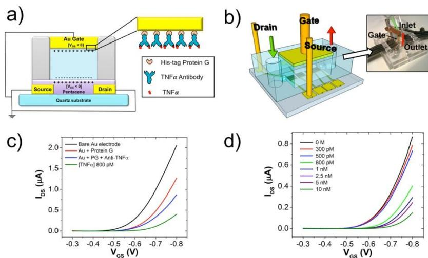
**Figure III.11.** EGOFET for monitoring tumor necrosis factor alpha (TNF $\alpha$ ) in human plasma: (a) Scheme of the EGOFET with a zoom on the functionalized gate. (b) Microfluidics device comprising the electrical connections and fluidic inlets and outlets. (c) Transfer curves recorded for each functionalization step. (d) Transfer curves upon exposure to various TNF $\alpha$  concentrations in PBS buffer<sup>(32)</sup>.
