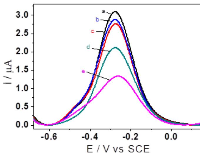
**Figure 3:** SWVs of (a) a  $DCF-Probe/E-Probe/GC$  electrode, (b) addition of  $5 \times 10^{-6}$  M  $Ab_{BPA}$ , (c) addition of  $5 \times 10^{-6}$  M  $Ab_{Ket}$ , (d) addition of  $5 \times 10^{-6}$  M  $Ab_{DCF}$  and (e) addition of  $5 \times 10^{-5}$  M  $Ab_{DCF}$ . SWV recorded in the oxidation direction from  $-0.55$  V to  $+0.05$  V<sup>1</sup> in deaerated PBS. Area  $0.07$  cm<sup>2</sup>.
