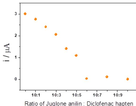
**Figure SI4.** SWV peak currents of a Ab/DCF-Probe/E-Probe/GC electrode for various ratio of E-Probe:DCF-Probe during electrografting. [E-Probe] kept constant at 1 mM and [DCF-Probe] varied between 0 and 1 mM.
