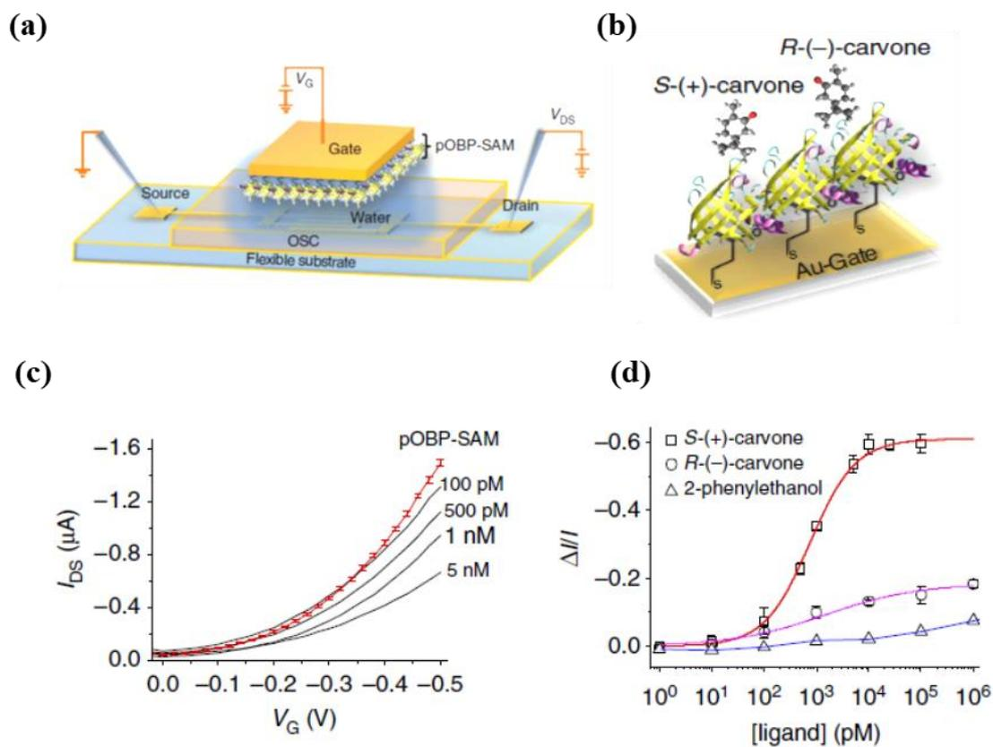
**Figure I.33.** EGO-FET where the gate is modified by a SAM of odorant binding protein (pOBP-SAM). (a) Schematic structure. The OSC is pBTTT-C14. (b) pOBP protein structure and interaction with the odorant molecule. (c)  $I_{DS}$ - $V_G$  transfer characteristics reported as a function of concentrations of the odorant molecule (carvone). (d) Calibration curves for the (R)-(-)- and (S)-(+)-carvone and for a non-specific molecule<sup>(156)</sup>.
