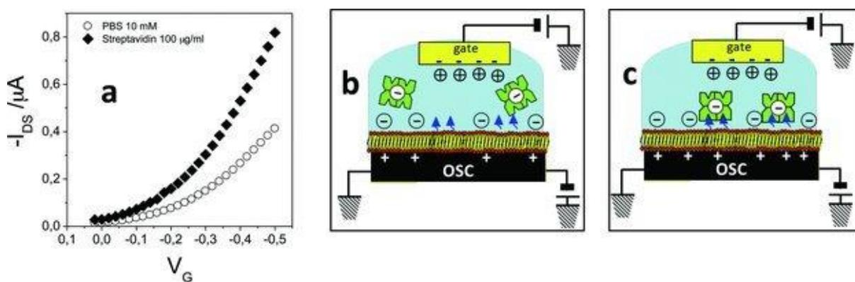
**Figure I.30.** Illustration of streptavidin detection via biotin-streptavidin binding: (a) Transfer characteristics of the biotin-functionalized phospholipid bilayer-EGOFET in PBS, pH 7.4 (open symbols) and streptavidin (plain symbols) solutions. (b) and (c) Diagram for the rationale leading to the  $I_{DS}$  current increase.
