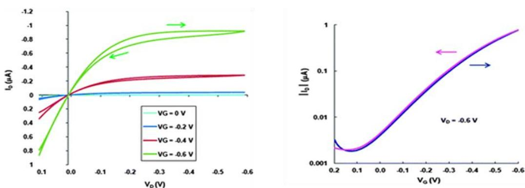
**Figure III.7. Output curves (left) and transfer curves (right) for a water-gated OFET based on P3HT-biotin <sup>(25)</sup>.**
