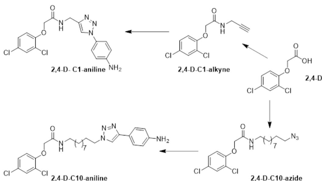
**Scheme 1:** Structure and synthesis of 2,4-D-C<sub>1</sub>-aniline and 2,4-D-C<sub>10</sub>-aniline.
