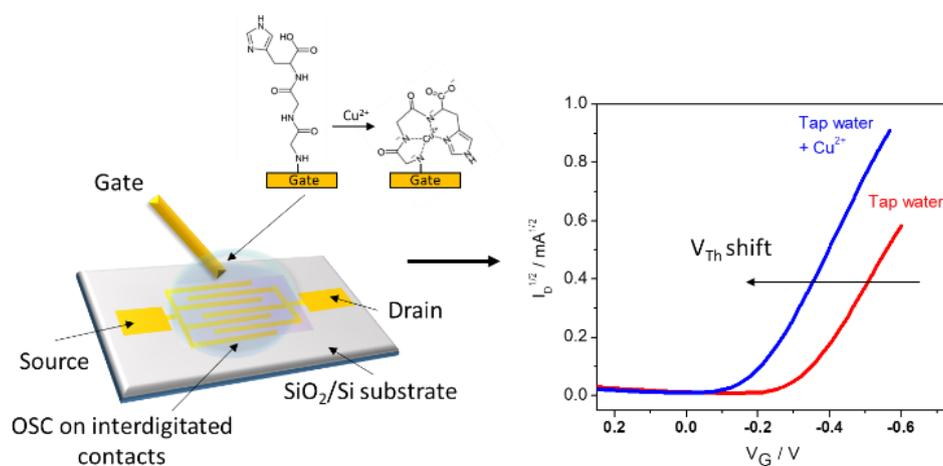
**Figure 1.** Schematic representation of the electrolyte-gated organic field-effect transistor with spin-coated DPP-DTT semiconductor on top of interdigitated source and drain contacts, tap water as electrolyte and a gold gate onto which GGH is grafted. Upon the presence of Cu<sup>2+</sup>, GGH folds, which modifies the gate/electrolyte interface and leads to a positive shift in threshold voltage.
