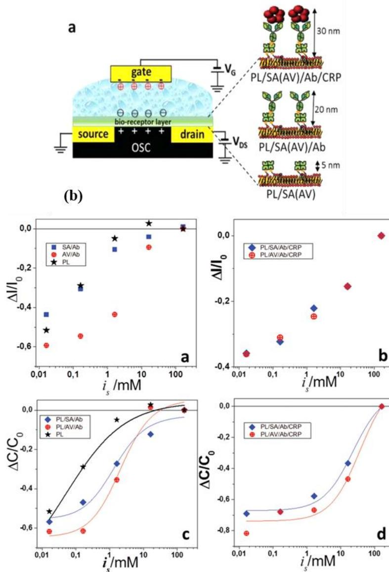
**Figure I.29. Illustration of CRP detection:** (A) Schematic view with different thicknesses of the bioreceptor layer. (B) Effect of the ionic strength on the fractional changes of the (a,b) current and (c,d) capacitance for a phospholipid/streptavidin/antibody (PL/SA/Ab) (a,c) and PL/SA/Ab/CRP (b,d) multilayers.
