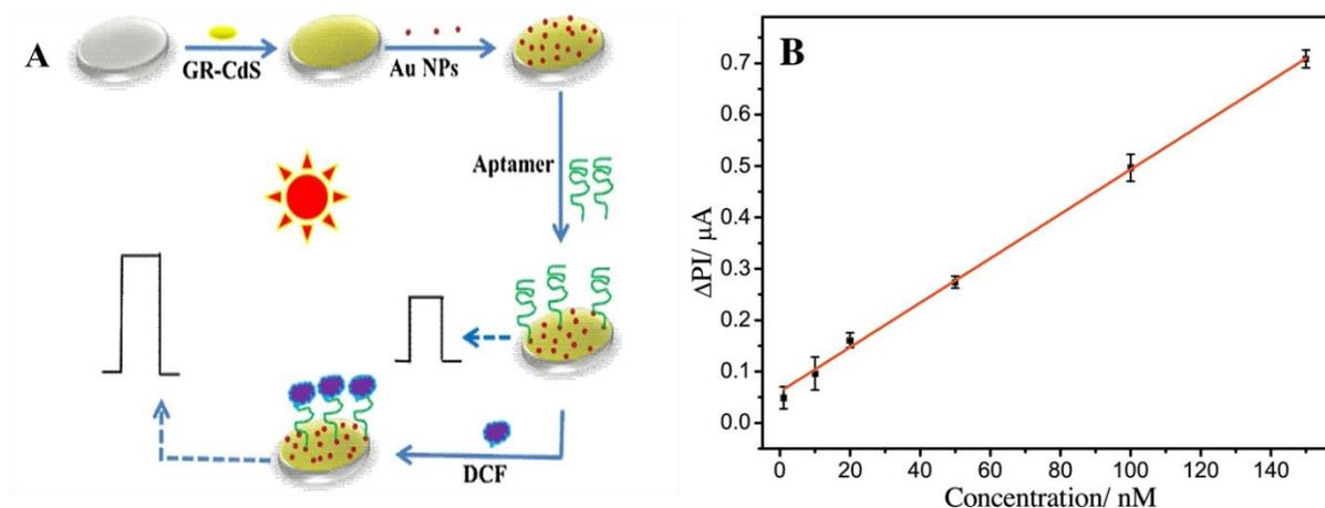
**Figure II.4.** Label-free aptasensor for DCF detection: (A) Fabrication process of the DCF aptasensor from Okoth *et al.*; (B) Corresponding calibration curve.  $\Delta PI$ : change in photocurrent intensity as a function of DCF concentration <sup>(15)</sup>.
