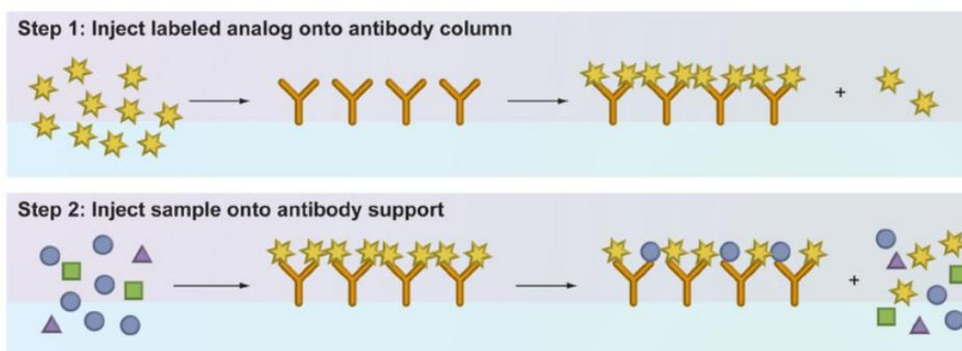
Figure I.6. General illustration of a displacement assay .
