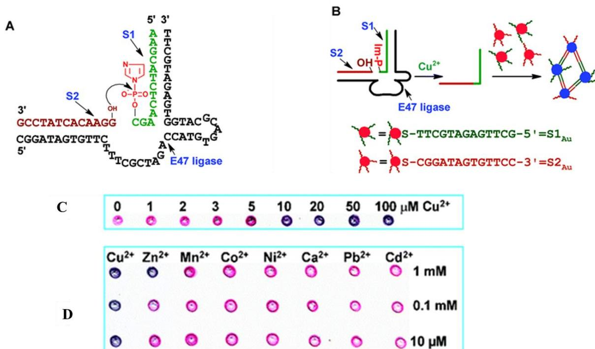
**Figure IV.1.** Cu<sup>2+</sup> detection using ligation DNAzyme complex assembled onto gold nanoparticles: (A) Secondary structure of the Cu<sup>2+</sup>-dependent DNAzyme with DNA ligation activity. (B) Formation of the ligation product and the assembly of AuNPs with it. (C) Colorimetric results for different Cu<sup>2+</sup> concentrations and (D) for different metal ions<sup>(1)</sup>.
