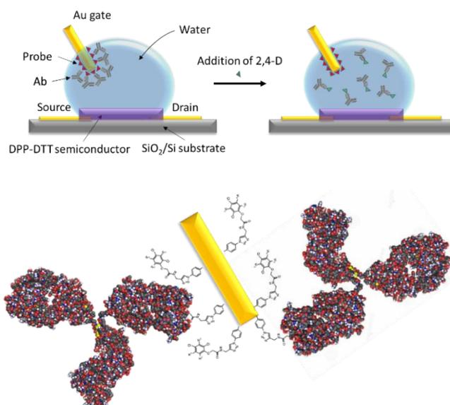
**Figure 1.** (Top) schematic view of the gate-modified EGOFET, before (left) and after (right) addition of the target molecule 2,4-D in the electrolyte. (Bottom) Antibodies immobilized by affinity interactions on the 2,4-D-modified gate.
