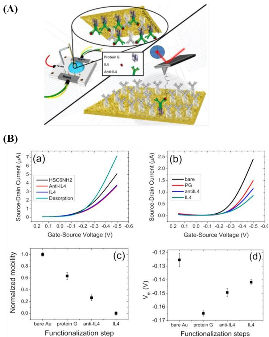
**Figure 1.32.** The gate-modified EGOFET for interleukin detection: (A) Schematic illustration of the modified gate and of the AFM measurements. (B) I-V transfer characteristics for (a) HSC<sub>6</sub>NH<sub>2</sub>- and (b) Protein G-based protocols. Normalized charge carriers mobility ratio (c) and threshold voltage (d) trends corresponding to the stepwise functionalization <sup>(190)</sup>.
