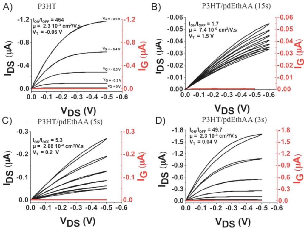
Figure I.27.  $I_{DS}$ - $V_{DS}$  curves of EGOFET devices fabricated with (a) pristine P3HT and (b), (c) and (d) with the pdEthAA/P3HT bilayer deposited by PE-CVD for 15, 5 and 3 s, respectively.  $L = 2 \mu\text{m}$  and  $W = 10\,000 \mu\text{m}$ <sup>(151)</sup>.
