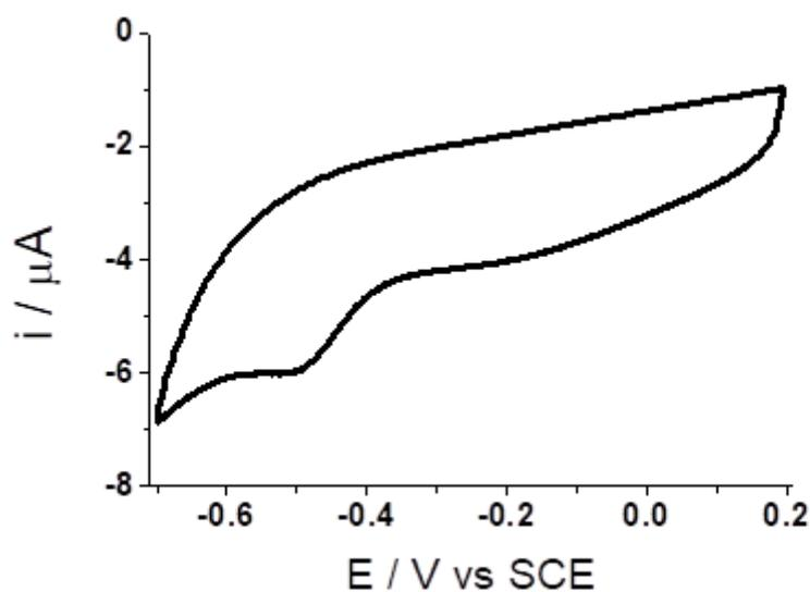
**Figure SI-2a.** Cyclic voltammogram corresponding to a 1 mm gold electrode, performed in degassed 5 mL  $\text{CH}_3\text{CN}$  + 190 mg  $\text{TBAPF}_6$  + 1 mg 2,4-D-aniline + 16  $\mu\text{L}$  tert-butyl nitrite. The potential of the gold electrode was swept from +0.2 V down to -0.7 V and back to 0.2 V at  $50\ \text{mV s}^{-1}$  for one cycle.
