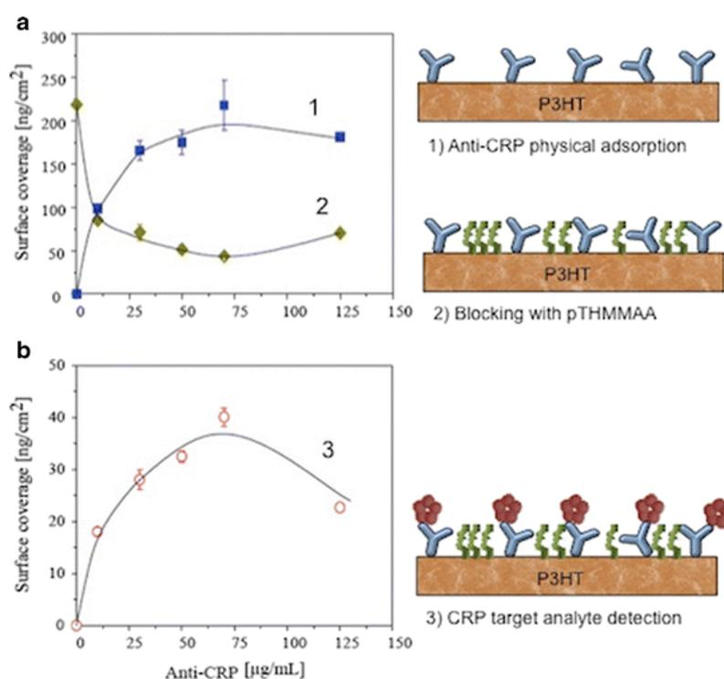
**Figure III.8.** EGOFET to determine the C-reactive protein: SPR measurements of (a) the amount of the antibodies physisorbed on P3HT layer for different anti-CRP concentrations is reported (blue squares) along with the measured quantity of the pTHMMAA polymer adsorbed on P3HT upon binding of the anti-CRP (green diamonds). (b) Amount of the CRP protein captured by the anti-CRP layer deposited on the P3HT surface at different concentrations <sup>(27)</sup>.
