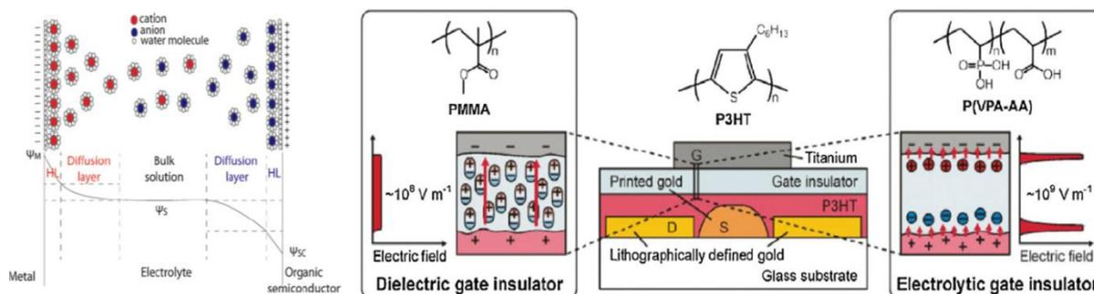
**Figure I.16. Illustration of the compact and diffuse layers corresponding to an OFET and an EGOFET, respectively<sup>(96)</sup>.**
