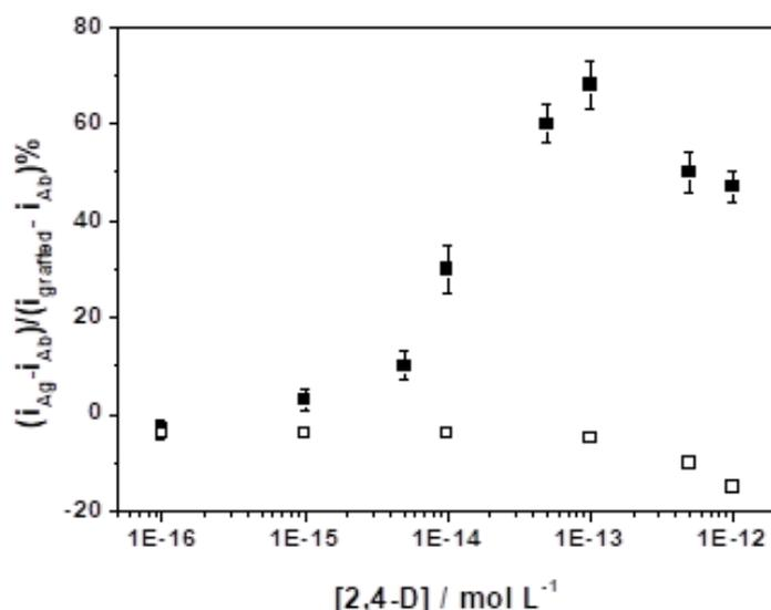
**Figure 8.** as a function of (solid squares) 2,4-D concentration and (open squares) 2,4,5-T. Electrolyte: air-saturated MilliQ water.  $V_{DS} = -0.4$  V,  $V_{GS} = -0.4$  V, for a  $[Ab_{2,4-D}/2,4-D-C_1]$ -modified gate ( $\varnothing 100$   $\mu$ m). Data points show mean values  $\pm$  SD ( $n=4$ ).
