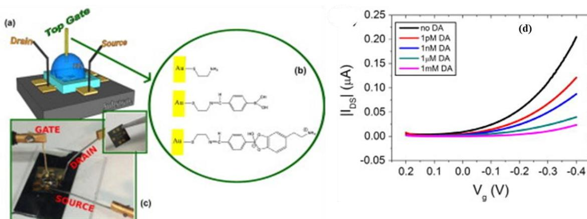
**Figure III.10.** EGOFET for dopamine sensing: (a) Scheme of the EGOFET device. (b) Gate functionalization with (1) CA, (2) BA and (3) dopamine. (c) Picture of the device. (d) Transfer curves acquired in the linear regime, for various dopamine concentrations <sup>(29)</sup>.
