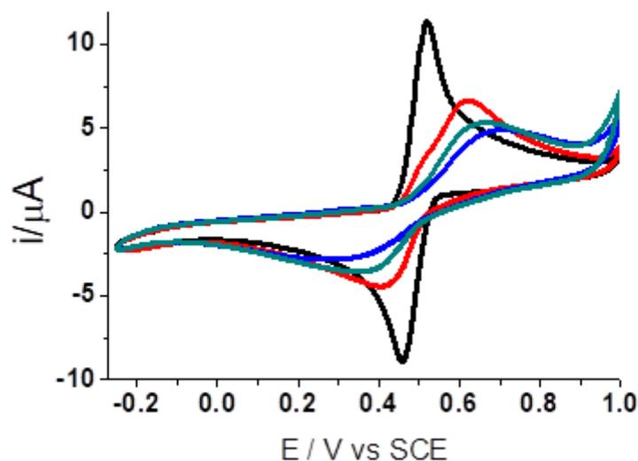
**Figure SI-2b.** Cyclic voltammograms recorded in  $0.1\text{ M H}_2\text{SO}_4 + 10^{-3}\text{ M}$  dopamine with a  $1\text{ mm}$  (black) bare gold electrode; (red) a  $[2,4\text{-D-C}_1]$ -modified electrode; (blue) a  $[\text{Ab}_{2,4\text{-D}}/2,4\text{-D-C}_1]$ -modified electrode and (green) after addition of 2,4-D.
