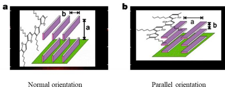
**Figure I.19. Lamellar structure of P3HT, normal or parallel to the substrate, respectively <sup>(133)</sup>.**
