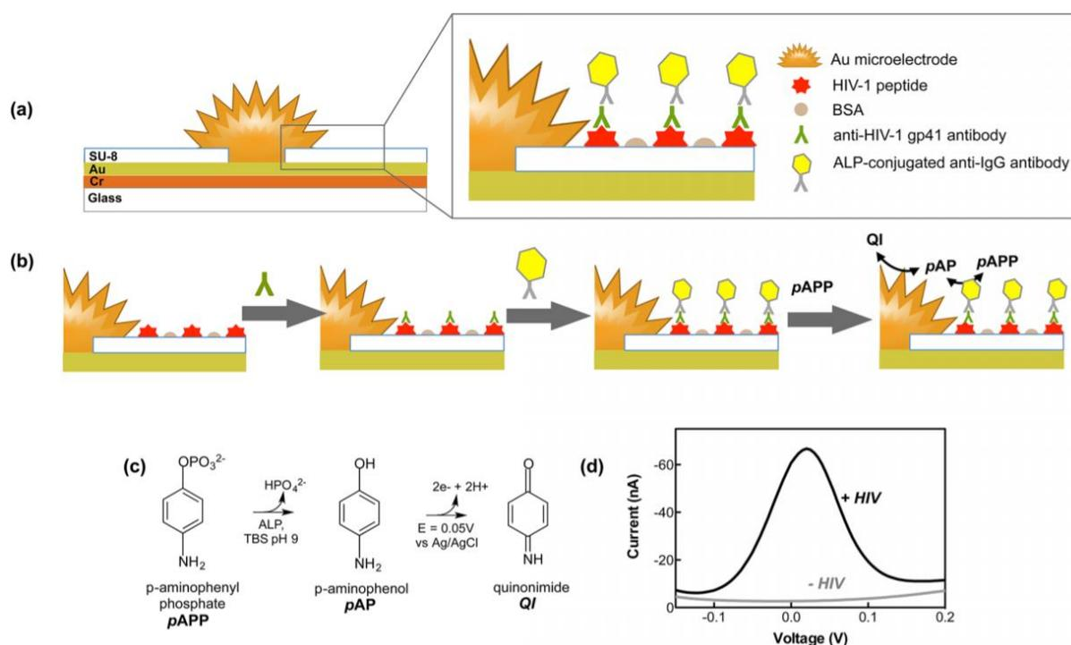
**Figure I.11. Illustration of antibodies detection of HIV. (a) Au microelectrodes (b) Immunorecognition (c) Transduction (d) Resulting DPV <sup>(41)</sup>.**
