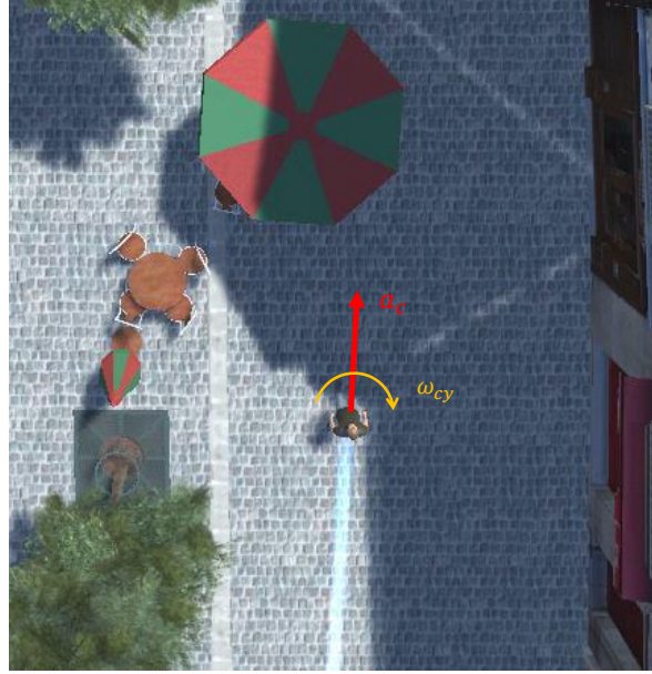
Figure 2.3 – Agent’s control variables. The output of the navigation algorithm updates the acceleration and the turning rate.
