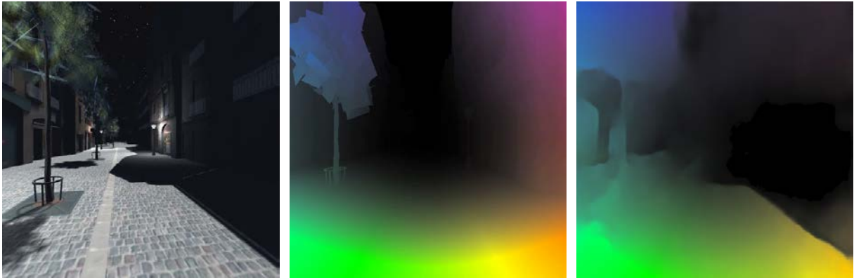
Figure 2.6 – Comparison between synthetic and numeric optical flow. (left) Color image, (middle) synthetic optical flow, (right) numerical optical flow using FlowNet2.0 [IMS + 17].
