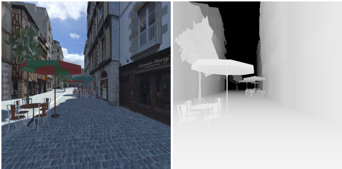
Figure 2.7 – Illustration of depth perception. (left) Color image. (right) Depth map in a grey scale representation.
