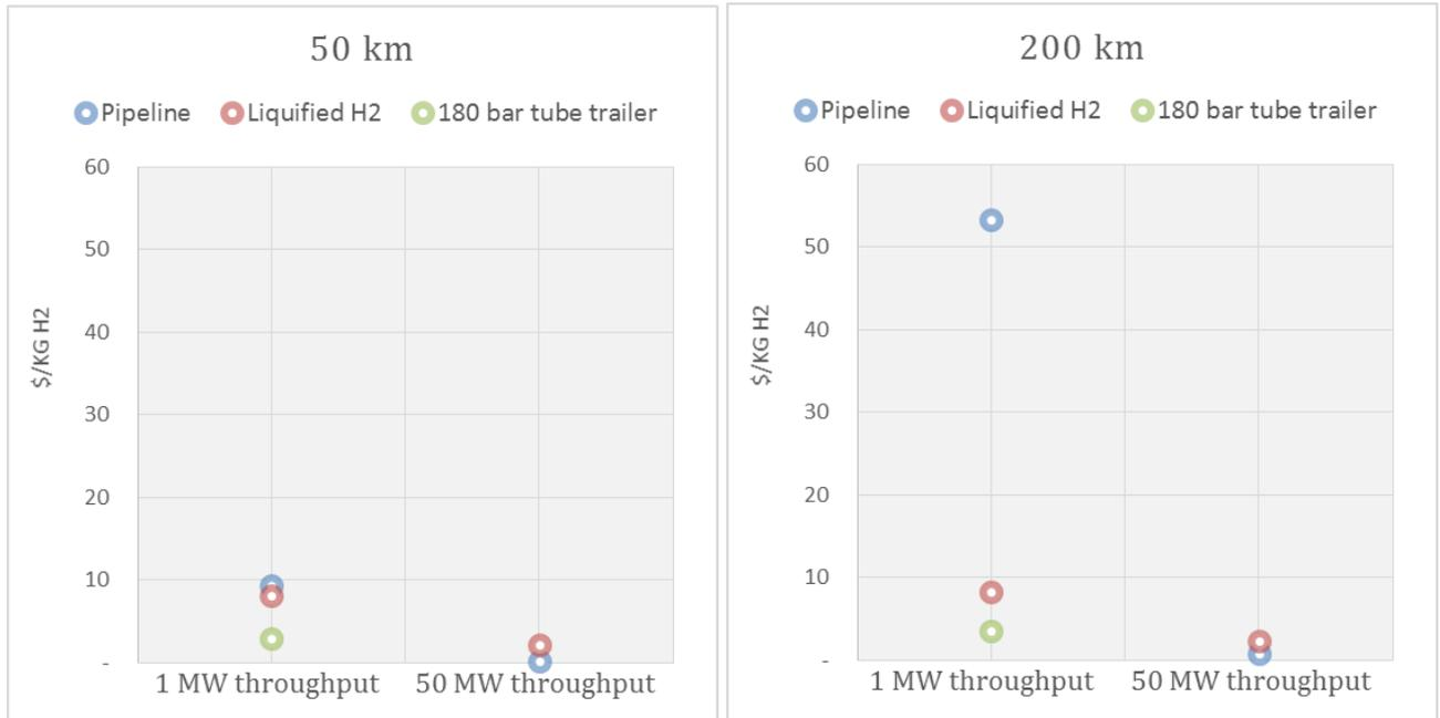
**Figure 29: Hydrogen transport pathways comparison (adapted from [14])**
