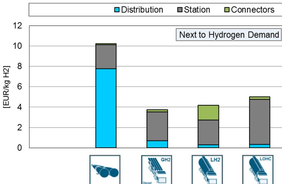
**Figure 81: Hydrogen delivery cost (scenario 5% market penetration)**
