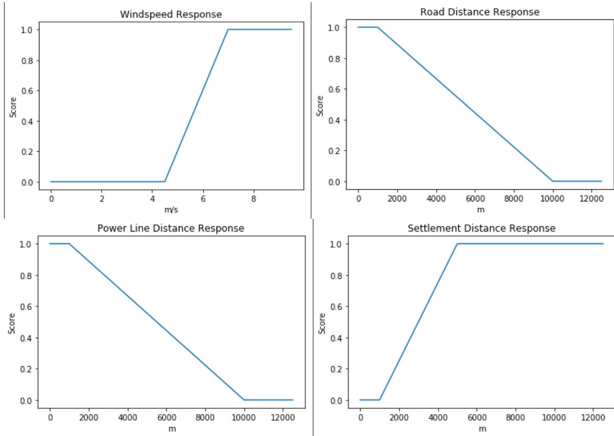
Figure 47: Wind criteria scoring functions
