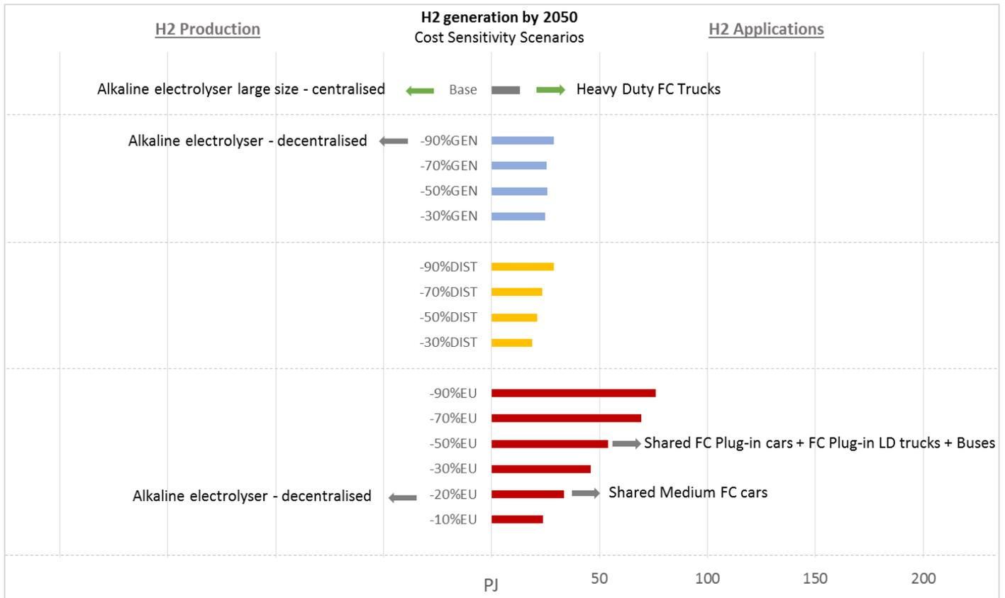
**Figure 38: Resulting hydrogen production volumes by cost reduction scenario (2050) - (arrows indicate production and end use technologies emerging in the results besides the ones appearing in the base scenario)**
