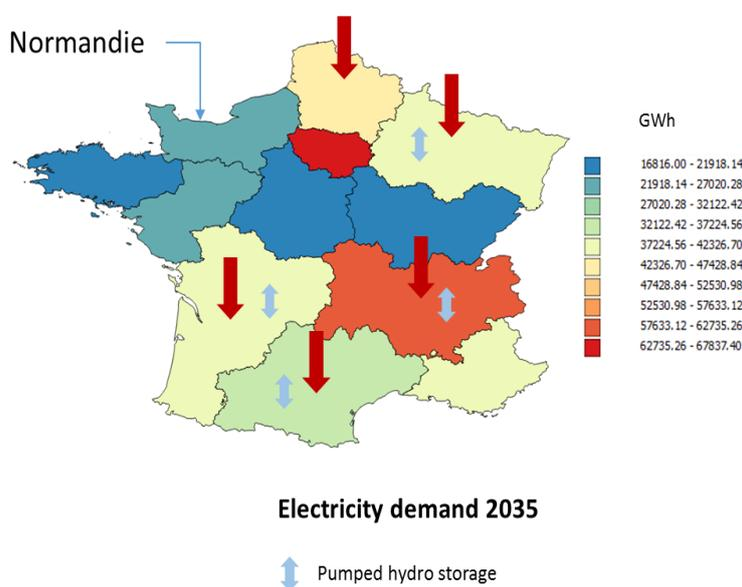
**Figure 60: Electricity demand distribution by region (blue arrows show the locations of pumped hydro storage facilities; red arrows point to the five regions with the highest installed power generation capacities).**
