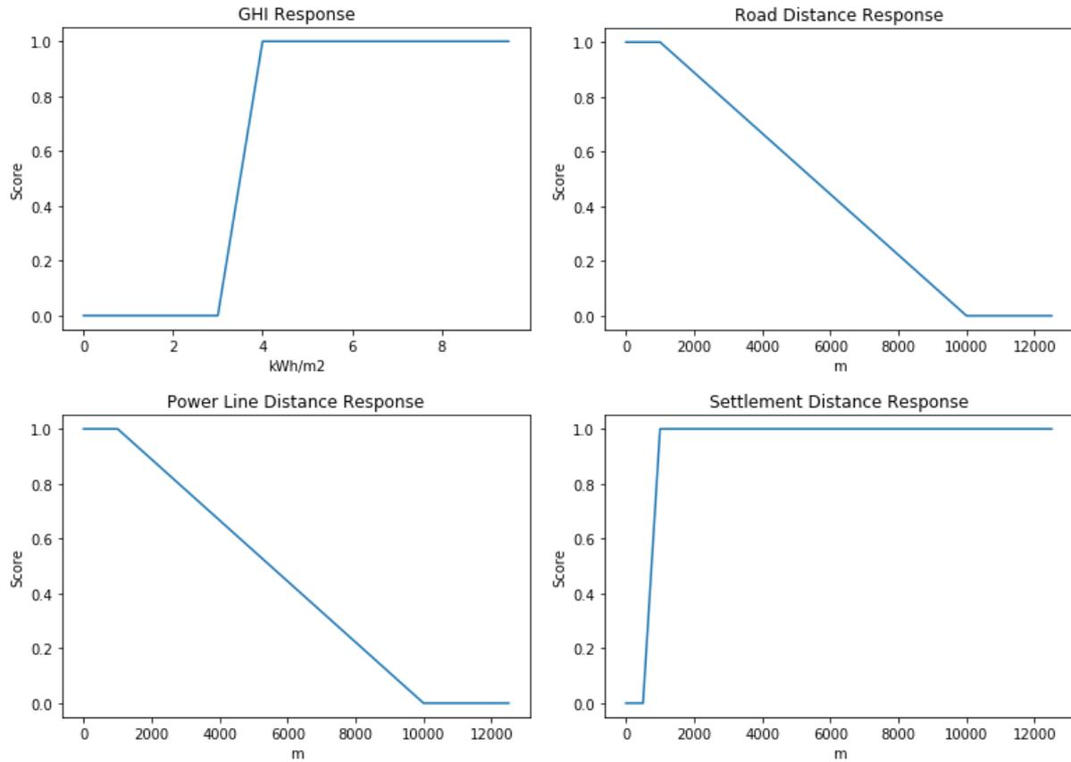
**Figure 48: PV criteria scoring functions**
