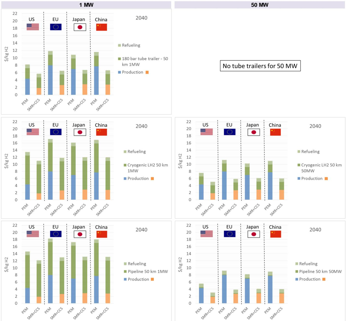
**Figure 32: Hydrogen cost at the pump for the centralized case study in 2040 (left column 1 MW, right column 50 MW of throughput capacity, each line corresponds to a delivery pathway)**
