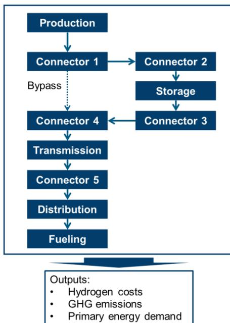
Figure 73: Supply chain setup used in this study
