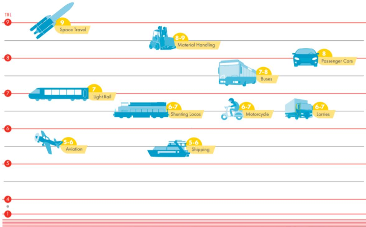
Figure 2: Technology Readiness Level of hydrogen mobility applications [20]
