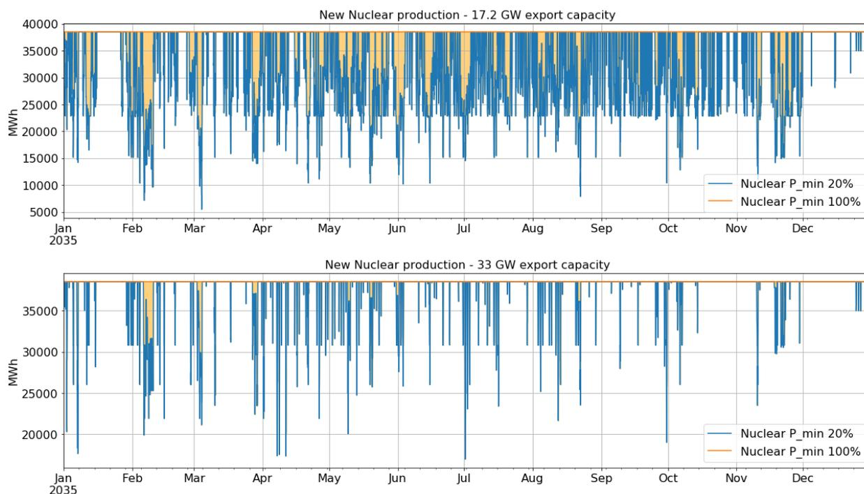
**Figure 67: Nuclear generation profile and available energy for the two alternatives of export capacity. The upper figure corresponds to the 17.2 GW export capacity case study and the lower figure to 33 GW one**
