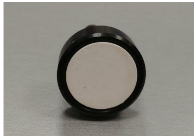
Figure 3.4 White reference used for calibration.
