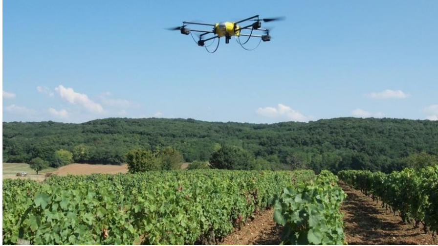
Figure 1.1 UAV equipped with a camera for grapevine disease detection.
