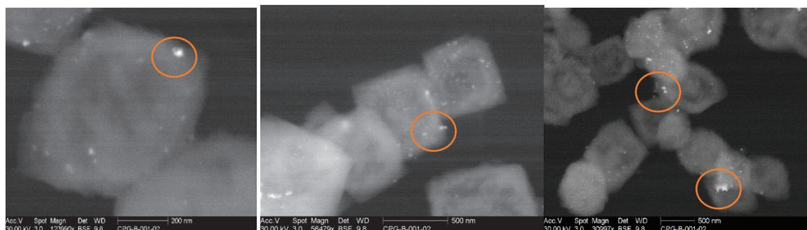
Figure 34 – SEM BSE images of Pt@Hollow $\beta$  prepared following pathway D.
