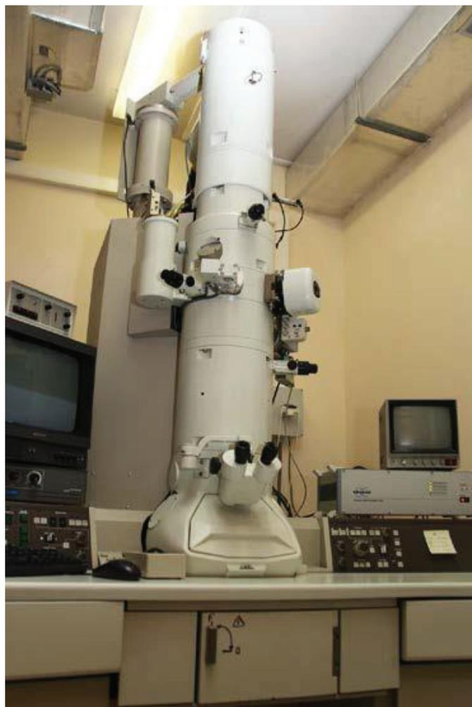
Figure 8 - Picture of JEOL 2010 TEM apparatus.
