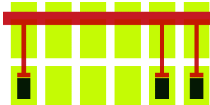
Figure 4. 20 Layout of the control gate and sensing gate of BEOL integrated sensors (red: control gate, black: sensing area)
