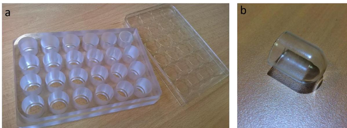
**Figure 64.** First version of the sample rack developed. a: sample rack with the standard COSTAR® cover. b: example of a truncated test tube in sodocalcic glass.
