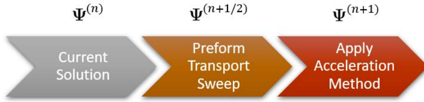
Figure 2.16 – The typical accelerated iterative scheme.
