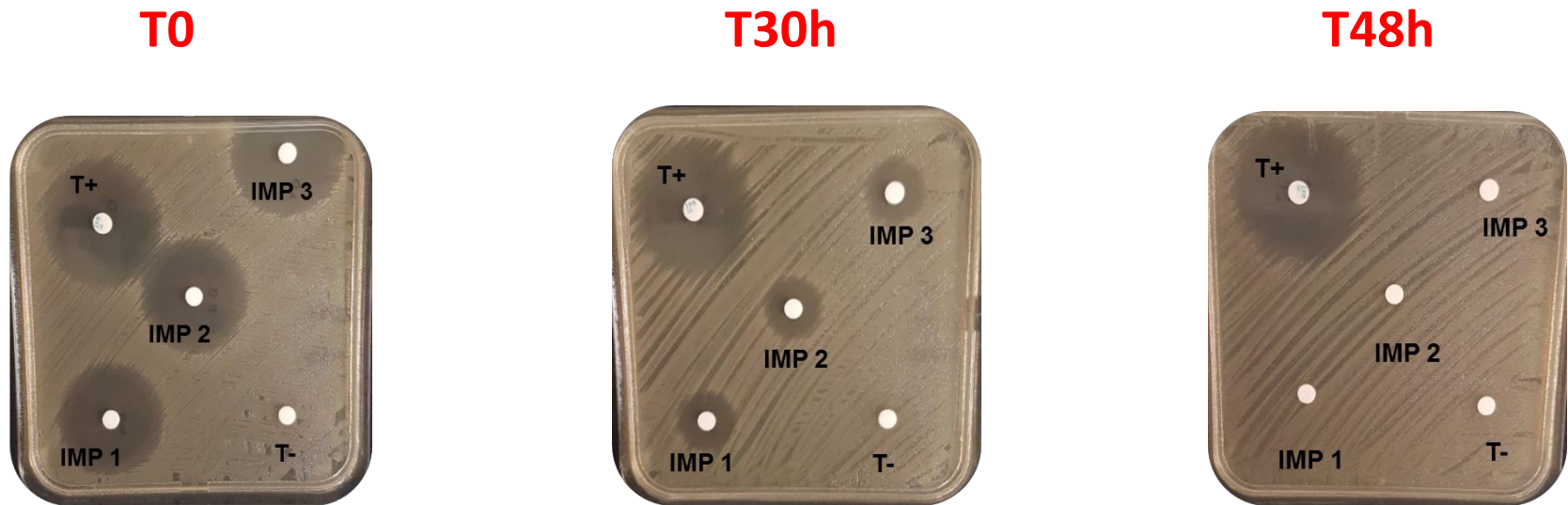
Figure 4: Pictures of the agar diffusion tests performed in triplicate (IMP1, IMP2 and IMP3) with imipenem solution at 10\mu\text{g/ml} stored at 26^\circ\text{C} for different lengths of time ( T=0\text{h} , T=30\text{h} and T=48\text{h} ). The negative (T-) and positive (T+) controls consisted in paper discs impregnated with saline and commercial imipenem disks ( 10\mu\text{g} ).
