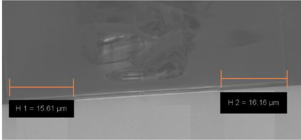
Figure 37: SEM image of a 70 μm wide waveguide. After oxidation at 410 °C for 1h, it was left in contact with air for 1 month. Severe surface delamination is present in the unoxidised central zone.
