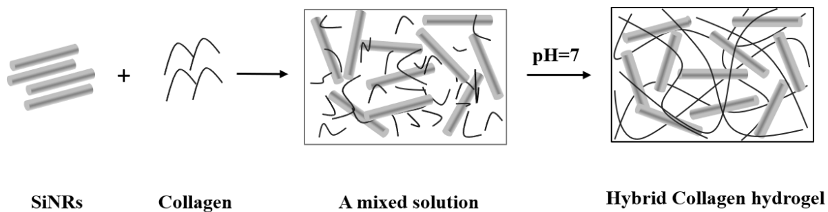
Figure 4-10 Schematic illustration of the preparation of SiNRs-collagen hydrogels
