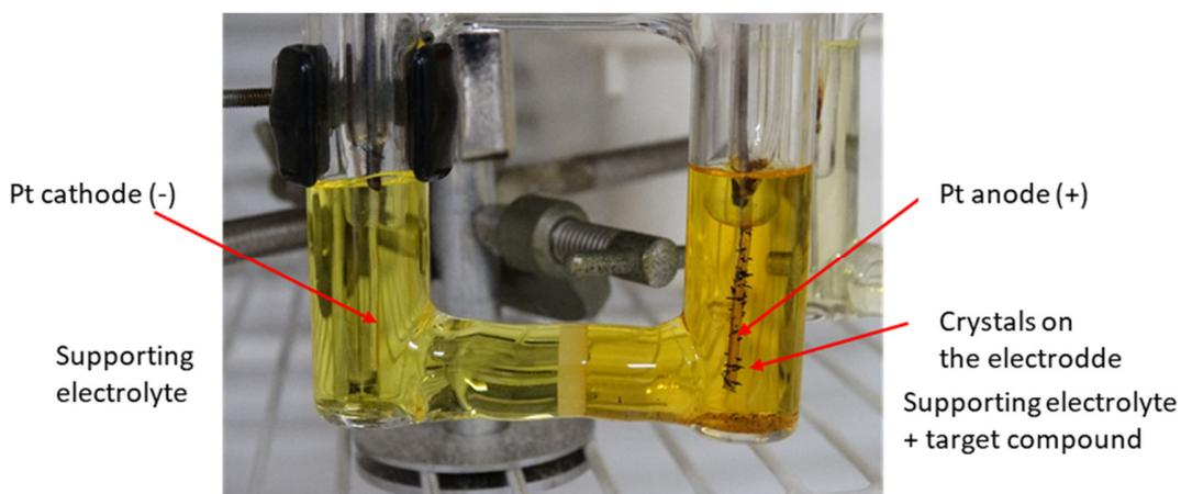
Experiment is conducted using the standard U-shaped electrochemical cell, with compartments separated with a glass filter in order to prevent mixing and contamination while maintaining conductivity. On order to prevent impurities, cell is washed with a H<sub>2</sub>SO<sub>4</sub>/H<sub>2</sub>O<sub>2</sub> mixture, followed by methanol, water, acetone and drying in the oven.
