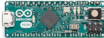
Figure 4.11: Arduino Micro Board.
