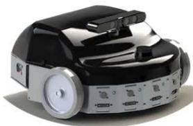
Figure 4.3: Minilab Enova Robot.
