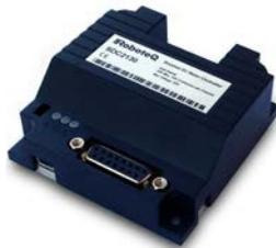
Figure 4.10: Roboteq SDC2130 controller.
