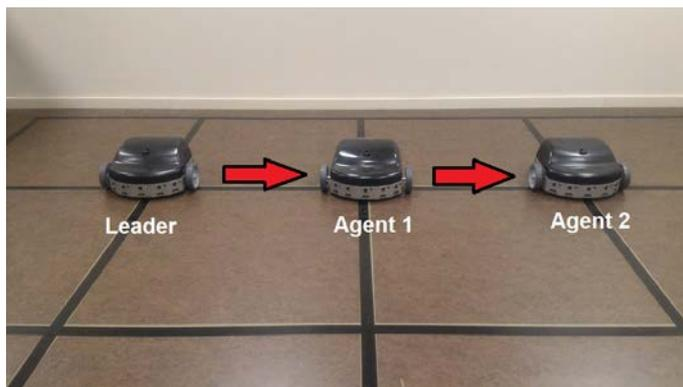
Figure 5.2: Topology of MAS using using our Minilab Enova robot platform.
