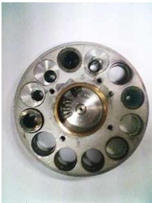
Figure 1-4: Picture of the wheel cones of the source HICONEX 384
