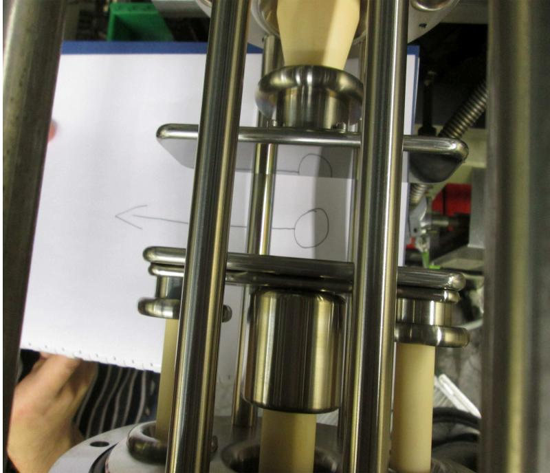
*Figure 1-11: Electrostatic deflector plates; the arrow shows the direction of the beam*
