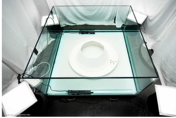
Figure 3.1: Experimental set-up. The ring-shaped tank is built from two walls, an outer wall of radius 35 cm and a conic inner wall with an average radius of 21 cm at the water level creating a corridor of 14 cm width. Photograph shot by David Villa, ScienceImage CBI CNRS, Toulouse, France.
