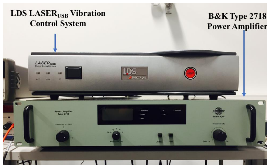
Figure 2-7 Picture of the vibration control system and the power amplifier
