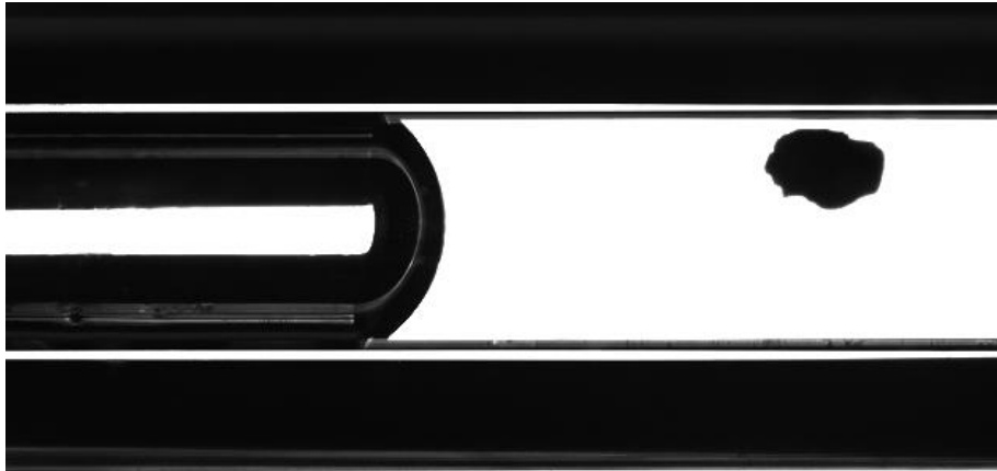
Figure 2-14 Picture of capillary tube marked by a paint drop
