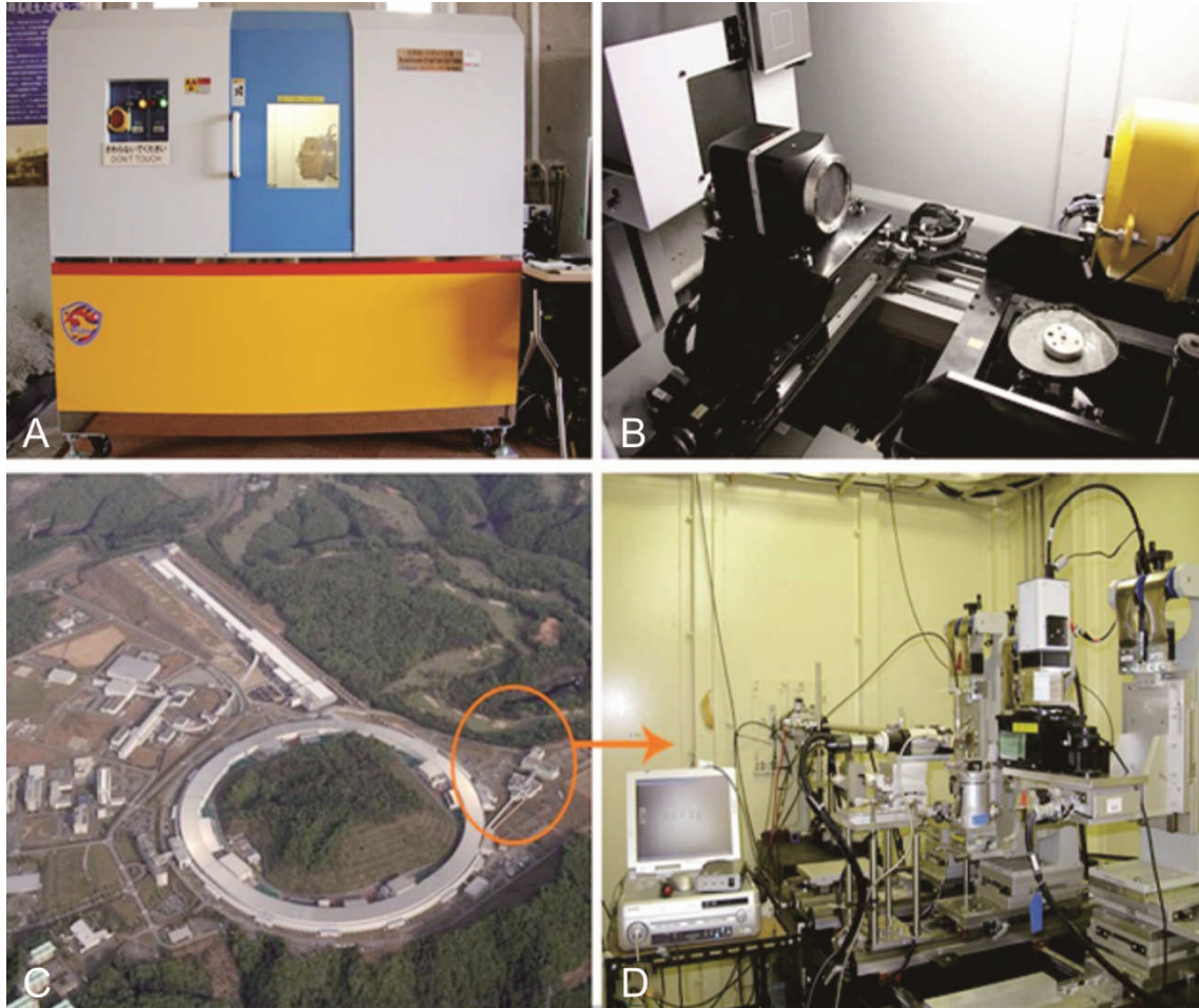
Fig. 68. A-B. The computed X-ray Microtomography (XTM) at Tohoku University, Japan. C-D. The synchrotron X-ray Microtomography (SRXTM) at Spring-8 in Hyogo, Japan.
