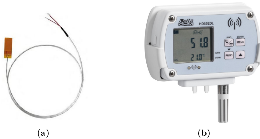
Figure 3.12: Instrumentation changes for the SCV2 showing (a) surface temperature sensors and (b) the Delta Ohm wireless acquisition modules.
