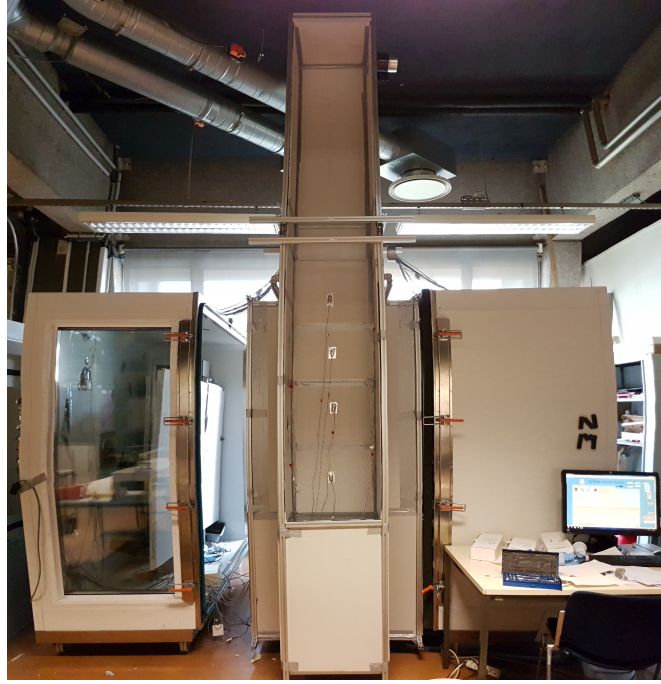
Figure 3.5: First solar chimney laboratory prototype developed at ENTPE
