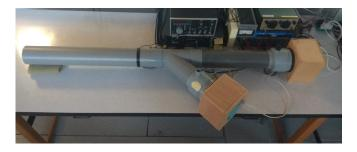
Fig. 1. Duct active noise control test-bench (Photo).
