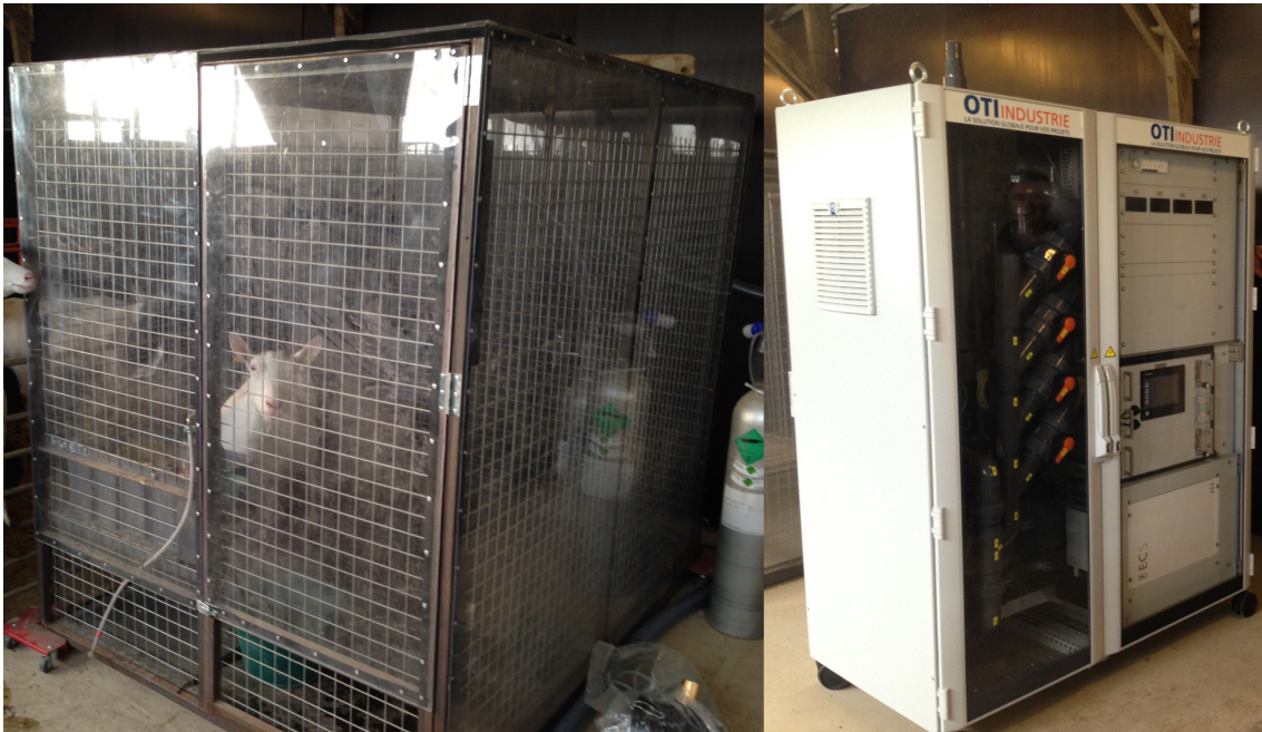
Figure 10.4: Phenobox prototype to measure ingestion kinetics and methane production. This device was designed and implemented by a MoSAR discussion group.
