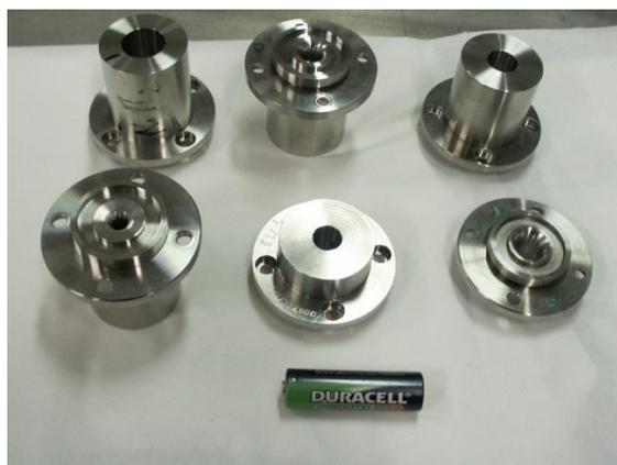
*Figure 2.10 Laval nozzles from the mini CRESU setup of Bordeaux*
