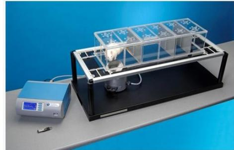
Figure 34: Electronic Von Frey aesthesiometer apparatus with the grid and plastic boxes
