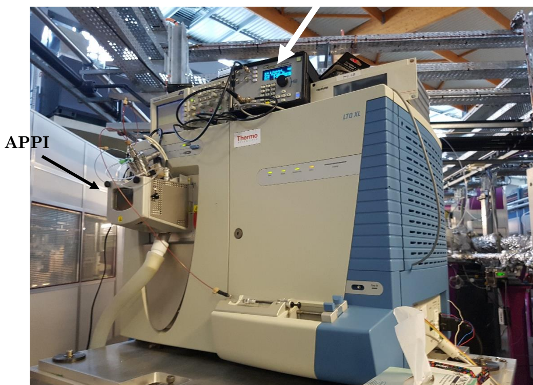
Figure 2-13 Photograph of the LTQ ion trap setup at DESIRS/SOLEIL. The PAH solution is injected from the needle (bottom right) towards the APPI source. The shutter controller can be seen on top of the instrument.
