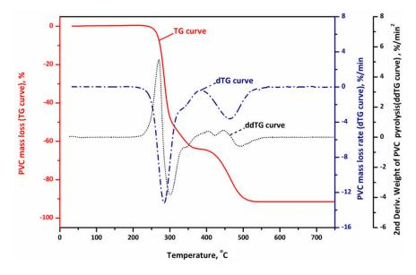
Figure 4. 7 TG, DTG and 2<sup>nd</sup> order DTG curves of PVC pyrolysis under N<sub>2</sub> atmosphere at heating rate of 10 °C/min
