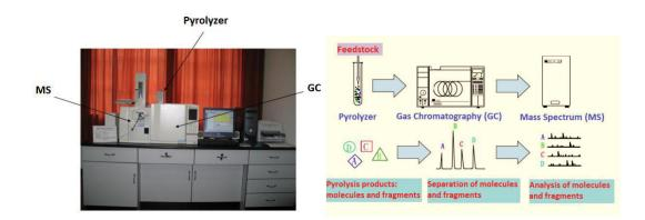
Figure 2. 6 General photograph and schematic diagram of the Py-GC/MS experimental apparatus
