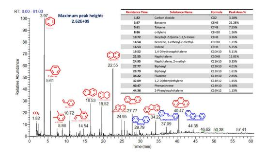
Figure 5. 17 Identified tar composition from PVC pyrolysis at 650 °C with the addition of CaO reactant
