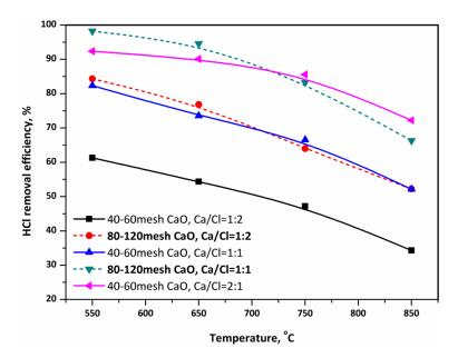
Figure 4. 14 Effect of CaO particle size on HCl mitigation efficiency during PVC pyrolysis with the presence of in-furnace CaO reactant
