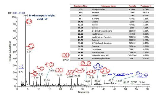
Figure 5. 16 Identified tar composition from PVC pyrolysis at 650  $^{\circ}\mathrm{C}$  in the absence of CaO
