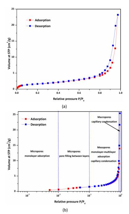
Figure 2. 3 N<sub>2</sub> adsorption-desorption (a) isotherms and (b) Log isotherms of CaO reactant with particle size of 0.25 - 0.43 mm (40-60 mesh)
