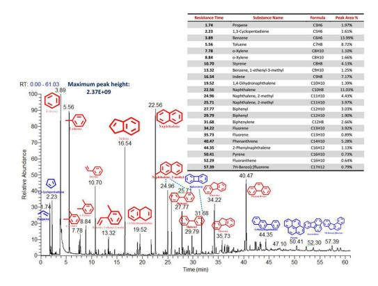
Figure 5. 18 Identified tar composition from PVC pyrolysis at 850 °C in the absence of CaO reactant
