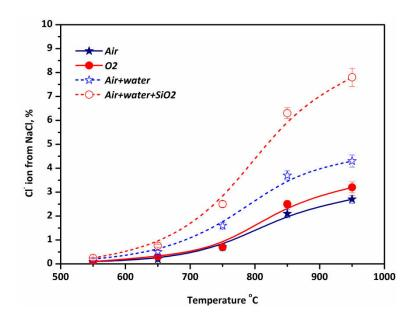
Figure 4. 6 Conversion of Cl<sup>-</sup> ion from NaCl under air atmosphere and O<sub>2</sub> atmosphere and the effect of water and SiO<sub>2</sub>
