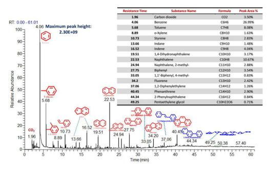
Figure 5. 14 Identified tar composition from PVC pyrolysis at 550 °C in the absence of CaO
