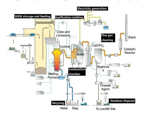
Figure 7. 5 Schematic diagram of the considered gasification-melting system, data obtained from the work of Tanigaki et al. [33]
