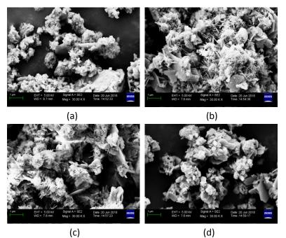
Figure 3. 12 Formation of the product-layer at temperature of 850 °C: a,  $t/t_f$ = 0.1; b,  $t/t_f$ = 0.3; c,  $t/t_f$ = 0.5; d,  $t/t_f$ = 1
