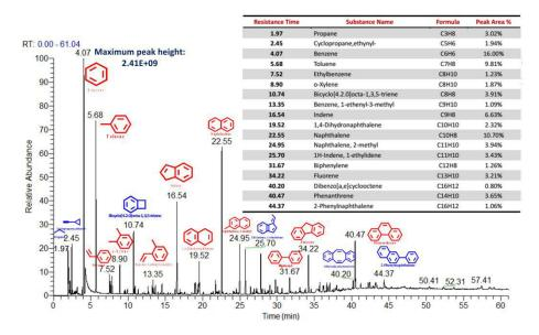
Figure 5. 9 Identified tar composition from PVC pyrolysis at 750 °C in the absence of CaO
