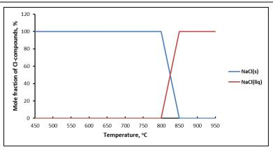
Figure 4. 2 Thermodynamic simulation results of pure NaCl under N<sub>2</sub> atmosphere
