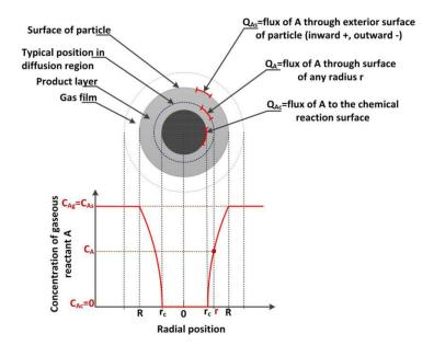
Figure 3. 3 Concentration of HCl gas under the condition that the reaction is only limited by internal diffusion of HCl through the product-layer (A refers to HCl gas)
