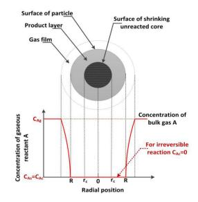
Figure 3. 2 Concentration of HCl under the condition that the reaction is only limited by gas film diffusion (A refers to HCl gas)
