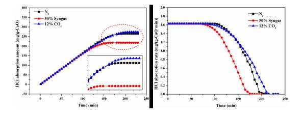
Figure 3. 15 Effect of gas composition on total HCl mitigation amount and HCl mitigation rate by CaO reactant
