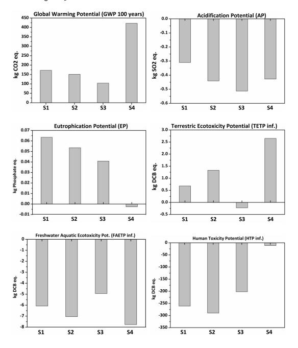
Figure 7. 6 Characterized environmental impacts of different systems: S1, Incineration system; S2, Pyrolysis system; S3, Gasification system; and S4, Gasification-melting system
