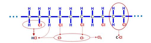
Figure 5. 11 Chlorine-content compounds formation from PVC pyrolysis, data derived from Ruizhi ZHANG [22]
