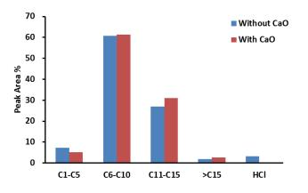
Figure 5. 12 Distributions of detected species of pyrolytic tar derived from PVC pyrolysis at 750 °C as a function of carbon atom numbers
