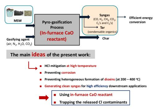
Figure 1. 5 The main ideas of this study: investigate in-furnace capture of chlorine to avoid the release of HCl by using in-situ CaO reactant
