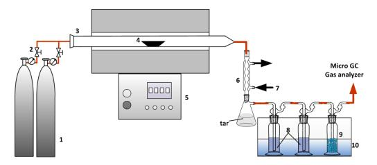
Figure 2. 5 Schematic diagram of the experimental fixed bed tubular furnace apparatus. 1, gas source; 2, gas flowmeter; 3, quartz tubular furnace; 4, quartz boat; 5, electric heater and temperature controller; 6, condenser for tar collection; 7, cooling water; 8, HCl mitigation solution (0.1 mol/L NaOH); 9, silica gel; 10, ice-water bath
