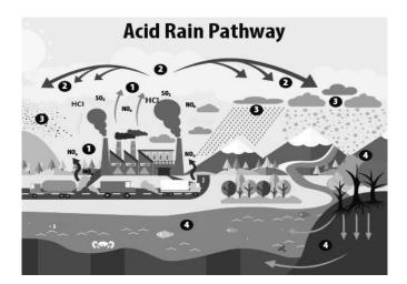
Figure 1. 6 Graphic principle of acid rain formation pathway: (1) Emissions of SO<sub>2</sub>, NO<sub>x</sub> and HCl are released into the air, where (2) the pollutants are transformed into acid particles that may be transported in a long distance, (3) the acid particles then fell to the earth as wet and dry deposition (dust, rain, snow, or etc.) and (4) may cause harmful effects on soil, forests and water, data obtained from [42]
