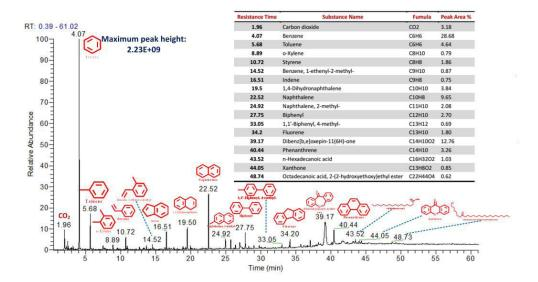
Figure 5. 15 Identified tar composition from PVC pyrolysis at 550 °C with the addition of CaO reactant
