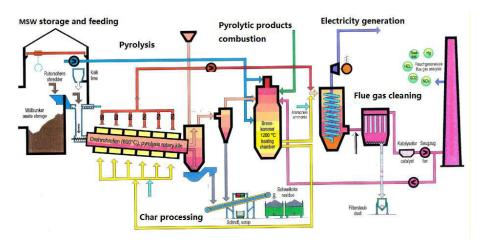
Figure 7. 3 Schematic diagram of the considered pyrolysis system, data obtained from the report of DGEngineering [29]
