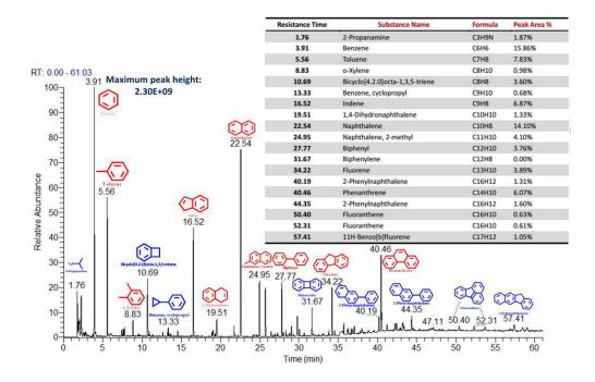
Figure 5. 19 Identified tar composition from PVC pyrolysis at 850 °C with the addition of CaO reactant
