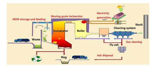
Figure 7. 2 Schematic diagram of the considered incineration system
