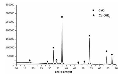
Figure 2. 2 XRD analysis of CaO reactant
