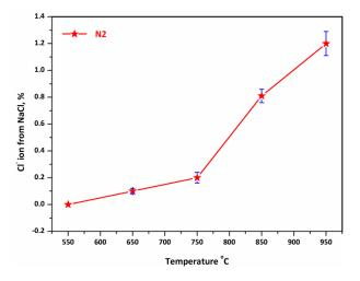
Figure 4. 5 Conversion of Cl<sup>-</sup> ion from NaCl under N<sub>2</sub> atmosphere
