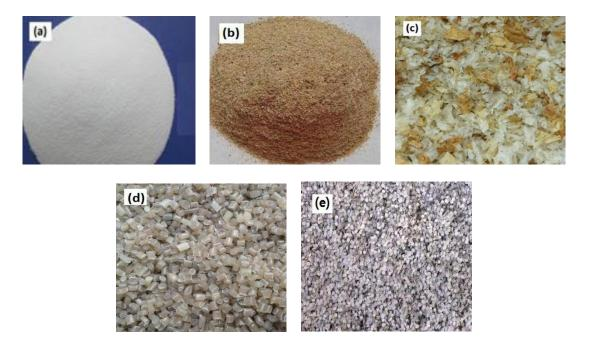
Figure 2. 1 Pictures of MSW components: (a), PVC pellet; (b), wood; (c), food waste; (d), PE pellet; and (e), paper
