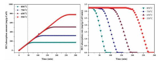
Figure 3. 7 The total HCl mitigation amount and mitigation rate with time under different reaction temperature
