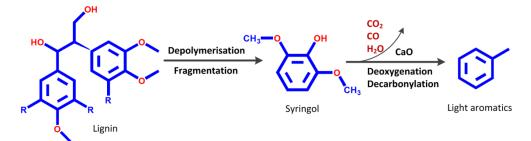
Figure 5. 6 Representative lignin pyrolysis, decarboxylation and decarbonylation of pyrolytic tar over CaO reactant
