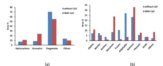
Figure 5. 7 Composition of pyrolytic tar derived from food waste pyrolysis at 750 °C without/with the addition of CaO reactant (others represent mainly nitrogen-content compounds)
