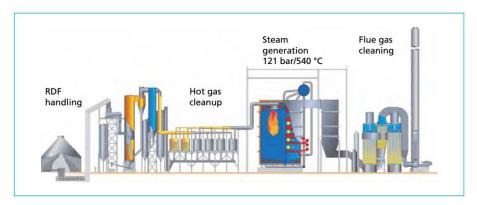
Figure 7. 4 Schematic diagram of the considered gasification system, data obtained from the work of Bolhàr-Nordenkampf et al. [30]
