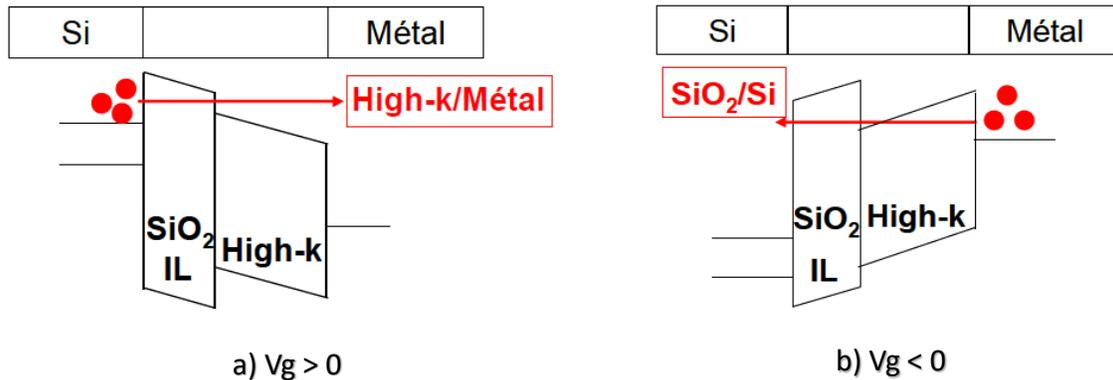
Figure 1.40: HKMG stack band diagrams in the case of the (a) injection regime from the substrate and (b) injection from the metal gate [115]
