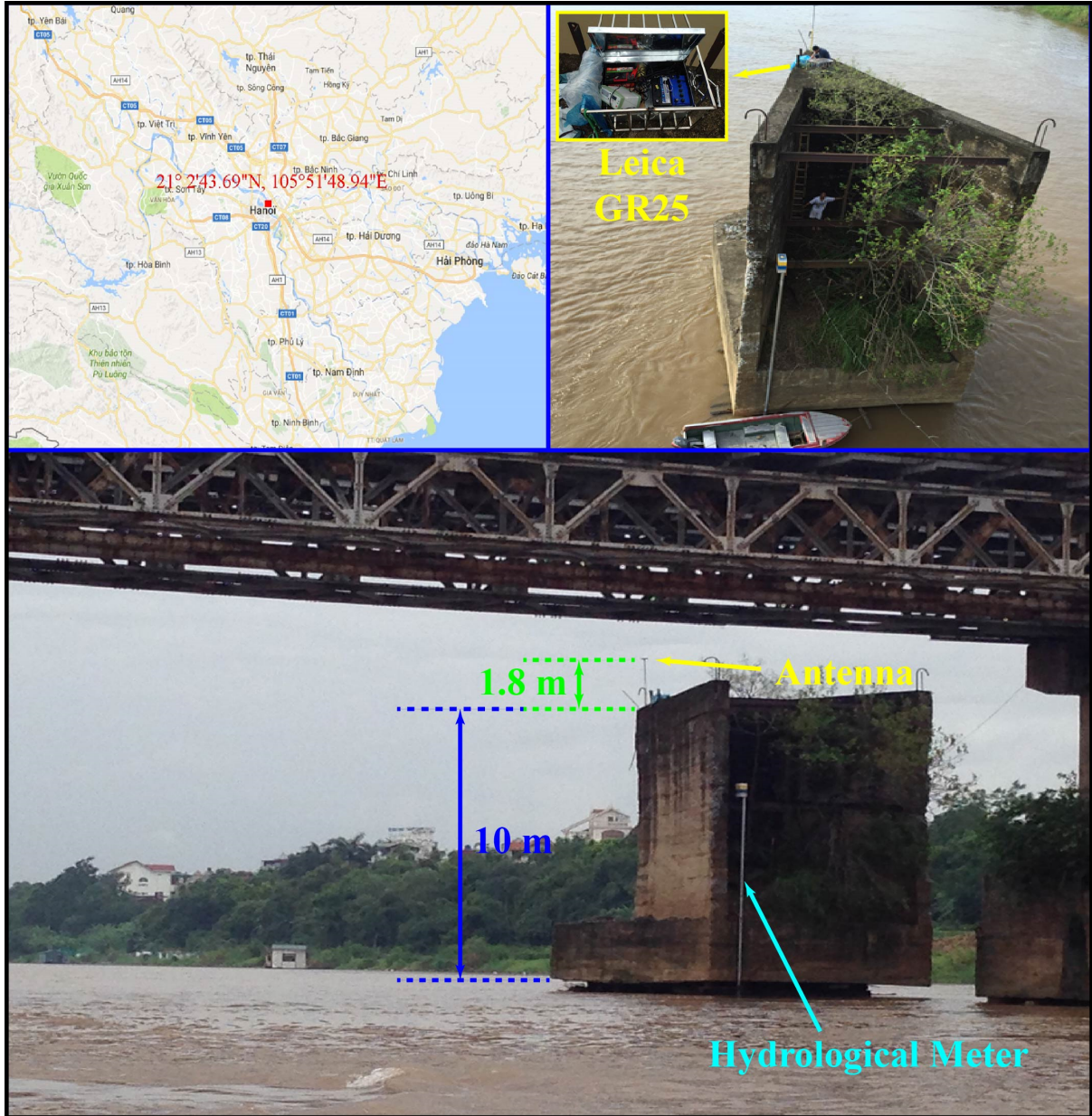
Figure IV.15 – The GNSS receiver with a single antenna installed on the top of the old bridge abutment ( 21^{\circ}2'44.04''N, 105^{\circ}51'48.86''E ) on the Red river in Hanoi, Vietnam from the 27 th July to 12 th August 2016. (Ha, 2018)
