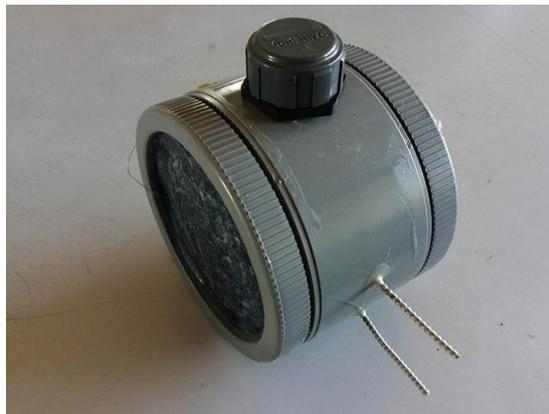
*Fig. 2.15: Photo of a lab-scale WWMFC*
