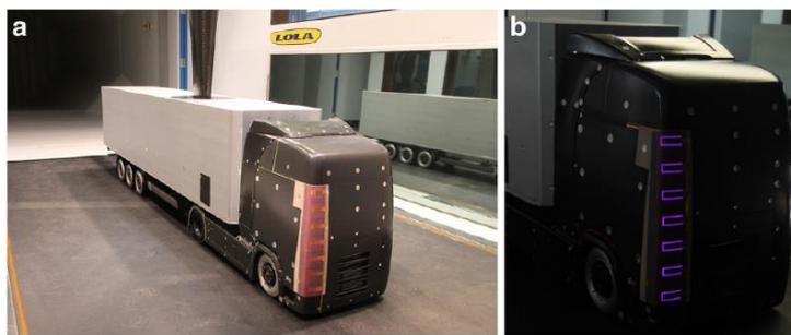
Figure I.41: (a) Picture of the reduced scale truck mockup with the unactive DBD actuators, (b) Focus on the A-pillar with the active DBD actuators.
