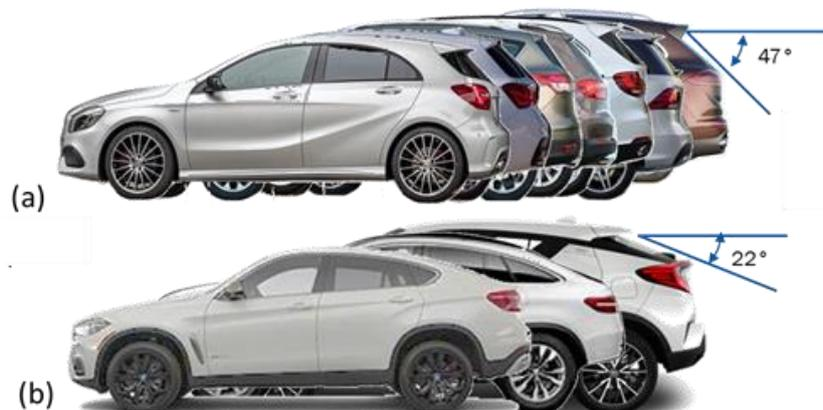
Figure I.7:(a) Hatchback versions of the SUV with a rear window inclined at  $45^\circ$ ; (b) New SUVs with a rear window inclined at  $22^\circ$ ;
