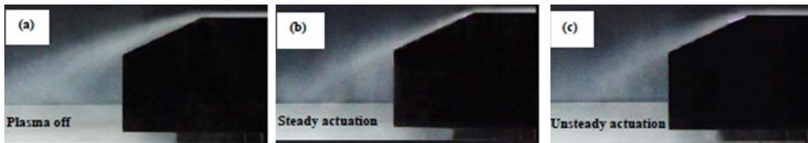
Figure I.40: Pattern of the flow passing through the 25° Ahmed Body behind the model at 10m/s: (a) Baseline wake flow; (b) Steady plasma actuation leading to a drag reduction of 7.3%; (c) Unsteady plasma actuation leading to a drag reduction of 4.88% (Shadmani et al., 2018).
