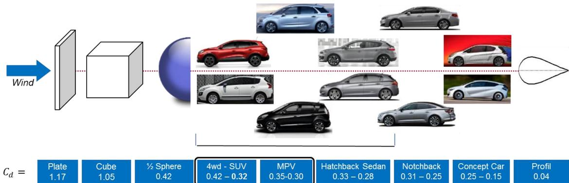
Figure I.5: Drag coefficient measured for different obstacle from the flat plate with high drag coefficient to the profiled body with an optimal drag coefficient.
