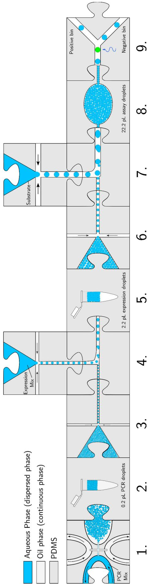
FIGURE 3.6: In vitro microfluidic workflow 2
