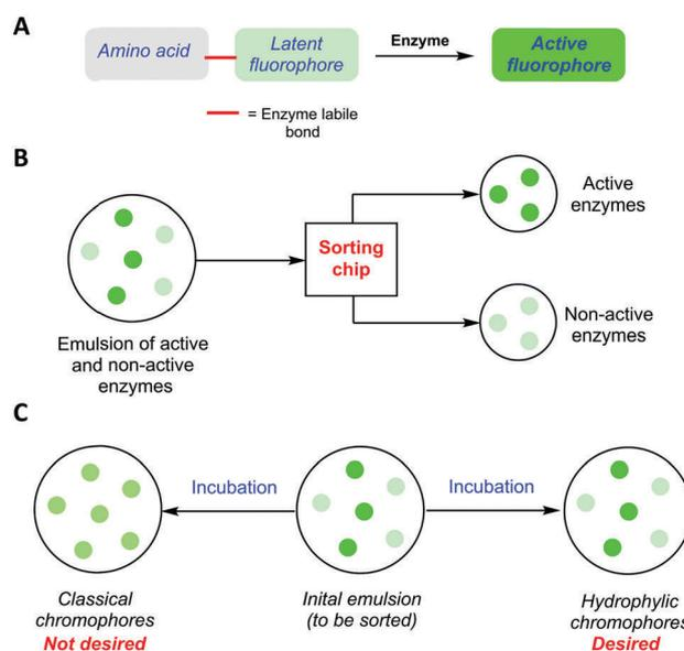
**Fig. 1** Fluorescence based enzymatic assay in droplets: (A) typical fluorogenic enzymatic substrate used for these assays. (B) Fluorescence based sorting device. (C) Evolution of droplet fluorescence over time during incubation.
