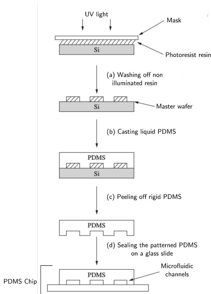
FIGURE 2.2: **Soft-lithography and PDMS chip fabrication.** (a): Soft-lithography process. The master wafer is patterned with resin forming negatives of the microfluidic channels. (b): Liquid PDMS is mixed with curing agent and poured on the master wafer and heated at 70°C for 2 h. (c): Rigid PDMS is peeled off the master wafer. (d): After plasma treatment, the PDMS slab is sealed on a glass slide. Adapted from [92].
