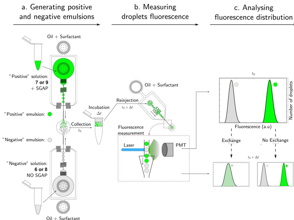
Fig. S2: Workflow of the exchange test experiment in droplets
