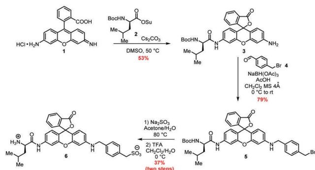
Scheme 3 Synthesis of fluorogenic SGAP substrate **6**.
