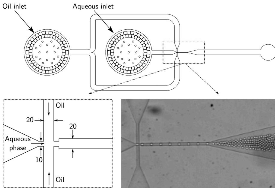
FIGURE 2.5: **2-5 pL droplet maker** All dimensions are in  $\mu\text{m}$ . Channels height is  $10\ \mu\text{m}$ . Pressure settings: aqueous phase: 1100 mBar, oil phase: 1000 mBar.
