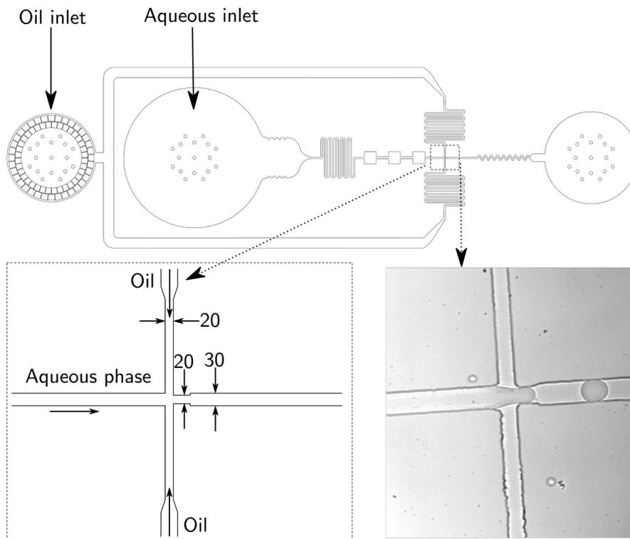
FIGURE 2.6: **20-30 pL droplet maker** All dimensions are in  $\mu\text{m}$ . Channels height is  $20\ \mu\text{m}$ . Pressure settings: aqueous phase: 1100 mBar, oil phase: 1000 mBar.
