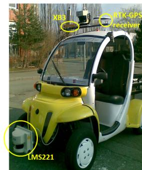
FIGURE 2.5 – Equipped UTBM car.
