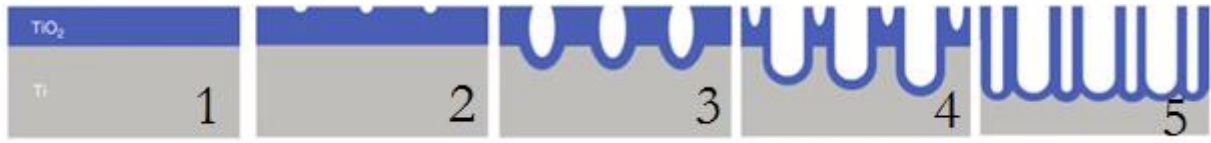
Figure 40: Different steps of the nanotubes growth (from [76]).
