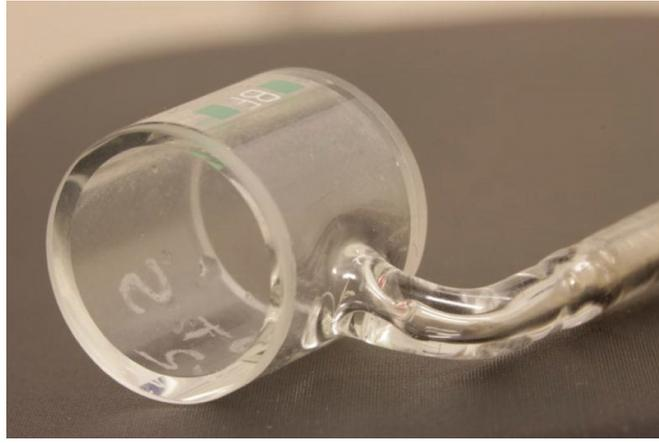
Figure 5.2: Photograph of the OTS-coated cell
