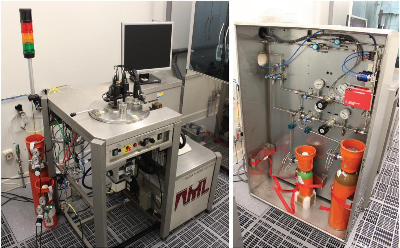
Figure 3.8: Pictures of the AML anodic bonding equipment without gas lines (left) and the dedicated gas lines added thereafter (right).
