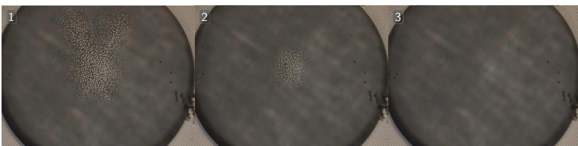
Figure 5.25: Evolution of the condensation in cell T26EE over several hours at 70 °C.
