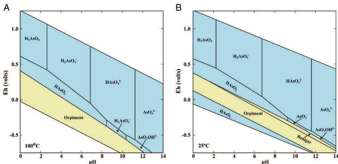
Fig. 7. Eh–pH phase diagrams for the As–S system calculated at  $P = 120$  bars,  $[As] = 900\text{--}1000$   $\mu\text{g/L}$ , and  $[SO_4] = 900\text{--}1900$   $\text{mg/L}$ . (A) stability fields of As fluid speciation and minerals at  $T = 100$  °C; (B) stability fields of As fluid speciation and minerals at  $T = 25$  °C. Yellow fields indicate mineral phases and blue fields indicate dissolved species.
