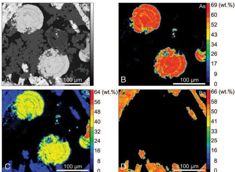
**Fig. 6.** BSE image and X-ray maps of cross-cut fungal elements among barite crystals (sample #MN-DR-1-11; polished section): (A) BSE image; (B) X-ray scan in As L<sub>α</sub>; (C) X-ray scan in S K<sub>α</sub>; (D) X-ray scan in Ba L<sub>α</sub>. Color scales (right-hand side), elemental concentrations.
