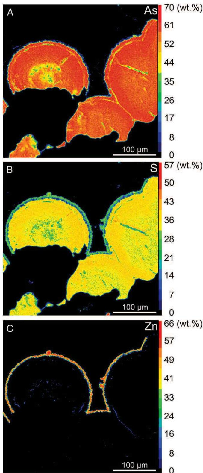
**Fig. 4.** X-ray maps of colloform orpiment (sample #SO-133 25GTVA-7; polished section): (A) X-ray scan in As  $L_{\alpha}$ ; (B) X-ray scan in S  $K_{\alpha}$ ; (C) X-ray scan in Zn  $K_{\alpha}$ . Color scales (right-hand side), elemental concentrations.
