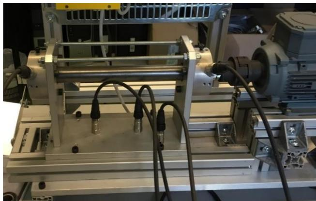
**Figure 4.3 The bench containing the rotating motor with bearing**
