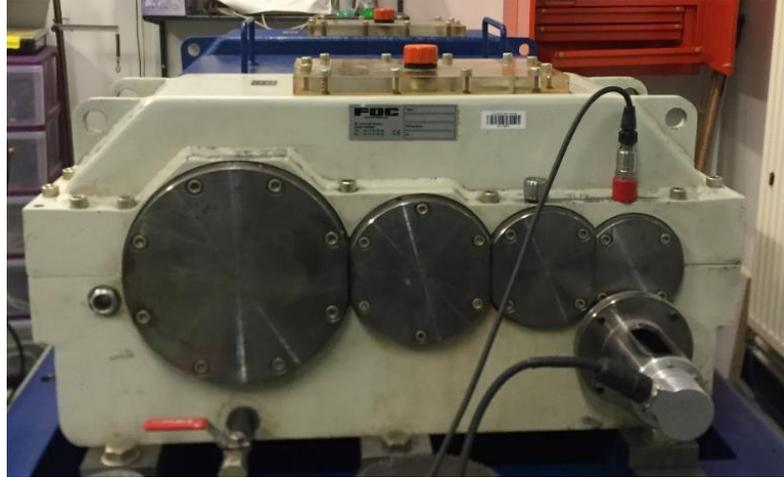
Figure 4.24 Gear test bench with an accelerometer directly above the gear under test
