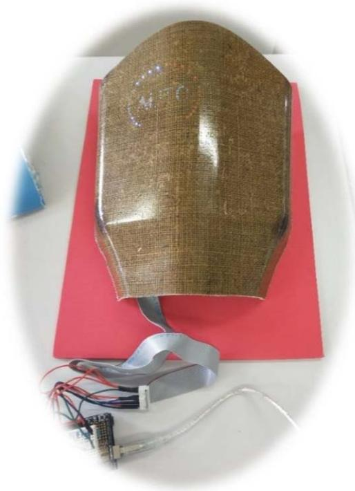
Fig 2-8 Smart composite monocoque of car
