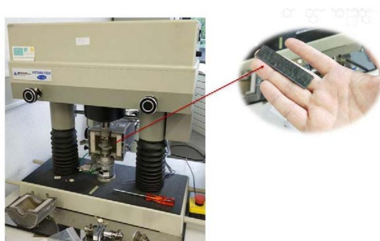
Fig 4-24 Experimental setup and a test sample for DMA
