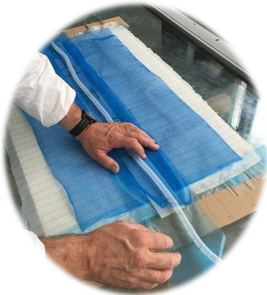
Fig A-5 Arrangement of the drainage materials
