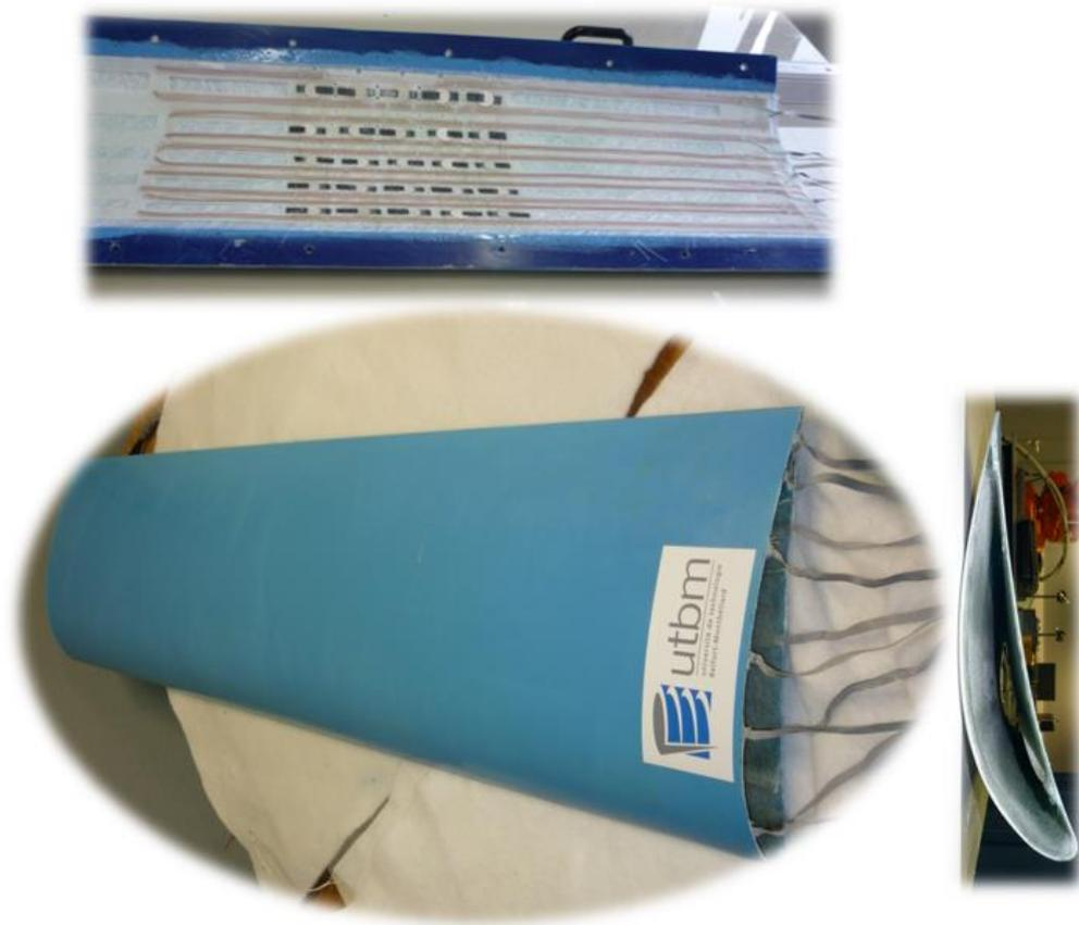
Fig 2-5 Smart composite wing
