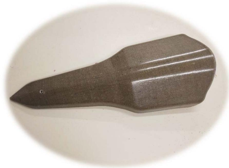
Fig 2-6 Smart composite bargeboard of racing car
