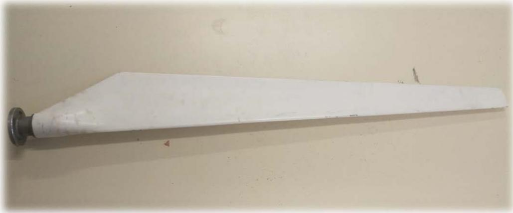
Fig 2-10 Smart composite blade of wind turbine
