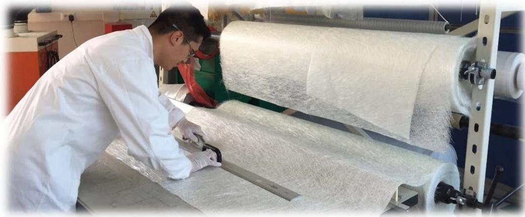
Fig A-3 Cutting of the mat of glass fiber
