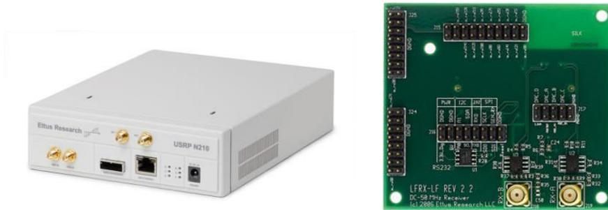
Figure 4.1 USRP N210 SDR box (left) and LFRX daughterboard (right)
