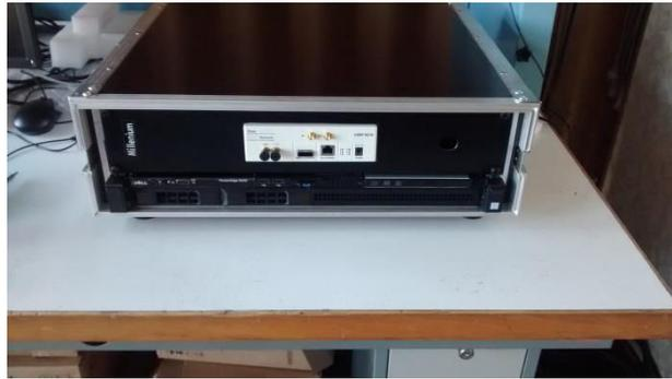
Figure 4.6 Server and USRP N210 module placed within the box
