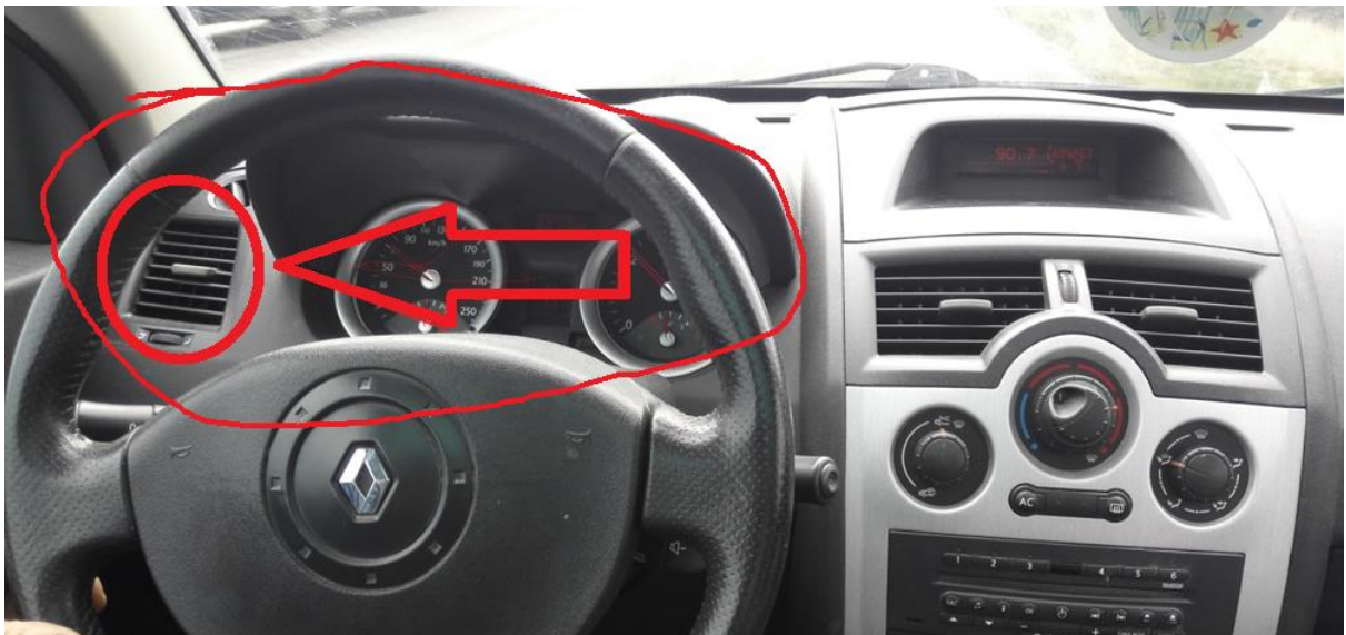
Figure 112: Renault Megane dashboard and the considered left air diffuser for the parametric variation of the angle of the guiding vanes
