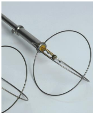
Figure 55: Hot film velocity probes used in this study: a) TSI Thermo-anemometer Straight Probe 960 and 9565 data logger, b) Dantec omnidirectional probe
