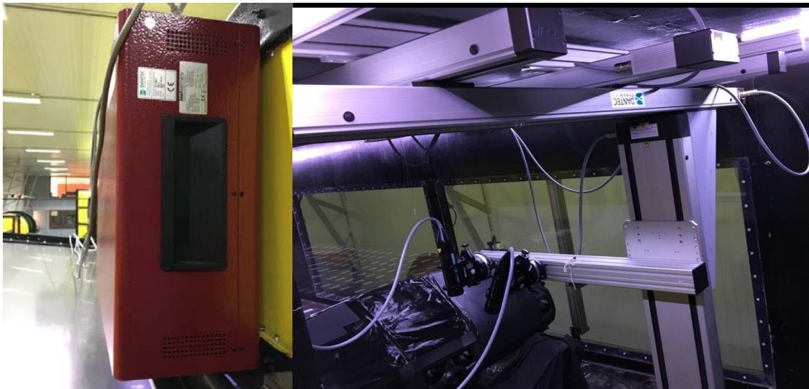
Figure 62: 3D traverse system used in this study
