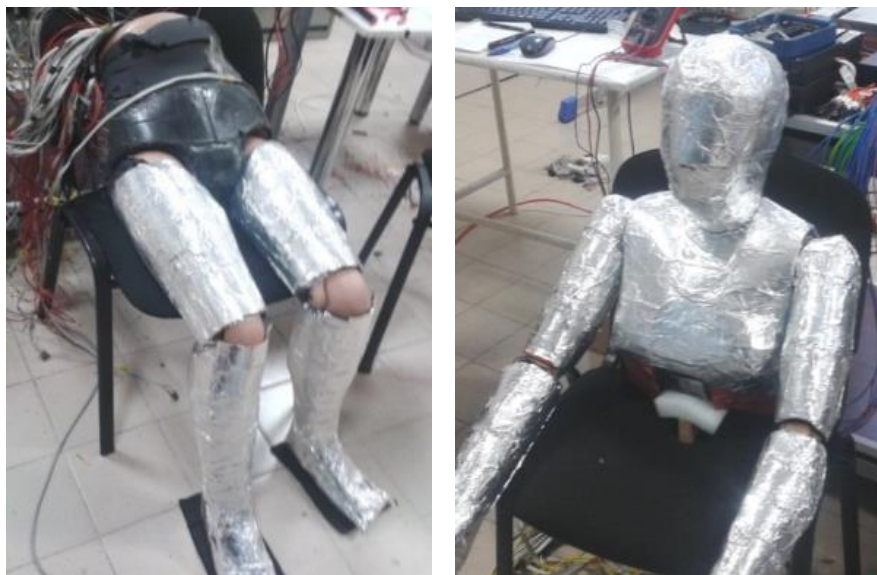
Figure 14:a) finished thermal manikin in lying position, b) testing the upper and the bottom body parts
