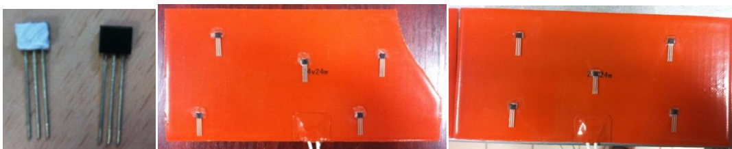
Figure 20: Photographs of Tsic T501 temperature sensors as disposed on the patches
