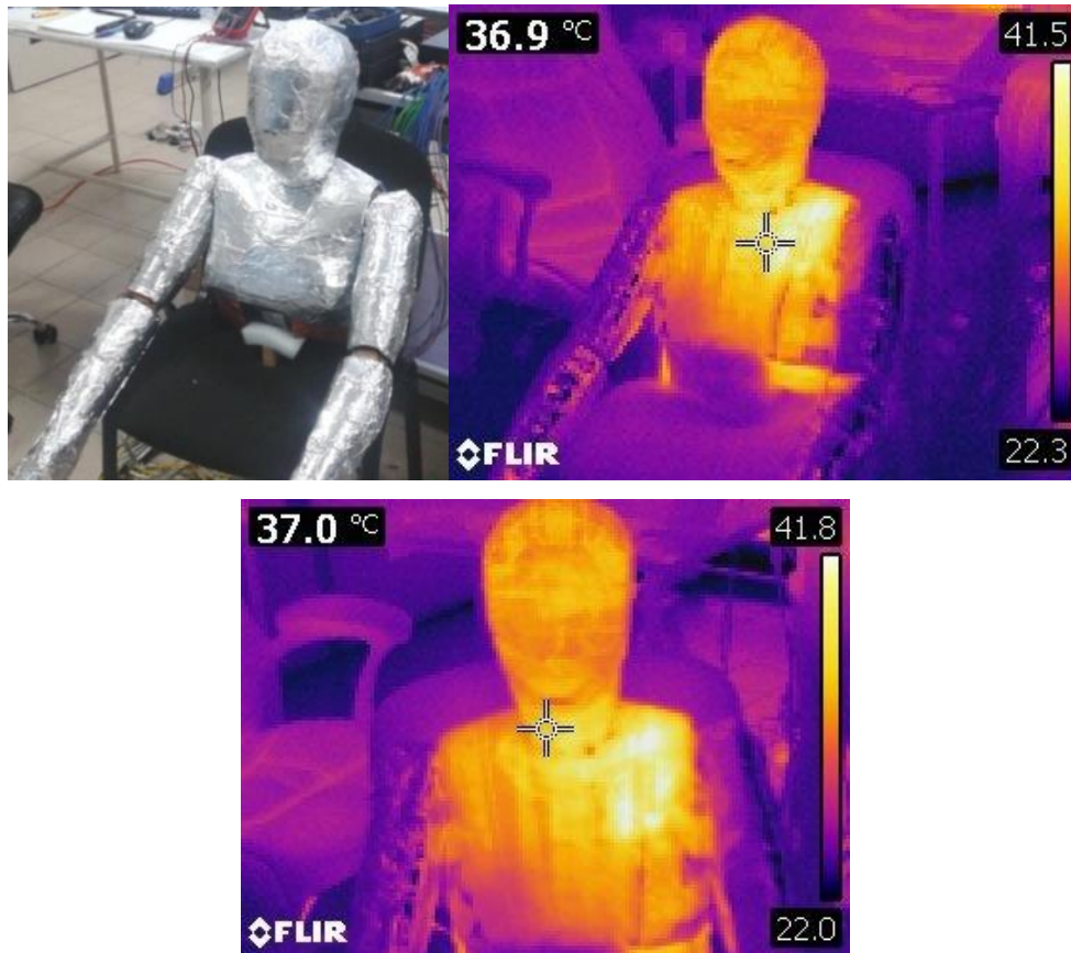
Figure 41: Experimental setup and temperature distribution for upper part of the manikin
