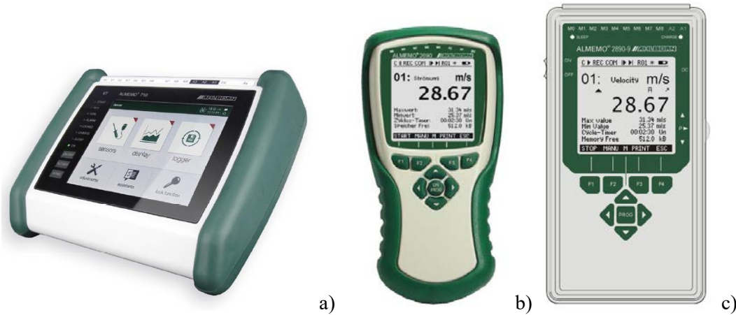
Figure 67: Almemo data loggers used in this study: a) Almemo 710; b) Almemo 2690-8; c) Almemo 2890-9
